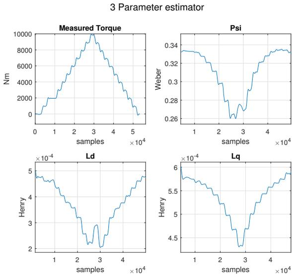
Fig. 8. 3PE experimental estimation
