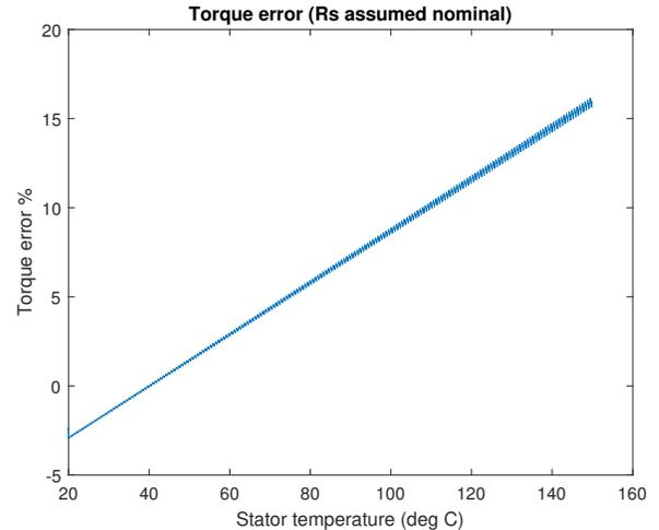
Fig. 5. Error on torque estimation (120RPM 8000Nm)
