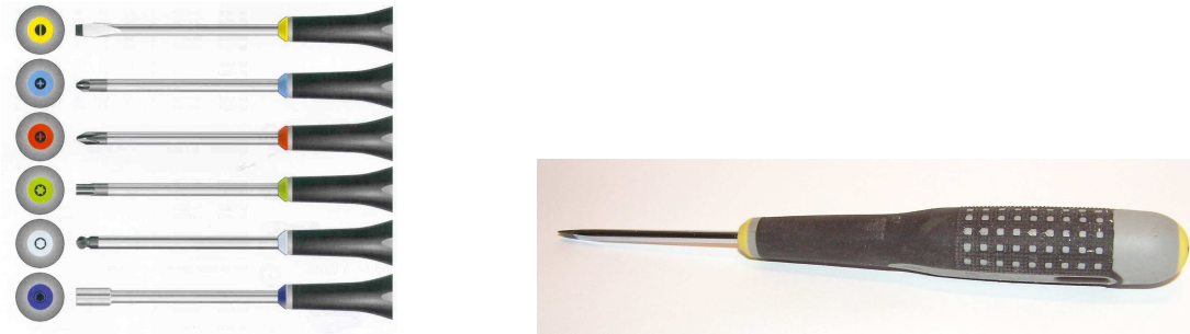
Figure 1a(left) and 1b(right). One of the set participatively and ergonomically designed screwdrivers (1a). In the area close to the metal it has a smaller diameter to enable precision tasks with a pinch grip (1b).
