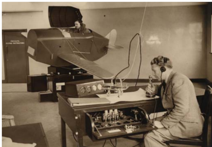
Figure 2.2: Link simulator in 1930 [14]
