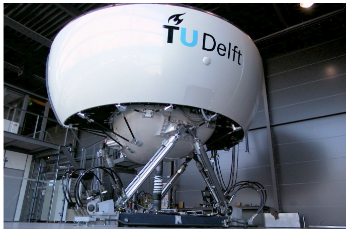
Figure 1-1: Flight simulator with Stewart platform [1]
