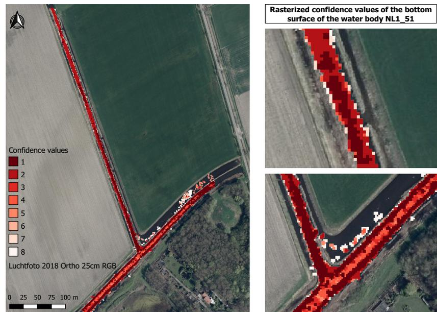
Figure 6.27: Water body (NL1\_151): Rasterized confidence values of bottom points with resolution 1m
