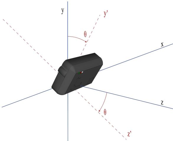
**Figure 2.1:** Roll angle during skating of the NGIMU sensor
