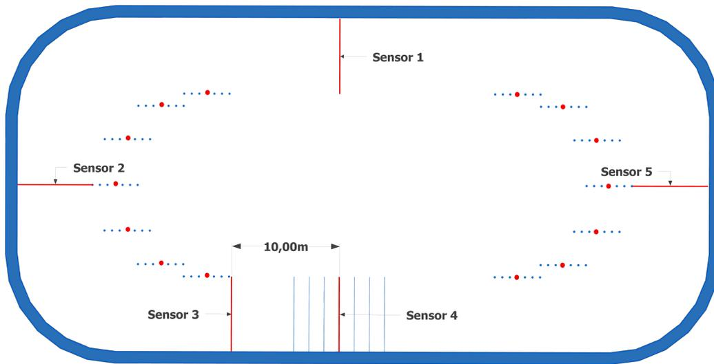
**Figure 2.2:** Mylapse sensors within the Thialf short track ice-rink
