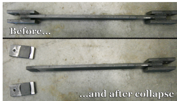
Figure 5.4: Failure mode of the beam
