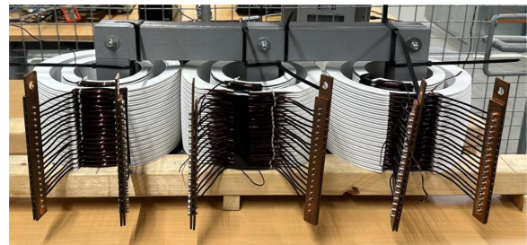
FIGURE 10. Assembled MFT with winding modules secured and core clamped in place.
