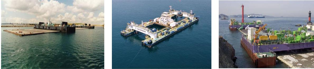
**Figure 5** different immersion pontoon types used in the projects (Oresund Fixed Link, Bosphorus Fixed Link and the Busan Goeje Fixed Link) [ (CAPITA SYMOND), (TAISEI Corporation , 2014), (Hans Cozijn and Jin Wook Heo, 2009) ]
