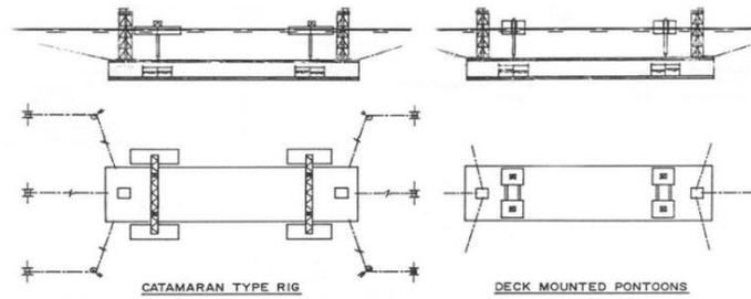
Figure 16 two type pontoons used often in construction of immersed tunnel (Gijsbert W. Nagel, 2011)
