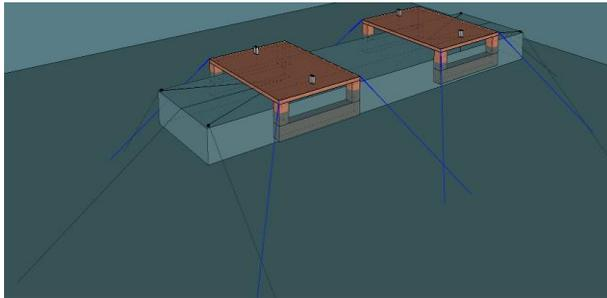
Figure 26 Semi-submersible pontoon during immersion
