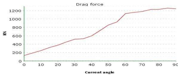
Figure 66 Drag force as a function of the current angle for a current velocity of 1[m/s]
