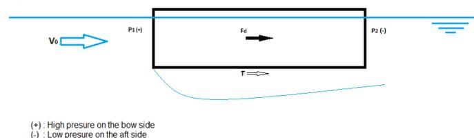
Figure 22 Principle of current force on TE during transport
