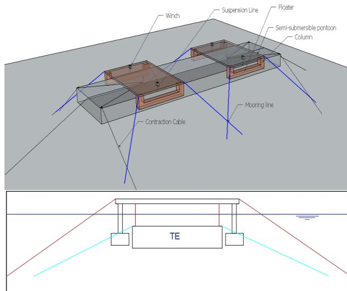
Figure 42 Semisubmersible pontoon
