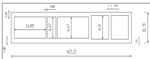
Figure 40 Simplified cross-section used in the calculations
