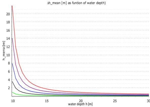
Figure 82 Mean values of the pressure drop as function of the water depth for five towing velocities (green = 0.5, black =1, blue=1.5, purple =2, red =2.5) in [m/s]
