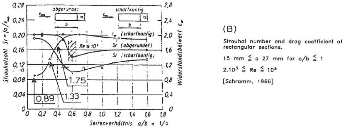
Figure 90 Strouhal -number Dependency on H/B (Schramm, 1966)
