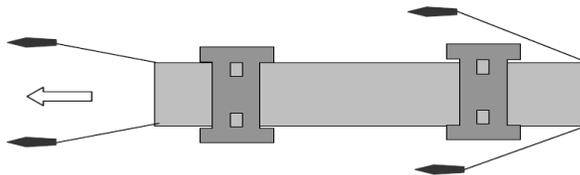
Figure 12 Tugboat configuration (FEHMARN BELT CONTRACTORS, 2013)
