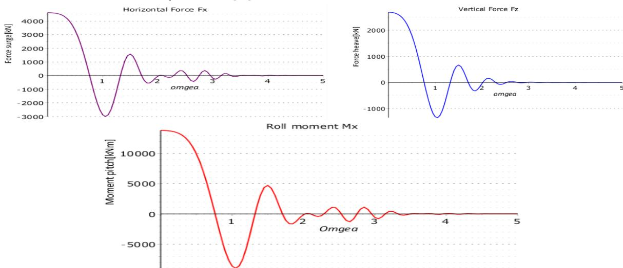
Figure 134 Froude-Krilov force on the Catamaran pontoon as function of the wave frequency
