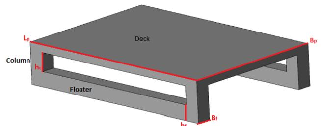
Figure 49 Altered pontoon layout
