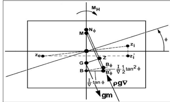
Figure 85 Principle of righting moment (J.M.J. Journée and W.W.Massie, "SHIP HYDRODYNAMICS", 2001)
