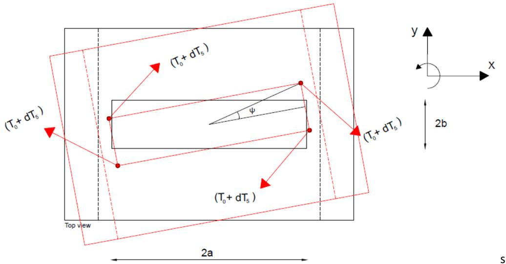
Figure 106 displacement in the yaw degree of freedom
