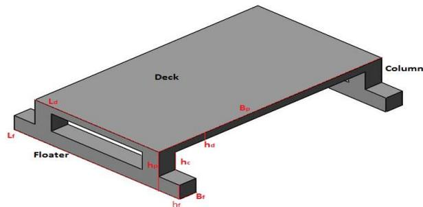
Figure 44 Semi-submersible pontoon
