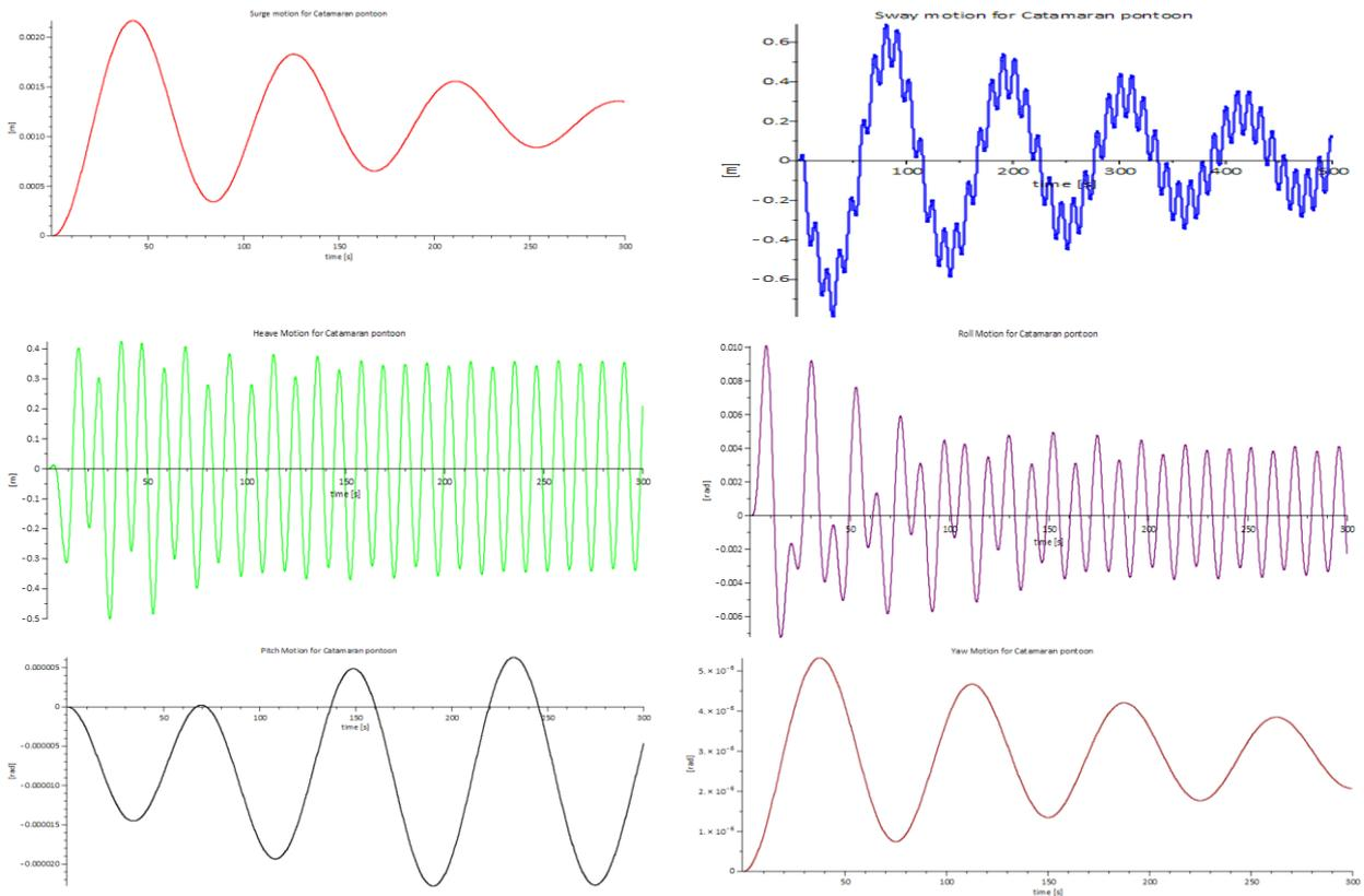
Figure 115 Motions of Catamaran Pontoon in 6 degrees of freedom for  $T_p=11$  [s] and  $H=1m$  (2 suspension cables)
