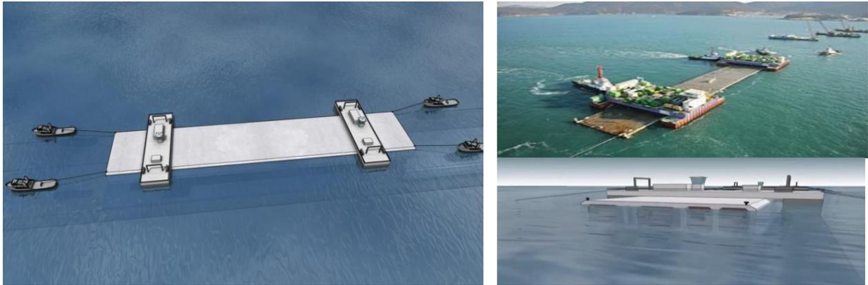
Figure 21 Tunnel element during transportation [(Femern A/S) and (Hans Cozijn and Jin Wook Heo, 2009)]
