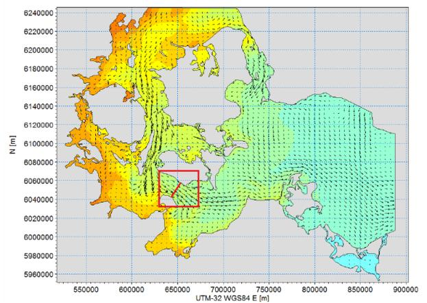
Figure 58 Ingoing flow from the North Sea (FEHY (Metocean Conditions), 2013)
