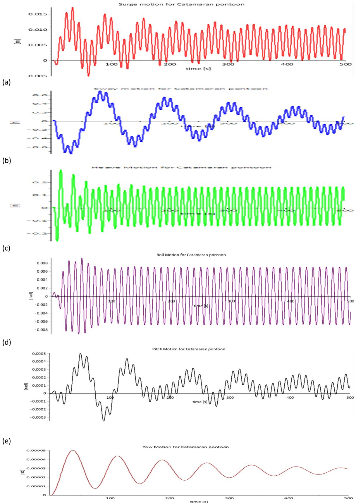
Figure 117 Motions of Catamaran Pontoon in 6 degrees of freedom for  $T_p=11$  [s] and  $H=1$ m (4 suspension cables)
