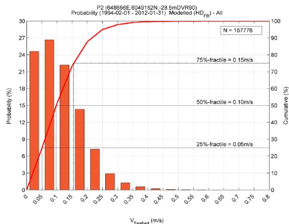
Figure 9 The distribution of near-bed current velocity (FEHY (Metocean Conditions), 2013)
