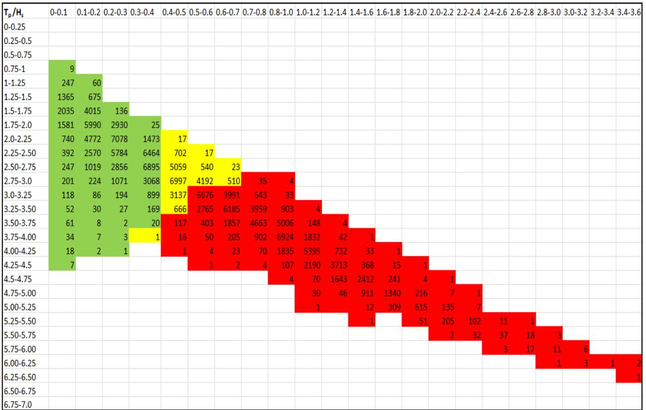
Figure 131 Workable conditions Semi-submersible pontoon (2suspension cables applied)
