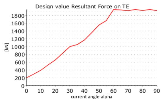
Figure 74 Design value Resultant force  $F_R$  for 1 m/s flow velocity
