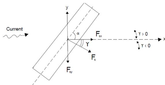
Figure 68 Transversal force in the y-direction
