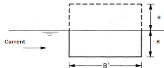
Figure 54 Principle of the drag coefficient derivation for a floating TE
