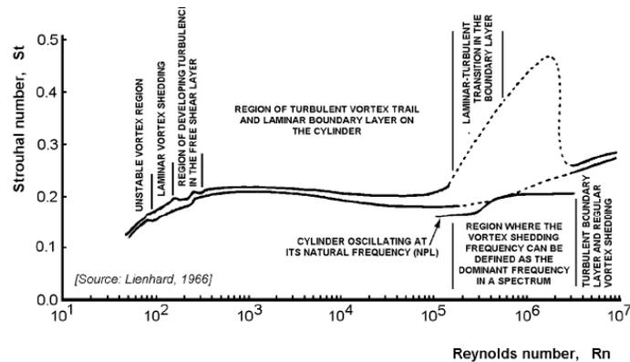
Figure 32 Strouhal number as function of Reynolds number for circular cylinder (J.M.J. Journée and W.W.Massie, First Edition, January 2001)
