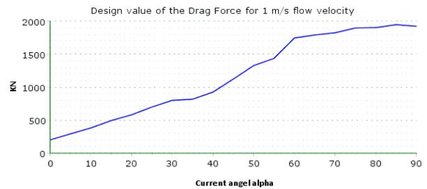
Figure 67 Design value of the drag force
