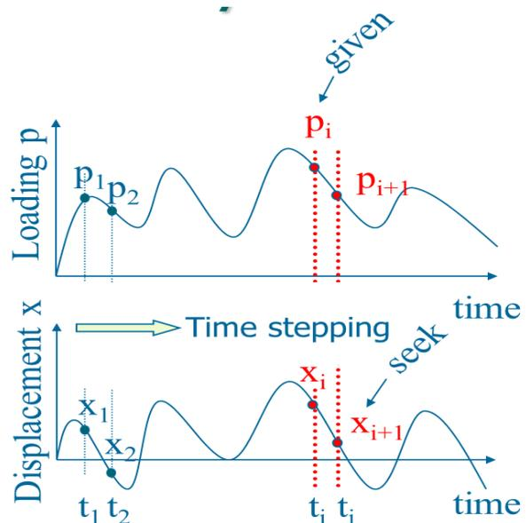
Figure 107 Principle of Newmark-beta method (Aurel Stratan, 2014)
