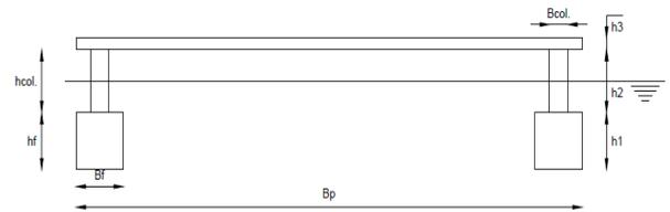
Figure 122 Semi-Submersible pontoon
