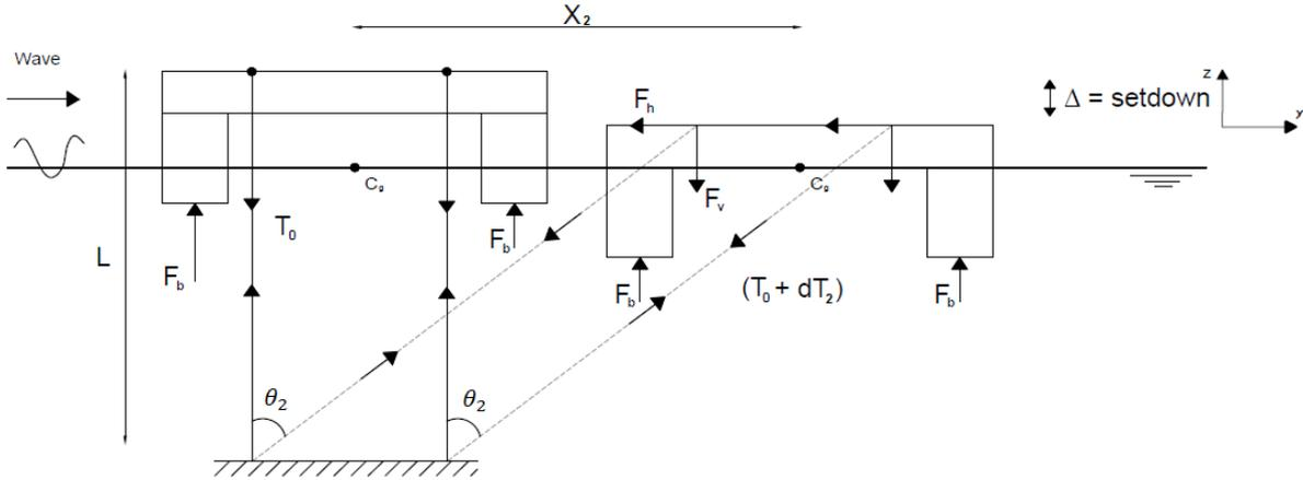
Figure 102 unit displacement in the sway direction.
