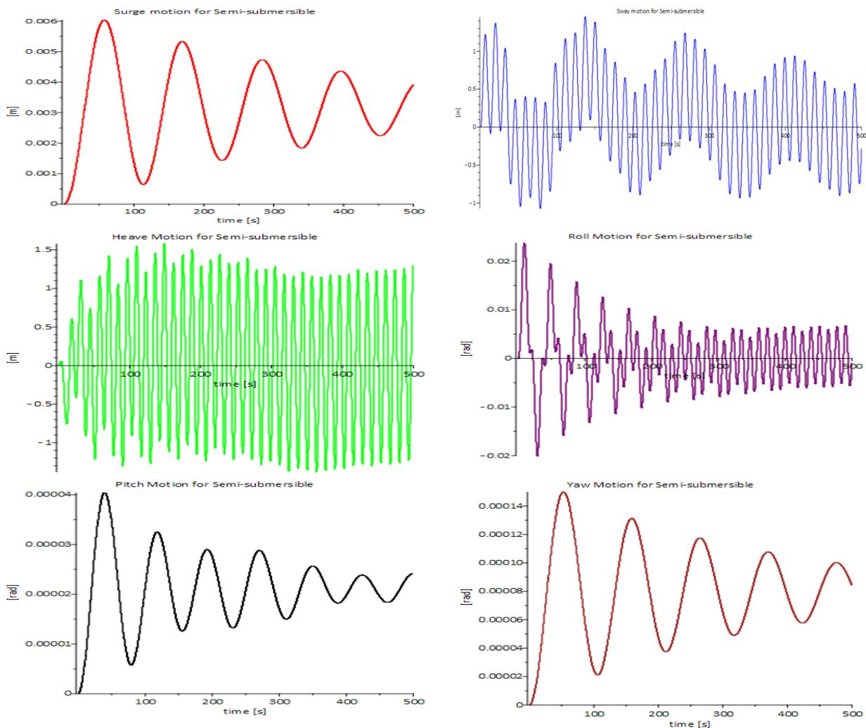
Figure 110 Motions of Semi-submersible in 6 degrees of freedom for  $T_p=13 [\text{s}]$  and  $H=2\text{m}$
