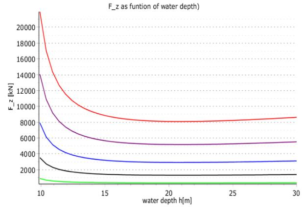
Figure 83 Vertical force as function of the water depth for five towing velocities (green = 0.5, black =1, blue=1.5, purple =2, red =2.5) in [m/s]
