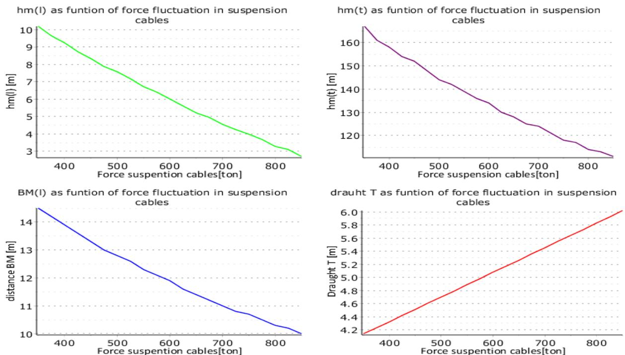
Figure 47 Effect of the fluctuation of the force in suspension cables on static stability
