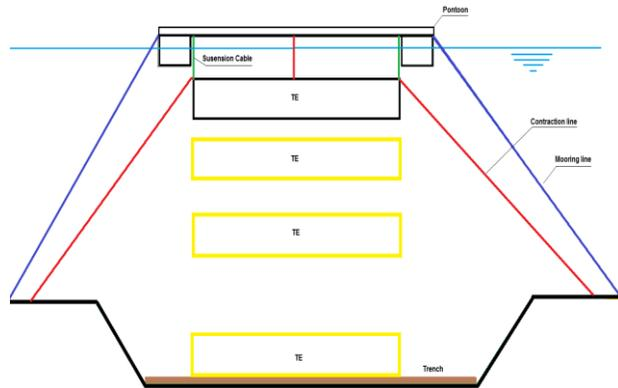
Figure 28 TE during immersion
