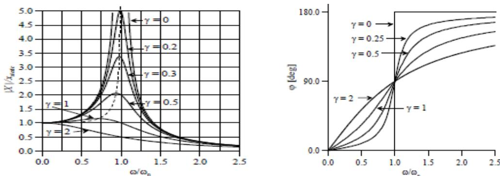
Figure 34 Amplification factor and phase lag (Spijkers, J.M.J., A.C.W.M. Vrouwenvelder, and E.C. Klaver., 2006)
