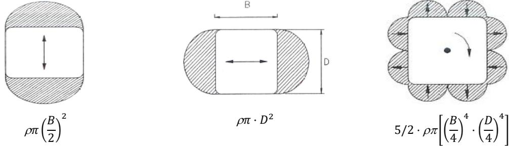
Figure 124 Estimate of added mass for fully submerged parts (Baltrop, 1998). Copied from (Floating Structures, 1998)
