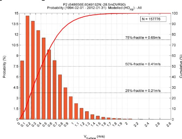
Figure 8 The distribution of surface current velocity (FEHY (Metocean Conditions), 2013)
