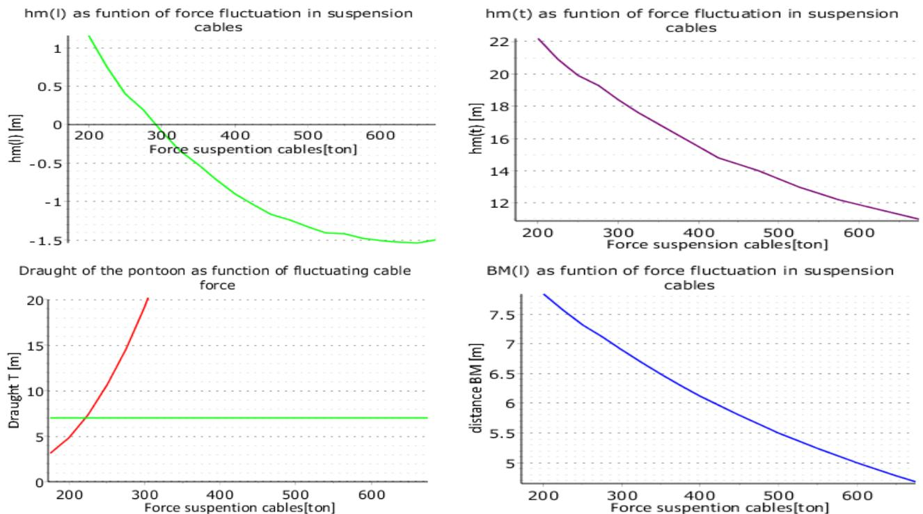
Figure 48 Effect of fluctuating cable force on static stability (Semisubmersible type pontoon)
