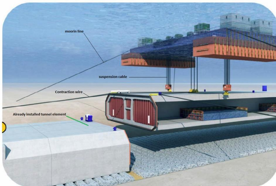
Figure 18 Tunnel element hanging on pontoon during the immersion (CAPITA SYMONDS)
