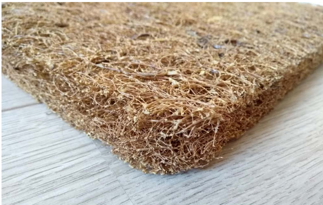
Figure 5.17: a sample of coconut husk 'foam'
