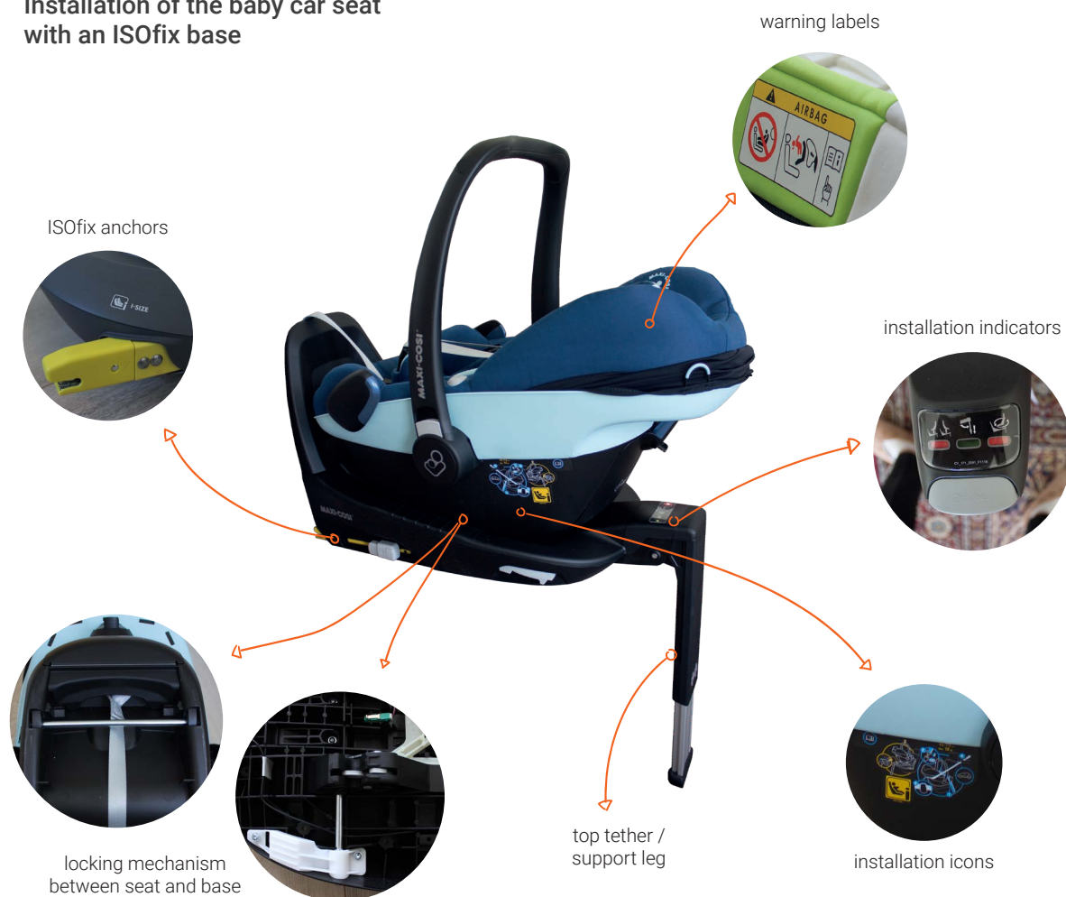
Figure 3.2: parts of a baby car seat and an ISOfix base facilitating correct installation of the seat inside the car with an ISOfix base
