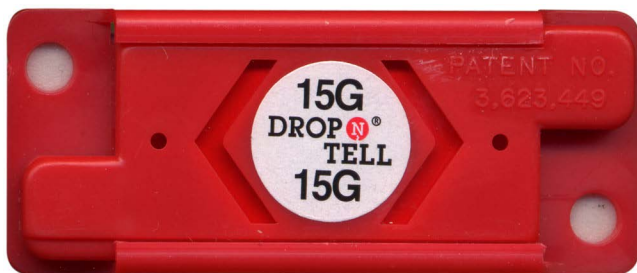
Figure 3.7: Drop N Tell impact indicator (courtesy of International Plastics, n.d.)
