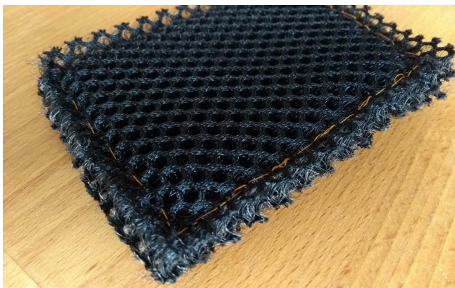
Figure 5.14: two layers of spacer mesh sewn together
