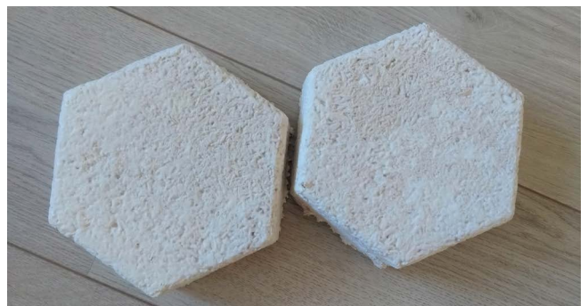
Figure 5.16: samples of rigid mycelium foam
