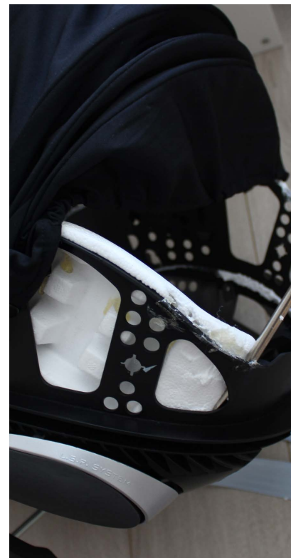
Figure 3.32: removing foam from the Cloud Z
