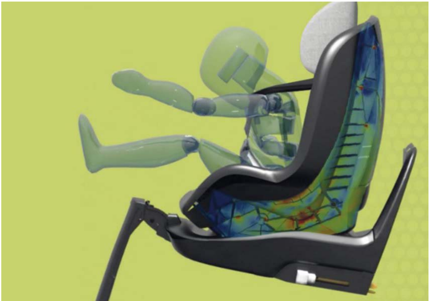
Figure 2.7: a crash simulation of a forward facing toddler seat and an ISOfix base (courtesy of Code Product Solutions, n.d.)
