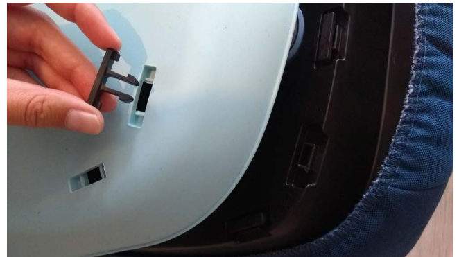
Figure 13: snapfit to fasten rubber cover to Pebble Pro
