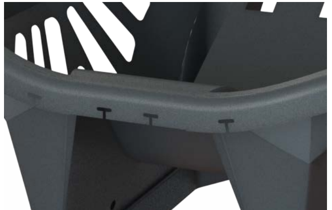
Figure 5.30: holes in the shell of the redesigned baby car seat to fasten the upholstery
