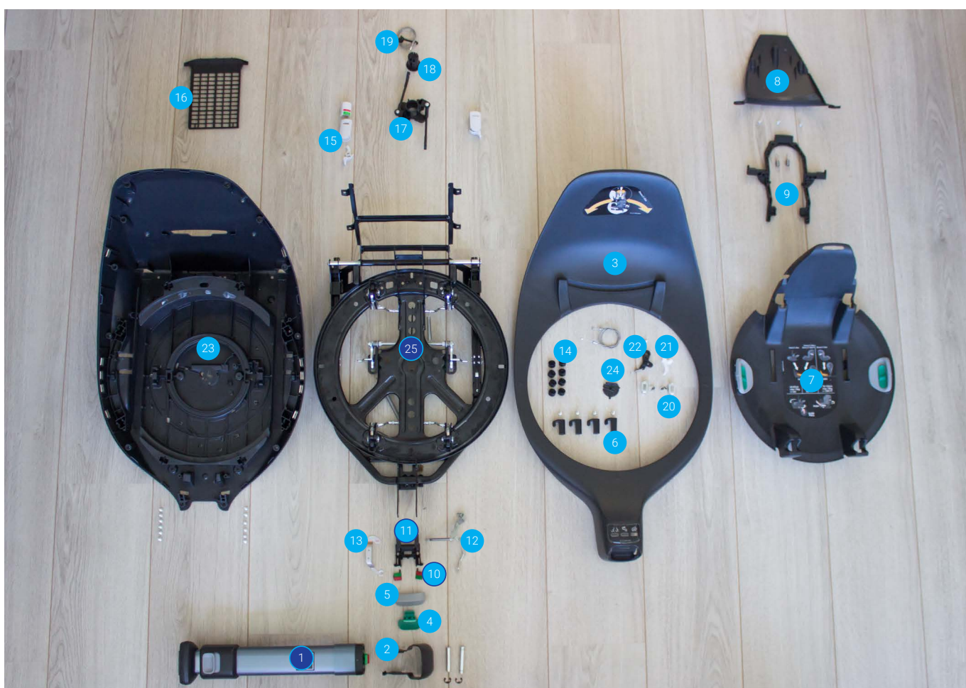
Figure 3.28: the componts of the Cybex Z base
