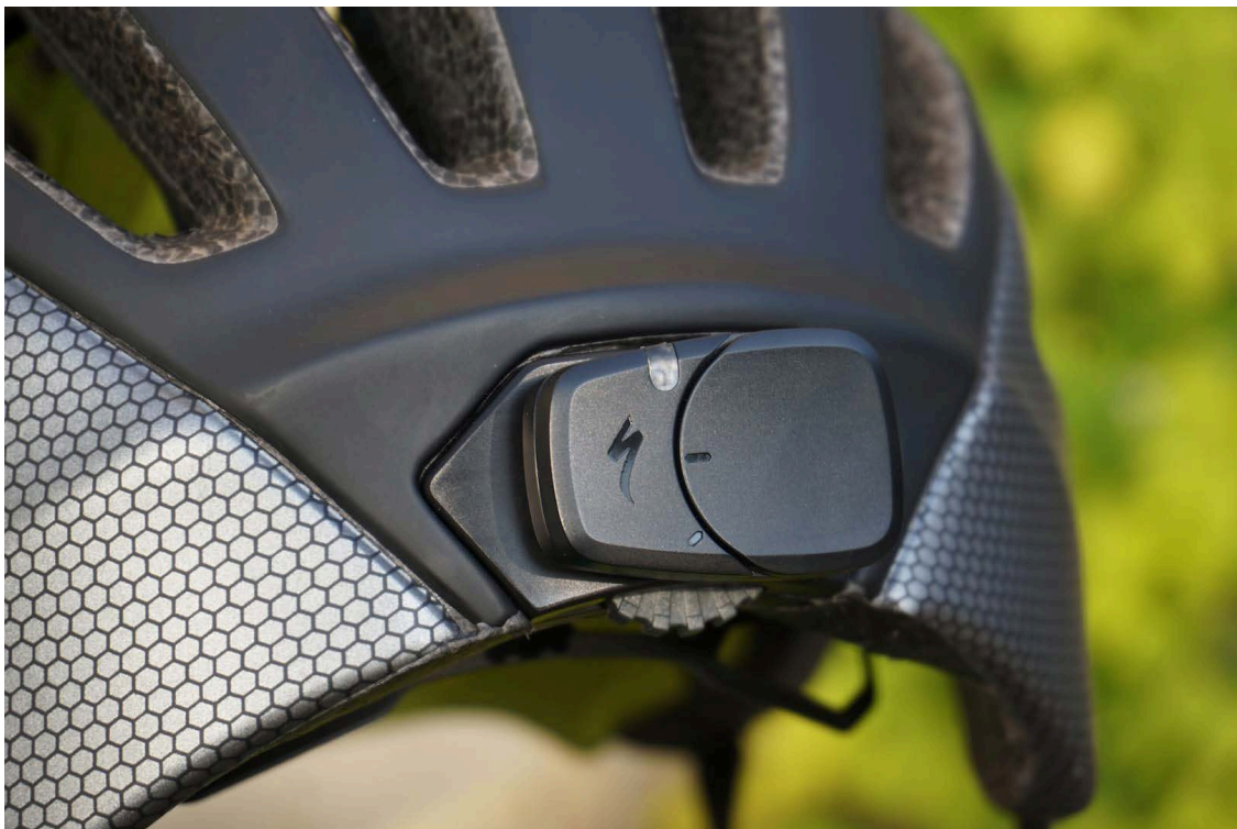
Figure 3.10: Specialized ANGI impact sensor for cyclists (courtesy of Specialized via Bikeshop.nl, n.d.)
