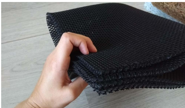
Figure 5.13: several layers of spacer mesh
