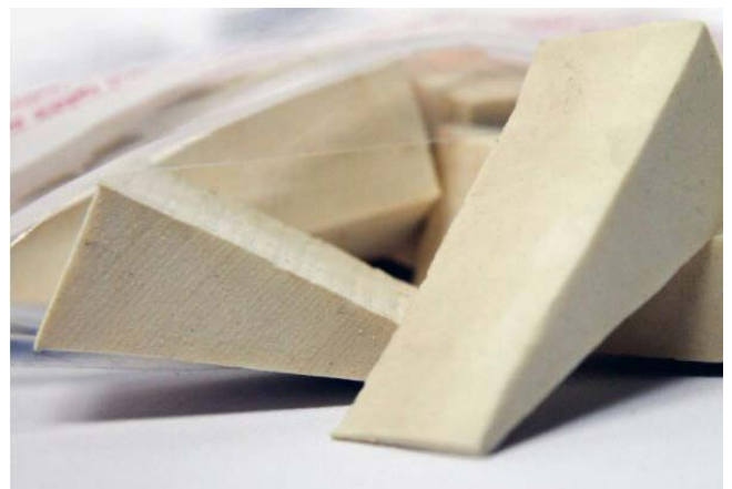
Figure 5.15: mycelium make-up sponges (courtesy of Ecovative, n.d.)
