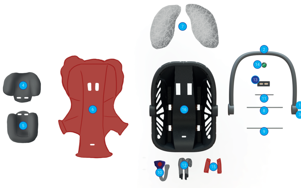
Figure 5.47: the components of the redesigned baby car seat
