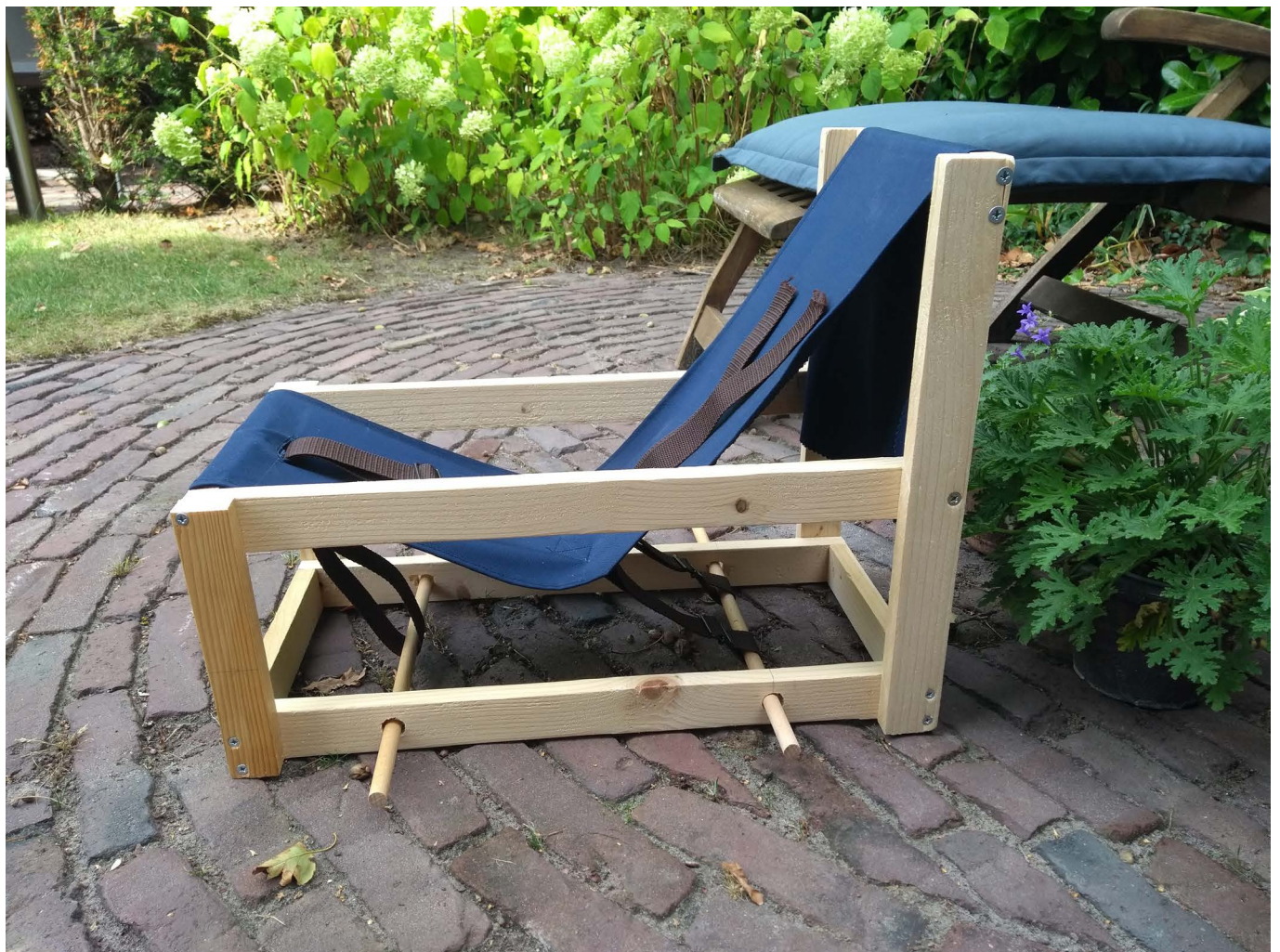
Figure 5.24: a prototype to test the application of self-supporting upholstery put under tension by fastening to an axis
