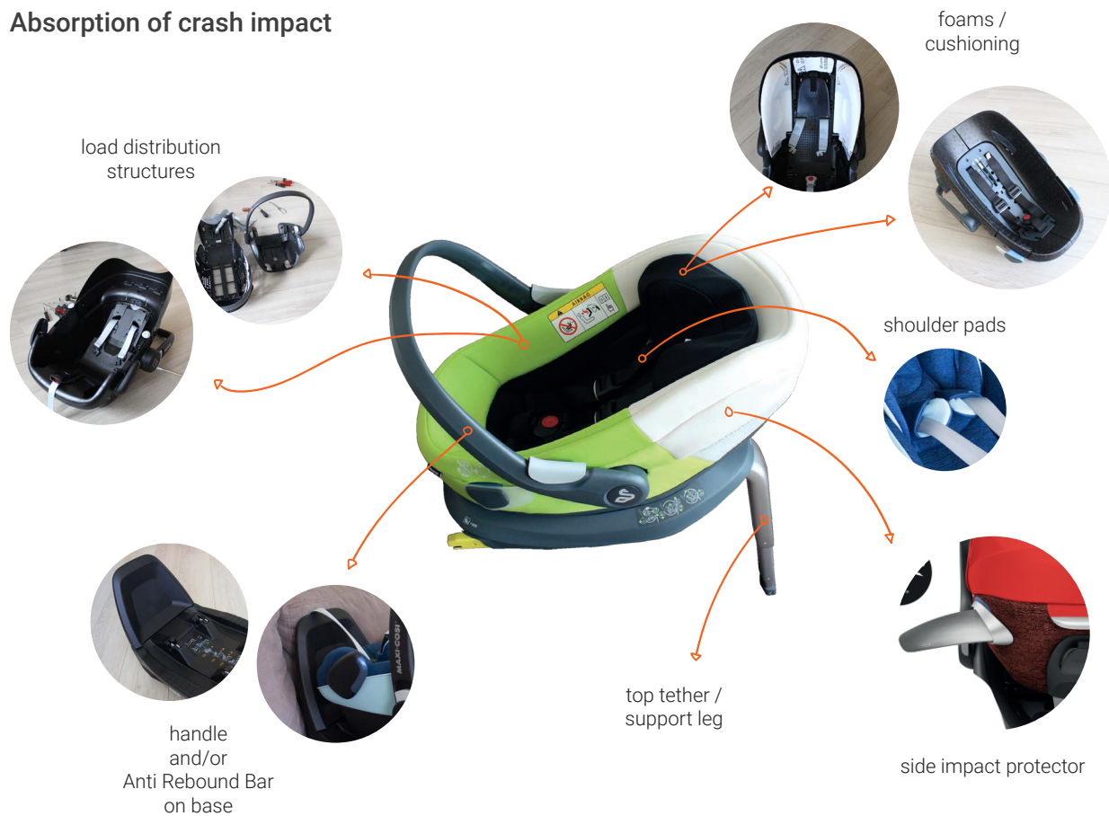
Figure 3.5: parts of a baby car seat and an ISOfix base facilitating absorption of crash impact (picture of side impact protector courtesy of Cybex, n.d.)
