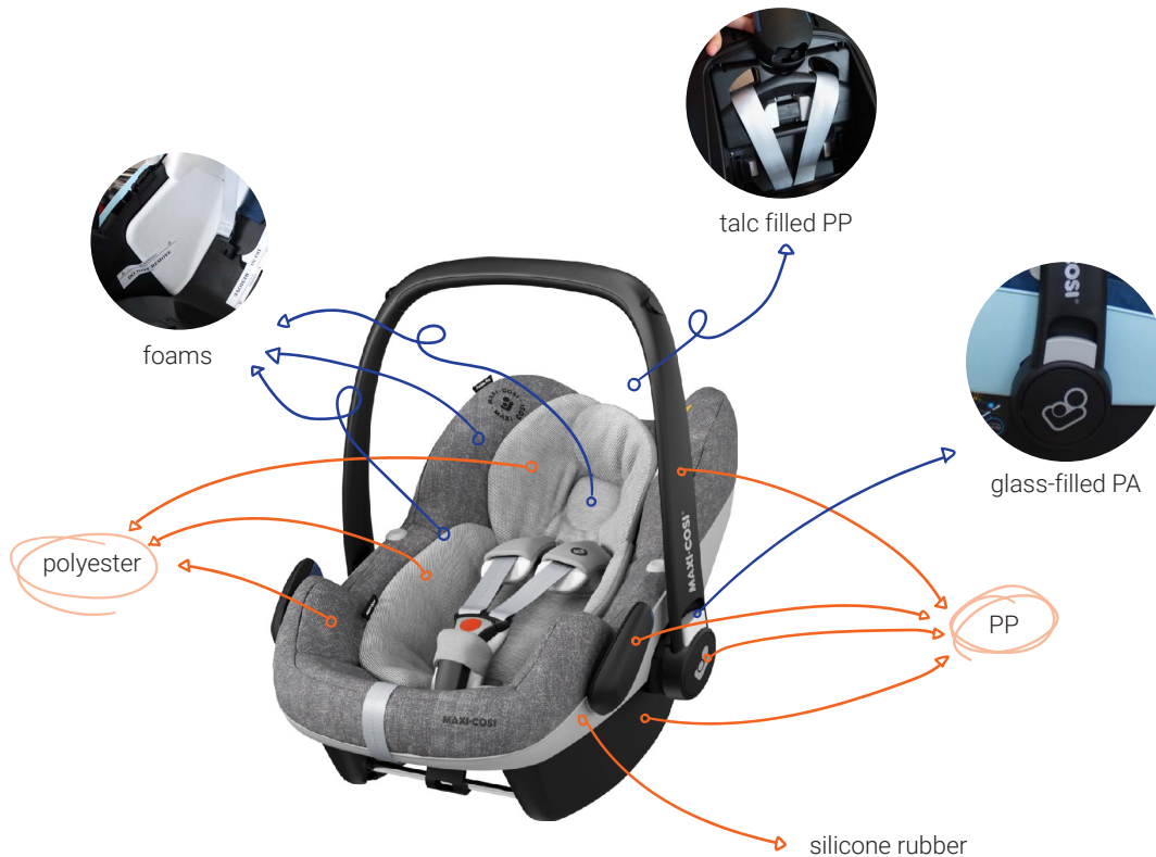
Figure 4.11: the different types of polymer-based materials of the Maxi-Cosi Pebble Pro
