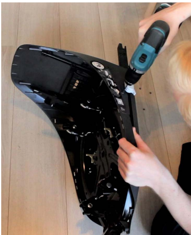
Figure 3.33: drilling out rivets of the Cybex Z base
