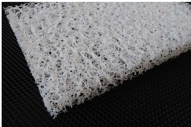
Figure 5.12: 3D polymer network
