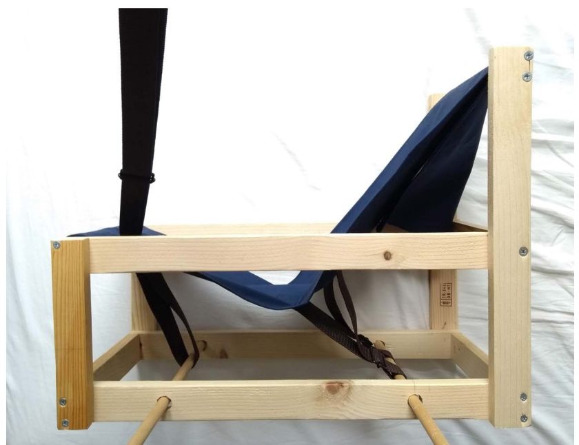
Figure 5.40: a prototype to test the fixation of the buckle with an axis at the bottom of the baby car seat
