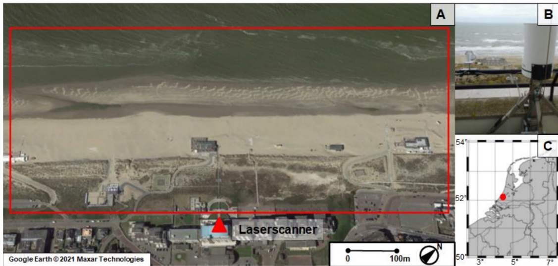
Figure 3.1: (A) An aerial image showing the location of the laser scanner (red triangle), and the research area covered by the laser scanner in Noordwijk. (B) The laser scanner, positioned on the rooftop of a hotel overlooking the beach. (C) The geographic position of Noordwijk ( 52.24^\circ N, 4.42^\circ E). Retrieved from Vos et al. (2023).
