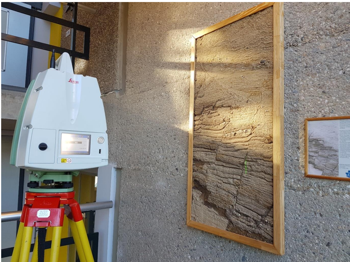
Figure 3.4.1. Practicing with the Leica C10 laser scanner.
