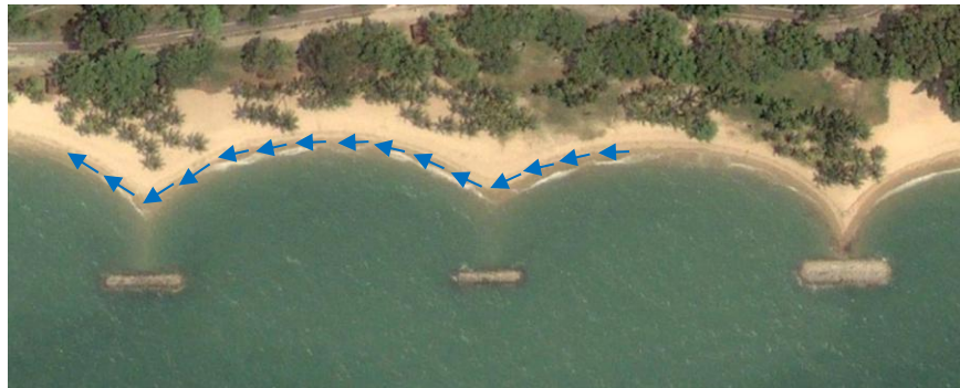
Figure 6.25 Pocket beaches enclosed by headlands 8, 9 and 10, prior to 2009 when the tombolos were raised through nourishment works. The blue arrows indicate the possible movement of sediment in the lee of the headlands during high water.
