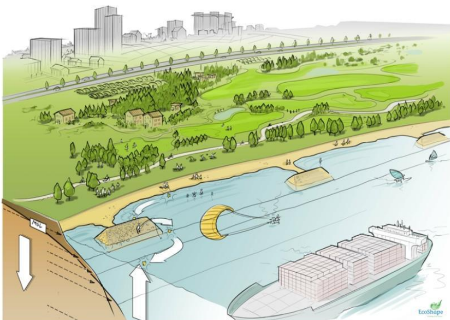
Figure 4.9 An illustration of processes contributing to a structural loss of sediment. Sediment by-passing around structures is shown in the top view of the sketch, and sea level rise and land subsidence in the cross-shore transect. Created by JAM visual thinking ( http://www.jam-site.nl/ )
