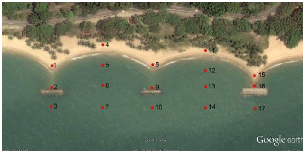
Figure C.1 Suggestive cross-shore locations of sediment samples to be collected within the beach cells enclosed by headlands 8, 9 and 10
