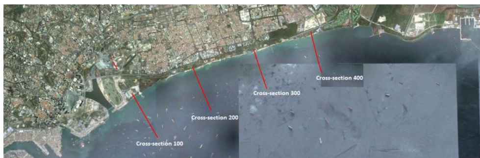
Figure 5.16 Cross-shore rays along the southeast coast, with no. 200, 300 and 400 along East Coast Park.
