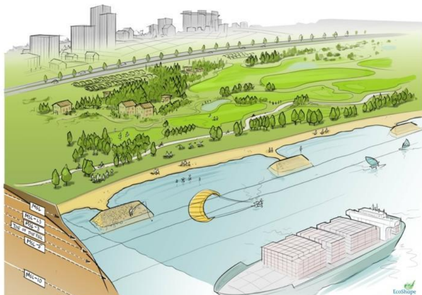
Figure 4.7 Illustrative sketch of a part of East Coast Park and a cross section, indicating different sediment layers and contour depths. Created by JAM visual thinking ( http://www.jam-site.nl/ )
