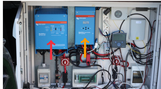
(b) Picture of the actual DC connected ESS experimental setup with all of the devices.
