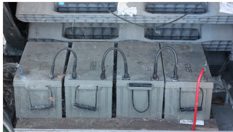
(c) Picture of the lead acid BESS connected to the DC experimental setup.
