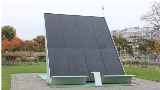
(a) PV panels used for the DC connected ESS experimental setup.
