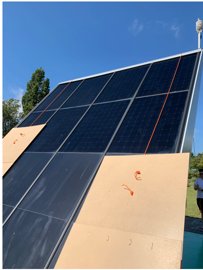
Figure 5.2: Illustration of how the shade experiments were conducted. The planks were moved up and down along the PV panels by pulling on a rope that is attached to the planks and runs all the way behind the PV system.
