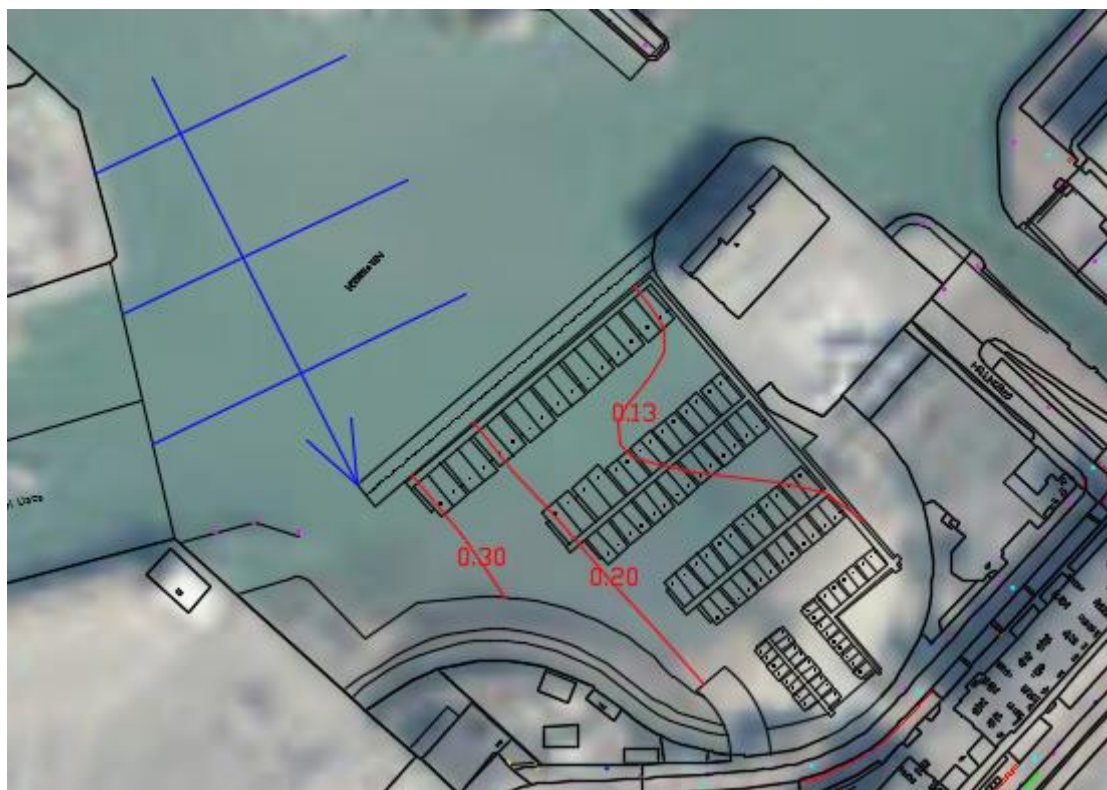
Figure 67. Wave attenuation – Wiegel (1964) diagram for a wave with angle of 15^\circ with perpendicular to breakwater. The red lines represent the wave attenuation coefficients, while the blue lines are the incoming wave crests and ray.
