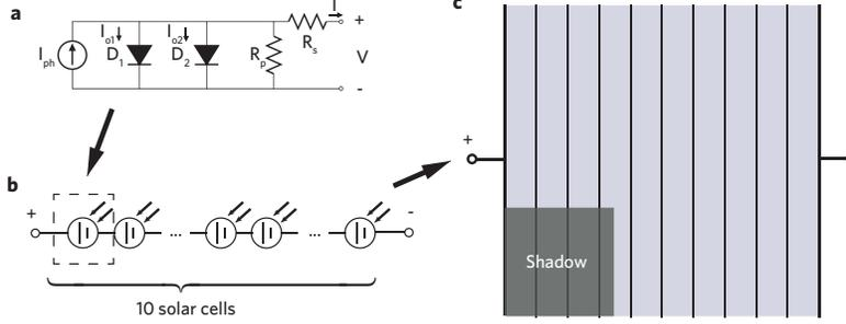
Figure 5: **Model of solar cell and PV module in shadows**
