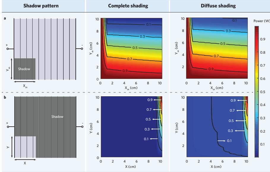
Figure 14: Simulation results of PV partial shading effects.
