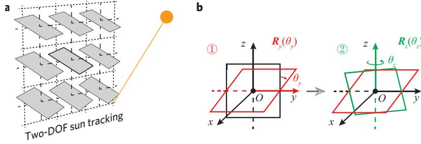
Figure 3: **Two-DOF sun tracking and definition of rotation angles**
