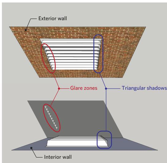
Figure 8: **Shadow simulation of the optimum position of one-DOF shading elements by SketchUp [51]. Interior glare zones (red) and triangular shadows (blue) on the slats are marked.**
