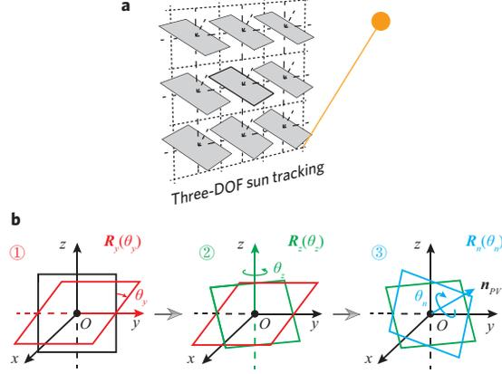
Figure 4: **Three-DOF sun tracking and definition of rotation angles**
