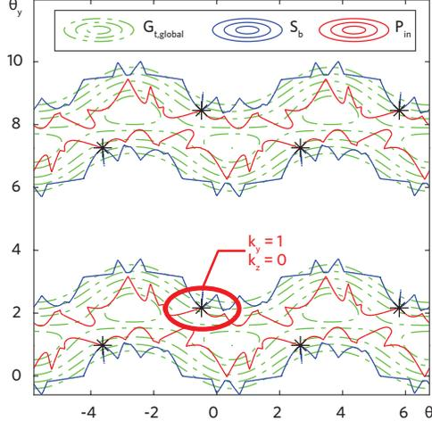
Figure 12: A periodic contour map of  $G_{t,global}$  (green),  $S_b$  (blue), and  $P_{in}$  (red) on the squares as a function of  $\theta_y$ ,  $\theta_z$ , and  $\theta_n$ , where the value of  $\theta_n$  is obtained by Eq. 32. The solution points are marked with stars, among which the one in the red circle is nearest to the initial position.
