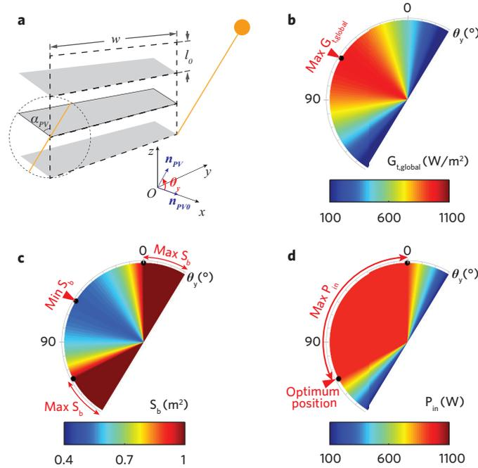
Figure 7: **Simulation results of all possible one-DOF sun tracking positions**
