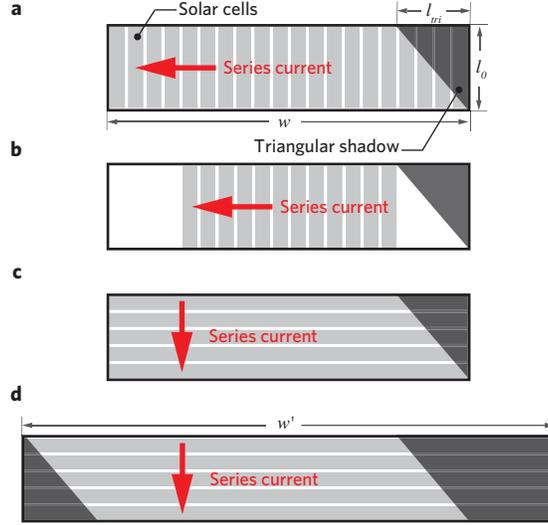
Figure 18: **Optimization of cell layouts for one-DOF sun tracking.**
