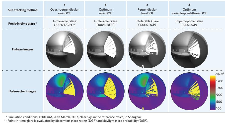
Figure 17: Simulation results of point-in-time glare by four sun-tracking methods.
