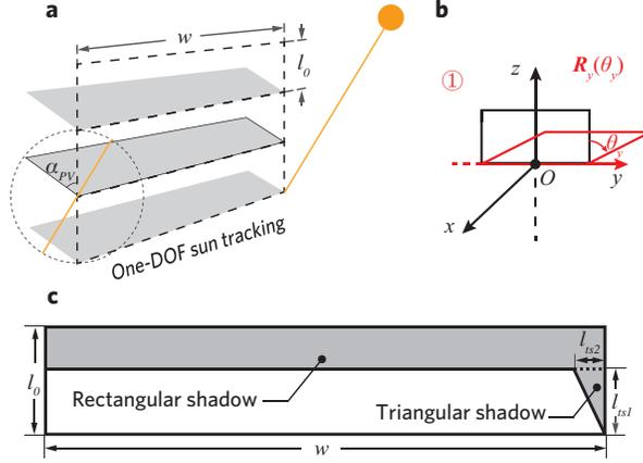
Figure 2: One-DOF sun tracking with a horizontal axis.
