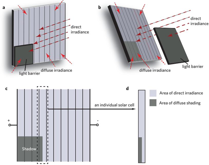
Figure 6: **Partial shading on the PV module**
