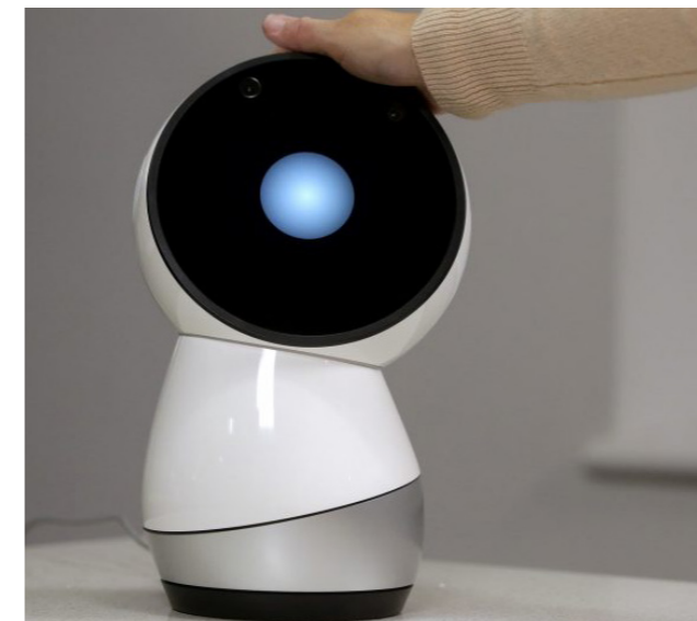
Figure 3.4: Jibo is a friendly robo-assistant. Equipped with cameras and microphones, it can recognize faces, understand what people say, and respond.
