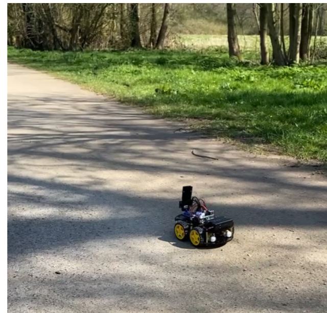
Figure 5.4: ELEGOO smart car is navigating on the streets without having an operator. In this case, the robot uses ultrasonic sensors that measure the distance from the surrounding objects.
