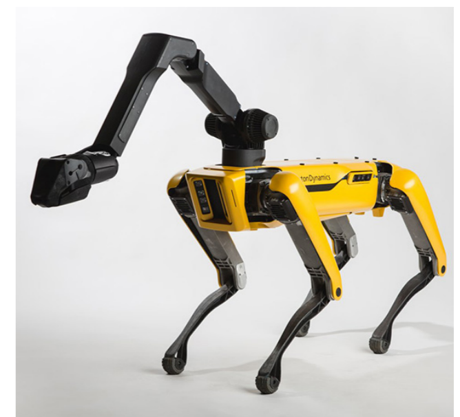
Figure 3.7: Spot is an agile mobile robot that navigates terrain with unprecedented mobility, allowing to automate routine inspection tasks and data capture safely, accurately, and frequently developed by Boston Dynamics.
