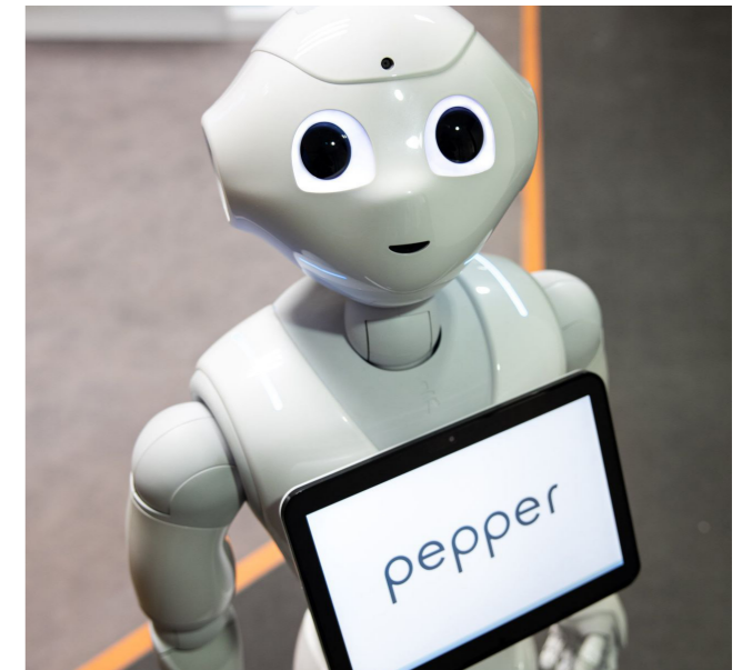
Figure 3.3: Pepper is a semi-humanoid robot manufactured by SoftBank Robotics, designed with the ability to read emotions.
