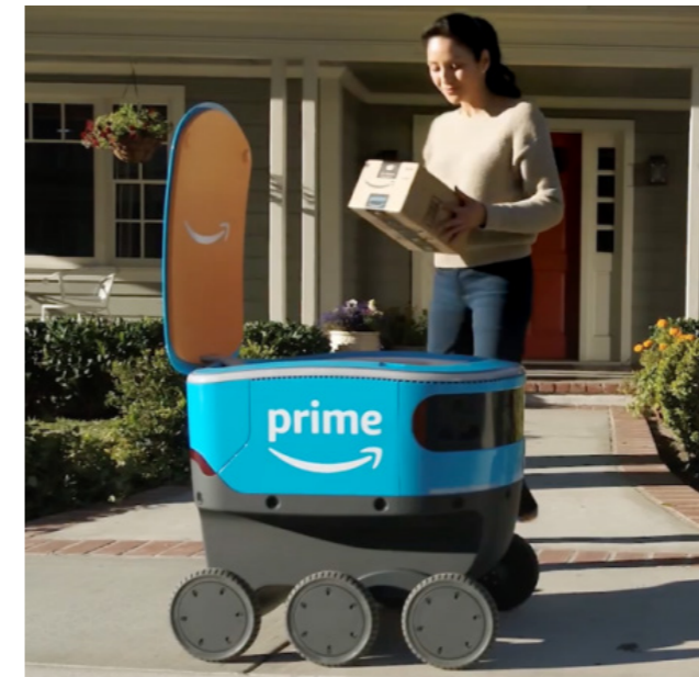
Figure 3.2: Amazon Scout is a 6 wheeled robot used to deliver packages for the E-commerce site, Amazon.com. Amazon Scout originally debuted on January 23, 2019, delivering packages to Amazon customers in Snohomish County, Washington. Amazon scouts move on sidewalks, at a walking pace.
