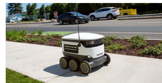
Figure 3.6: Starship delivery robot. These robots can cross streets, climb curbs, travel at night and operate in both rain and snow, are monitored remotely by Starship. Human operators can take control of the robots if needed.
