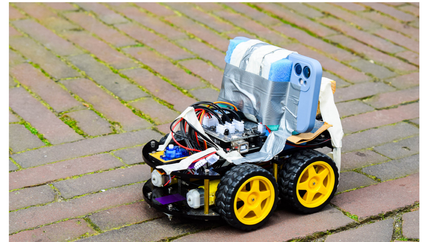
Figure 5.21: A picture of the system that used for recording first perspective videos. A smartphone was temporarily attached to the ELEGOO SMART CAR for recording its perspective.
