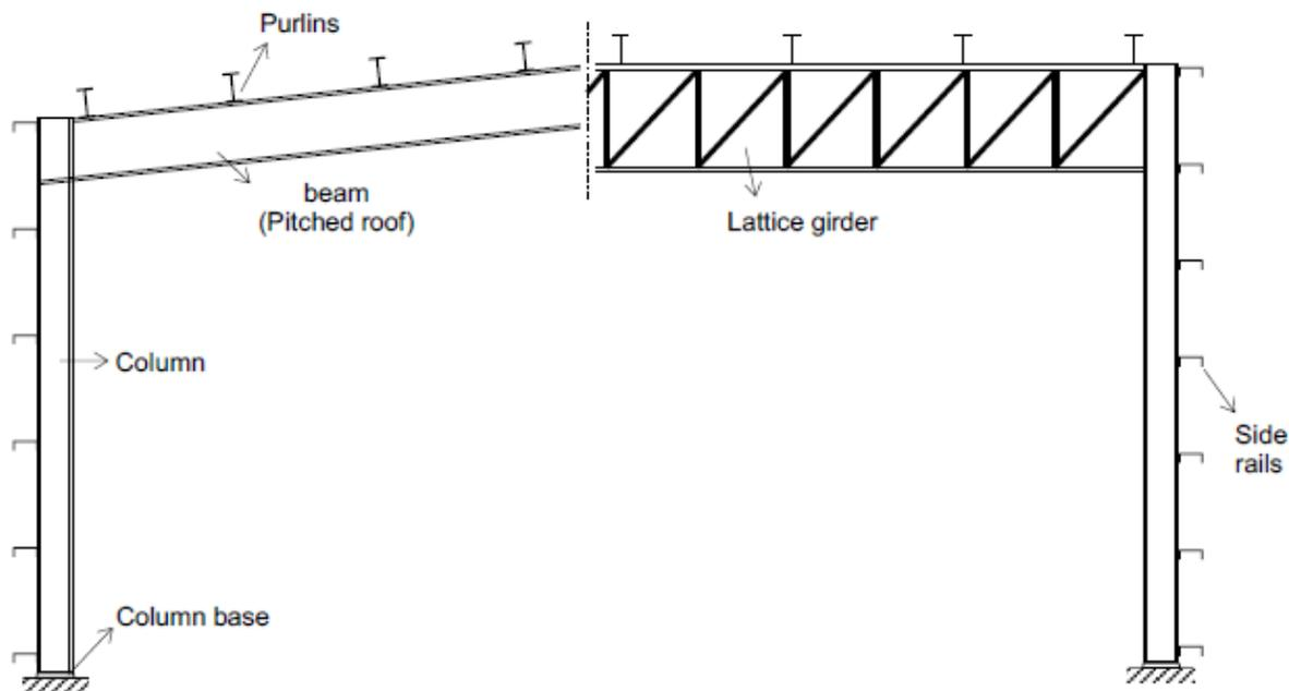
Figure 2.18: Typical structural elements in single storey industrial halls [24]
