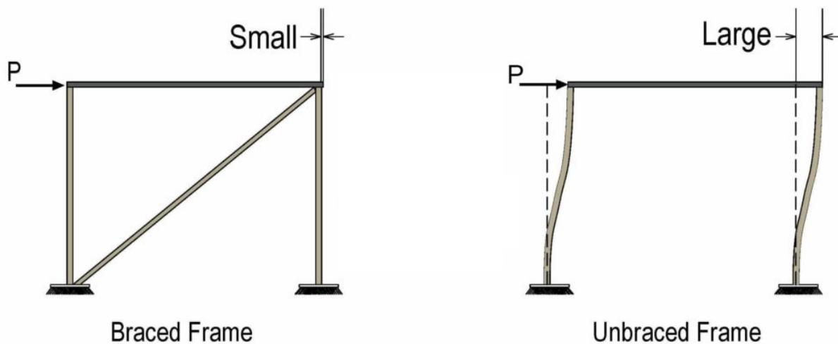
Figure 2.21: Braced and unbraced stability systems [Adapted from 25]
