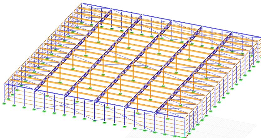
Figure 5.16: Multi objective optimized design for Newlogic III in RFEM
