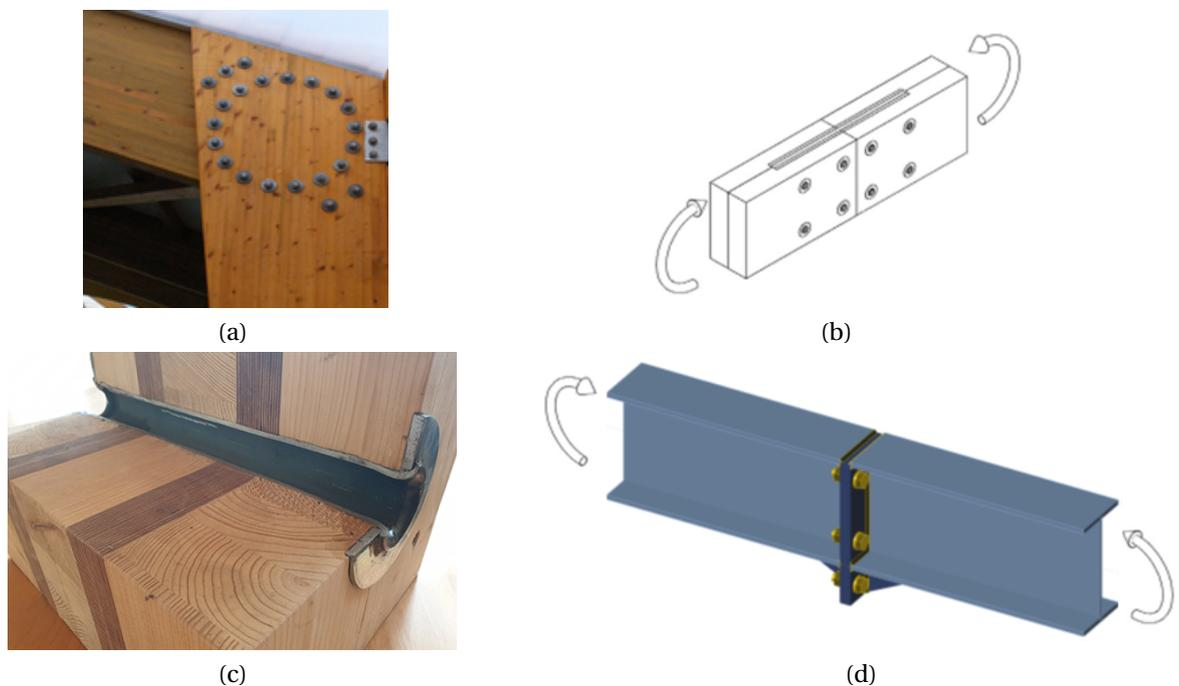
Figure 4.4: Examples of demountable connection types in steel and timber [97], [96], [98]
