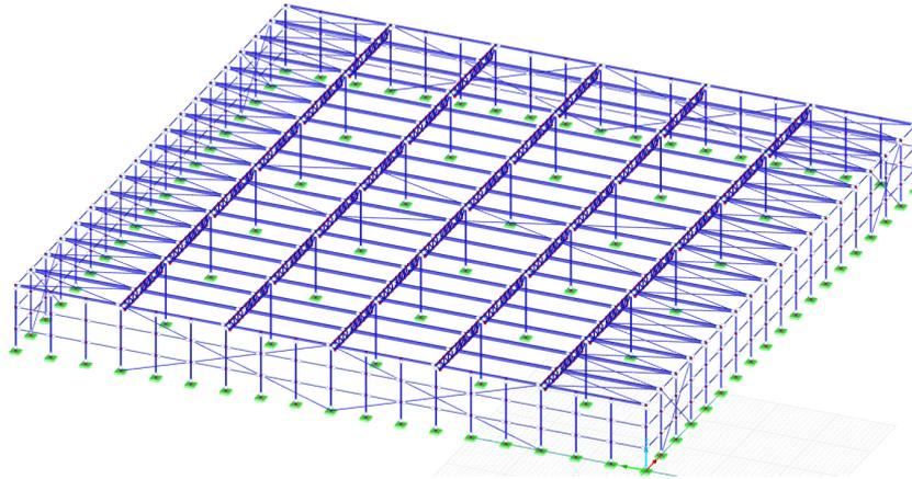
Figure 5.15: ECI optimized design for Newlogic in RFEM
