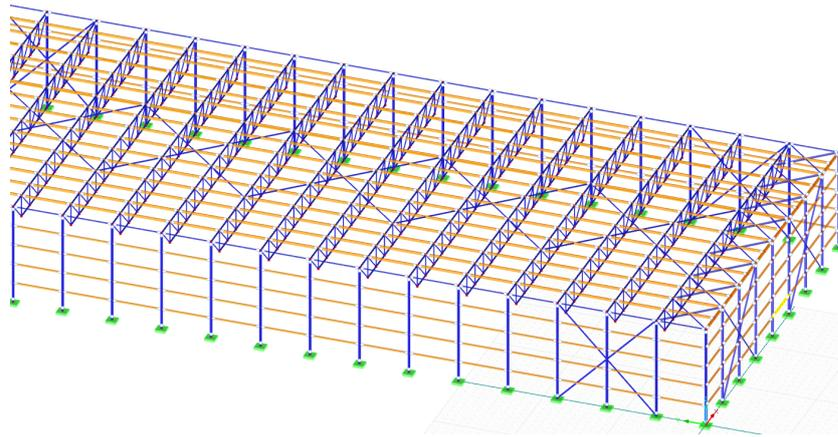
Figure 5.13: Multi objective optimized design for Coca Cola 27 in RFEM
