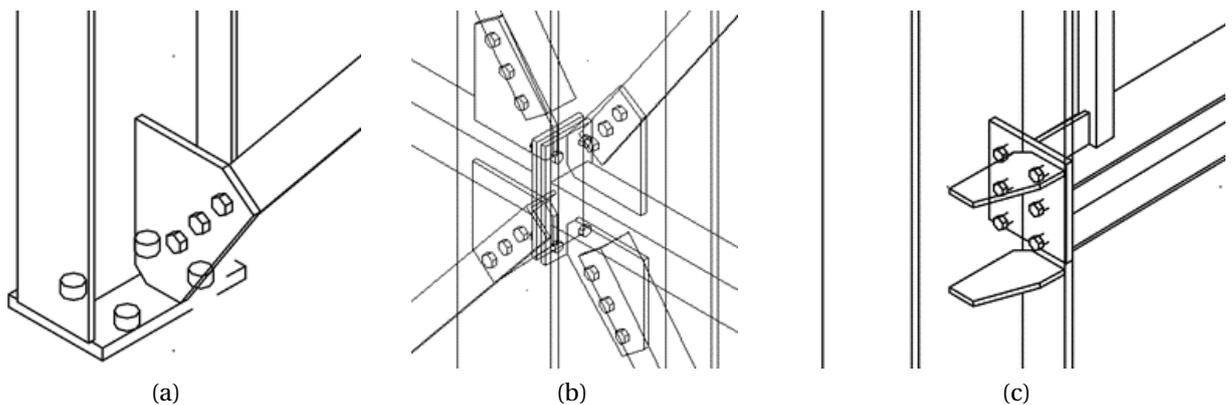
Figure 2.7: (a) Columnbase-windbrace connection, (b) Windbrace intersection connection, (c) Truss-column connection [20]
