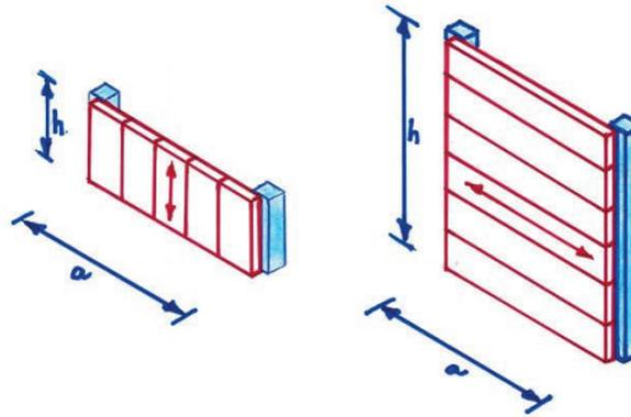
Figure 2.19: Span directions of facade elements [Adapted from 23]
