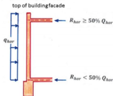
Figure 2.20: Transfer of horizontal loads on the facade to the roof and foundation [Adapted from 23]
