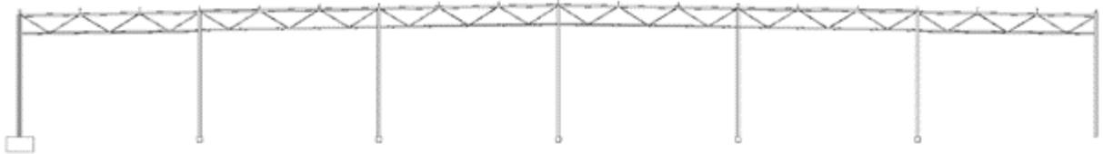
Figure 2.12: Portal frame of distribution center Newlogic III Tilburg [21]
