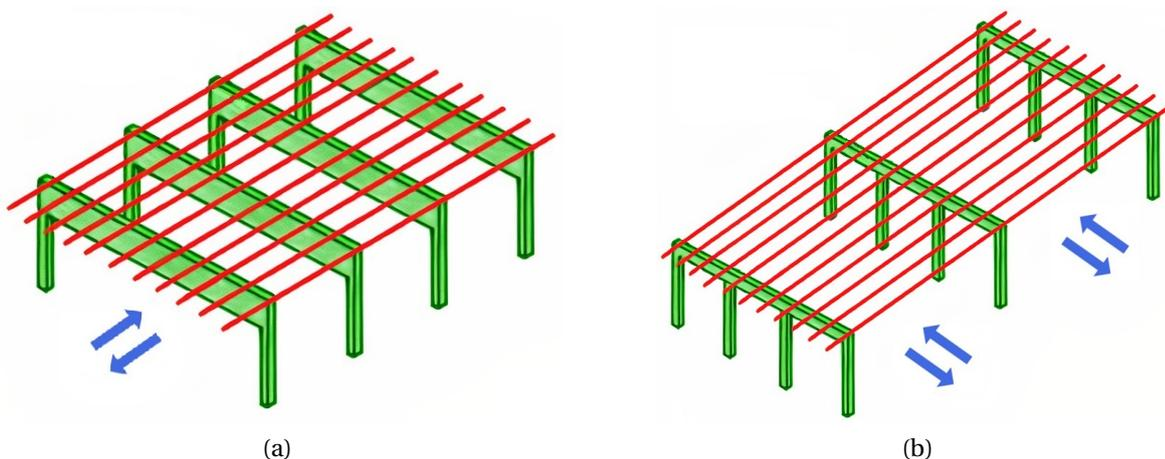
Figure 2.17: Configuration of primary and secondary beams (a) Single hall typology (b) Sub hall typology
