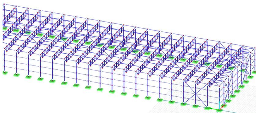
Figure 5.12: ECI optimized design for Coca Cola 27 in RFEM
