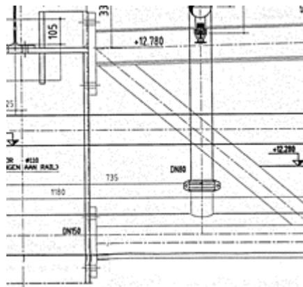
Figure 2.4: Connection detail truss-column [20]
