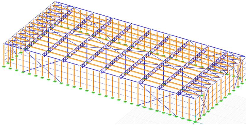
Figure 5.10: RFEM model of multi objective optimized hall
