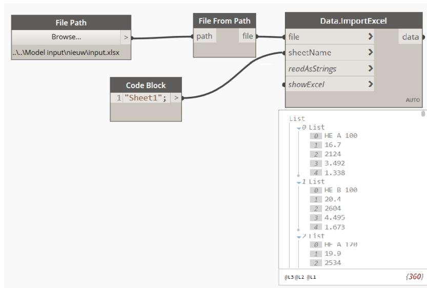
Figure 4.3: Excel input in Dynamo
