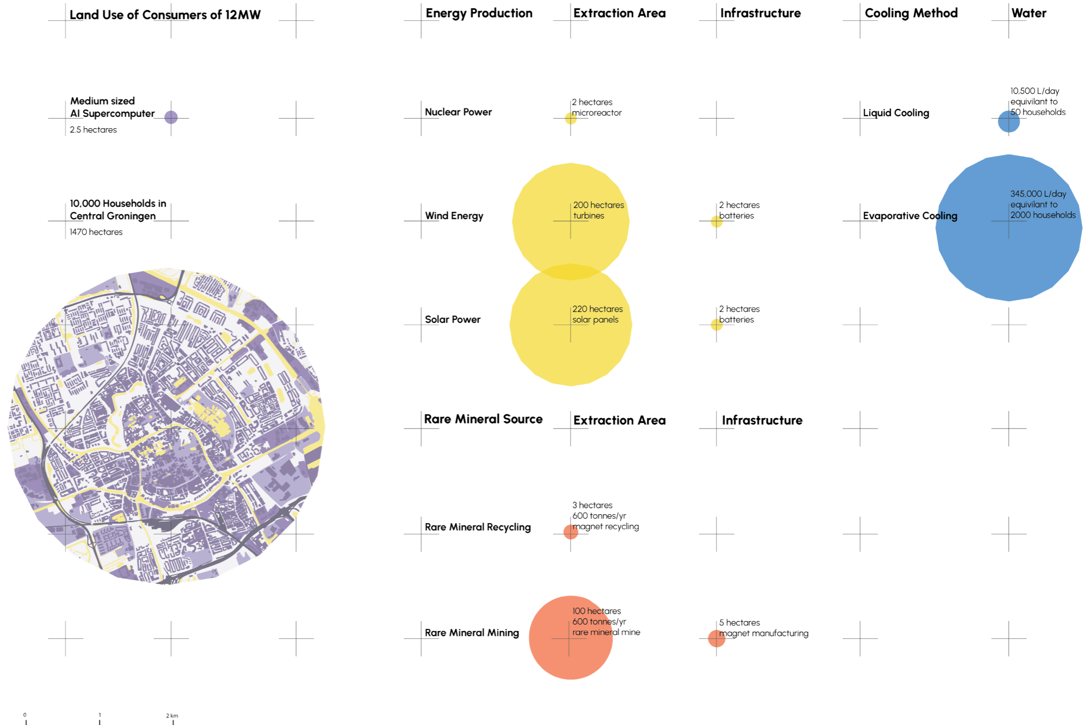
F41. Spatial requirements of different forms of production and consumption of 12 MW AI Supercomputer
