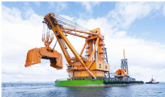
Figure 71: The largest grab dredger in the World: Gosho (200m 3 ) used for a terminal reclamation project in Singapore (2016). It uses a counterweight system to reduce the energy consumption and simplify the hoisting mechanism (source: http://www.kk-kojimagumi.co.jp/english/news/excepteur_sint_occaecat_cupidatat_non.html )
