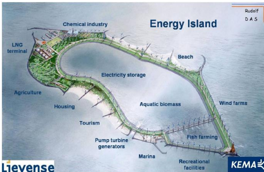
Figure 10: An artist impression of an inverse offshore pumped hydropower storage plant (source: De Boer et al., 2007)
