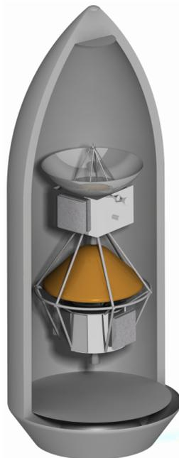
Figure 3.15: Launch configuration shown inside the Falcon 9 fairing.
