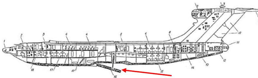
Figure 3.5.2 Side view of Lun-class (hydro ski gear is indicated with arrow) (Yun et al. , 2010)
