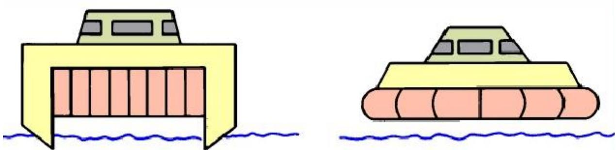
Figure 2.1.3 Illustration of surface effect ship (left) & hovercraft (right) (Darling, 2016)
