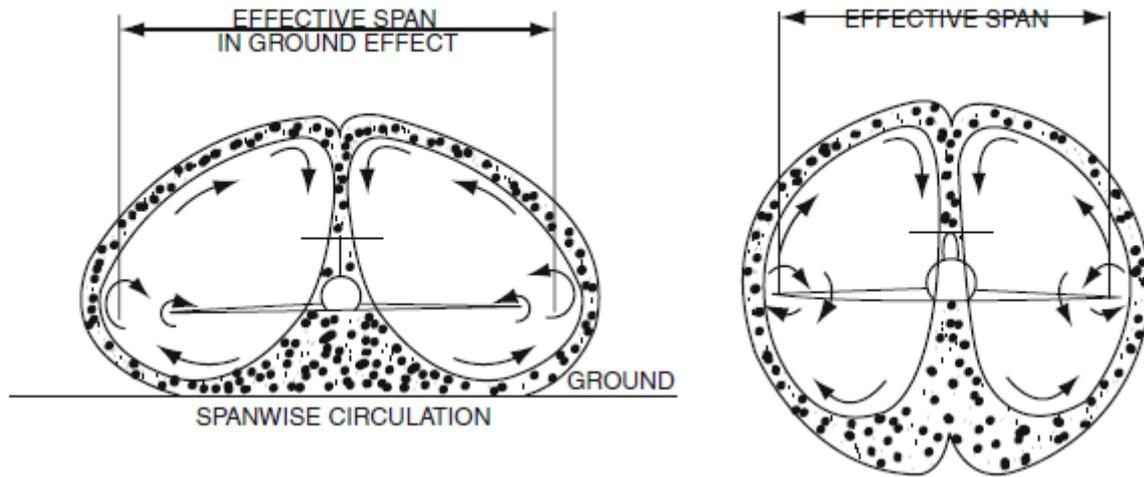
Figure 3.2.2 Illustration of down-wash and lift induced drag in (L) and out (R) of ground effect (Yun et al. 2010)
