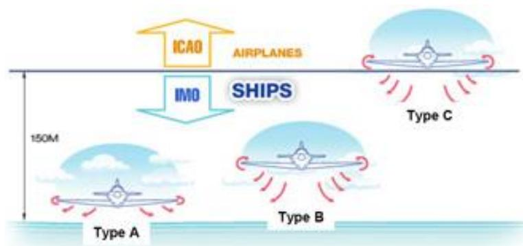
Figure 2.1.5 Illustration of WIG classification types A, B & C (Fischer & Zagklis, WSH-500, 2013)
