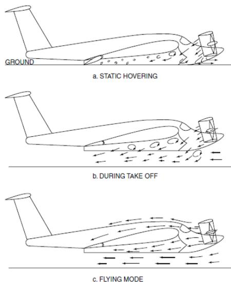
Figure 3.5.6 Illustration of dynamic air cushion WIG vehicle (Yun et al. , 2010)
