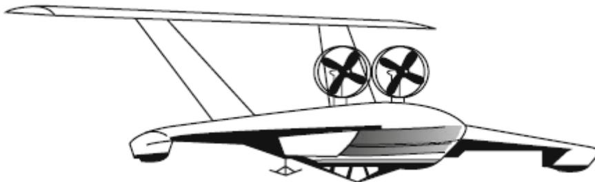
Figure 3.5.8 Design proposal equipped with hydrofoils (Yun et al. 2010)
