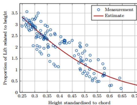
Figure 2.1.8 The relation between the aerodynamic lift force to the ground distance (Hahn et al. 2014)
