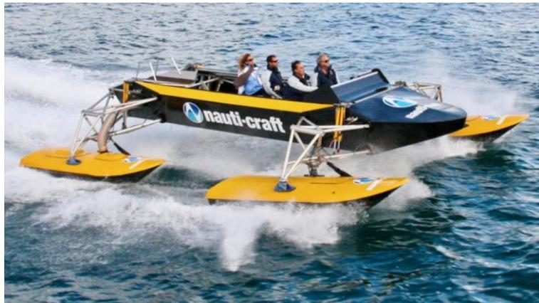
Figure 3.3.3 Quadmaran with hydraulic suspension (Goldberg, 2017)
