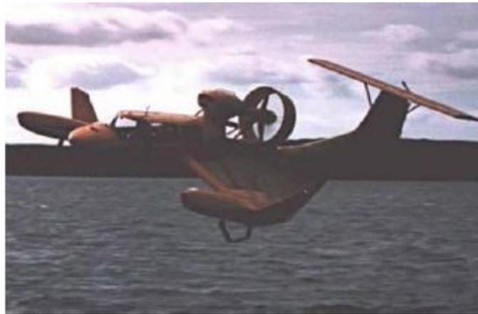
Figure 3.5.7 The X-114 equipped with hydrofoils (Yun et al. 2010)
