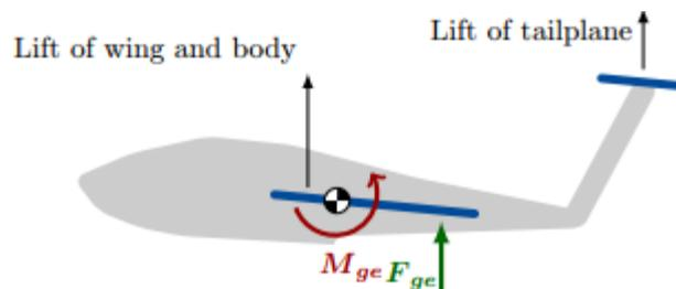
Figure 2.1.7 Illustration of force and moment acting on WIG vehicle in ground effect (Hahn et al. 2014)
