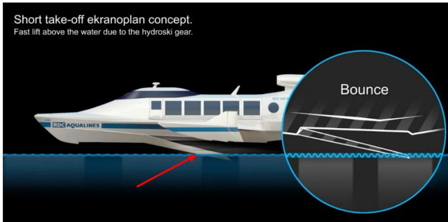
Figure 3.5.1 Illustration of EP-15 (hydro ski gear is indicated with arrow) (Aqualines, 2018)
