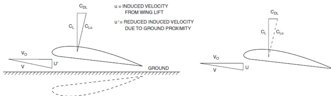
Figure 3.2.1 Illustration of wing in (L) and out of ground effect (R) (Yun et al. 2010)
