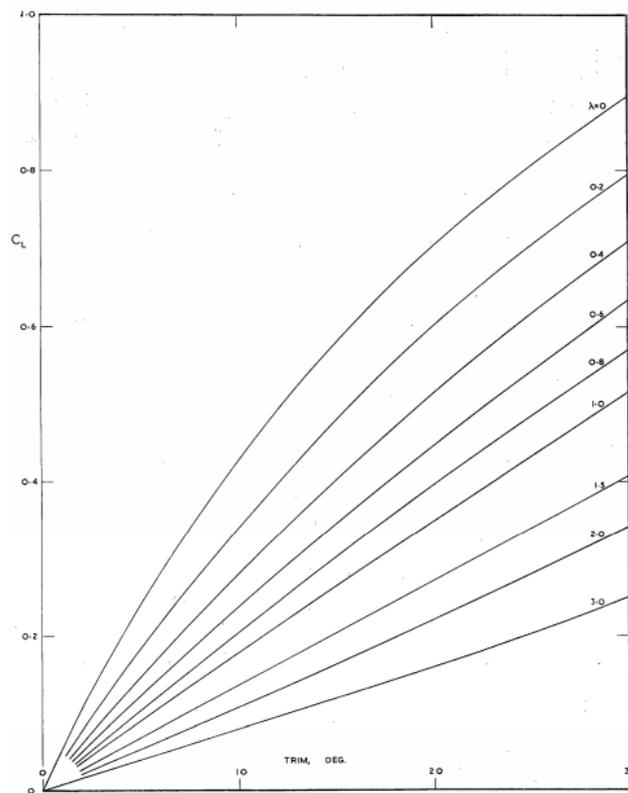
Figure 3.5.4 Lift coefficient curve of flat-plate (Brown, 1957)
