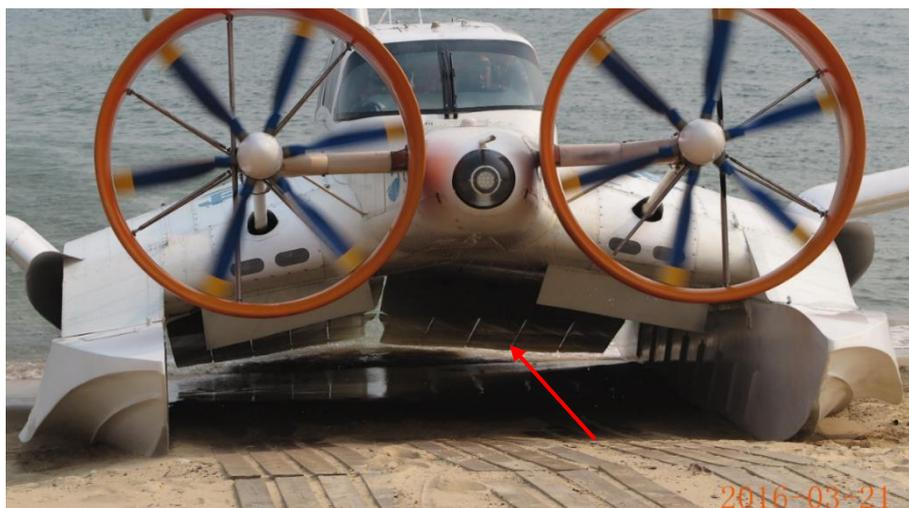
Figure 3.5.3 Picture of Orion 12 (hydro ski gear is indicated with arrow) (Yingge, 2017)
