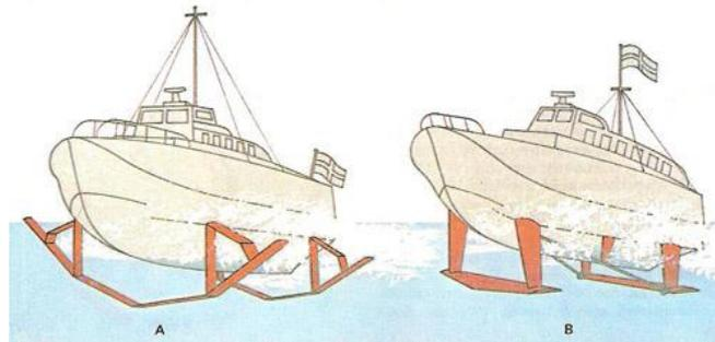
Figure 2.1.2 Illustration of two hydrofoil types – Surface piercing (left) & fully submerged (right) (Darling, 2016)
