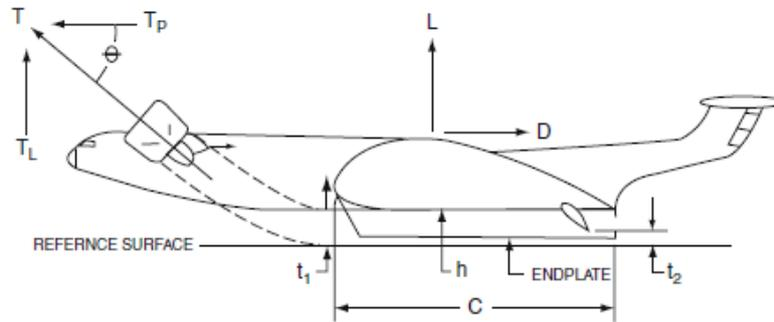
Figure 3.5.5 Illustration of power augmented lift WIG vehicle (Yun et al. , 2010)
