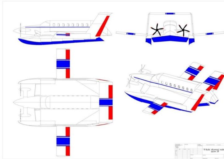
Figure 2.1.16 General arrangement of the Orion 20 (Ekroplani association, 2010)
