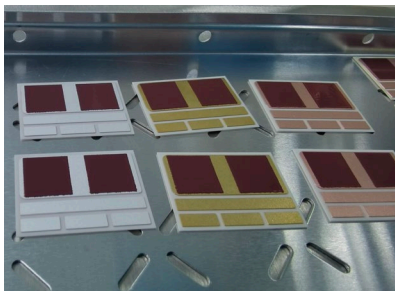
Figure 1 DBC with bare Cu surface, Ag metallization and Au metallization.
