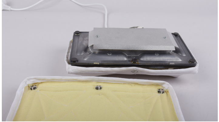
Figure 70. The aluminium cap and Kevlar-lined cover
