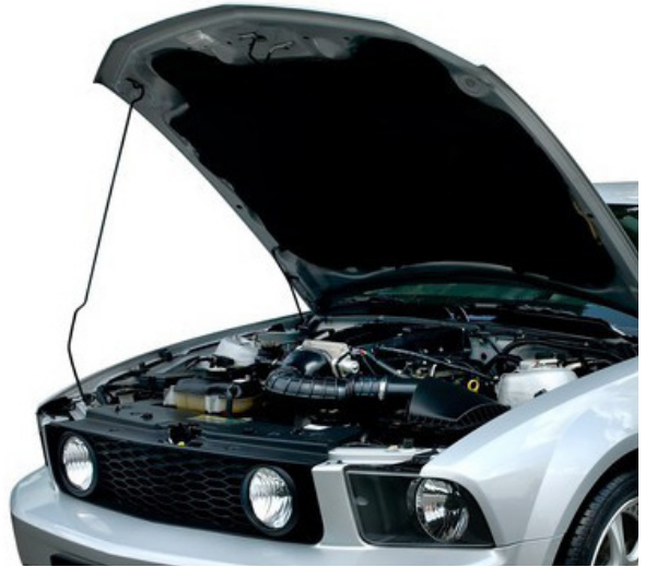
Figure 42. A car hood opened by a rod
