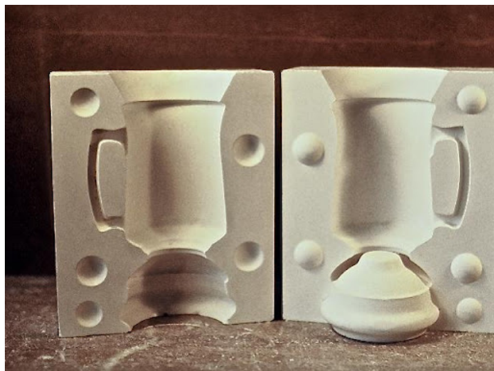
Figure 45. Two halves of a plaster mould, to cast a cup, the ball connectors served as inspiration
