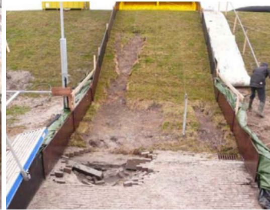
Figure 4-14: Damage transition between different types of revetment
