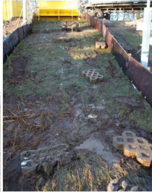
Figure 4-9: Damage transition dike segments in the landward slope
