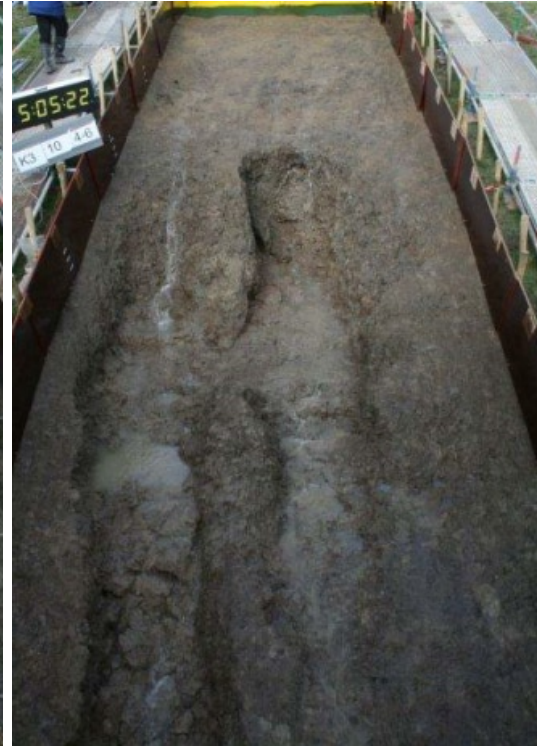
Figure 4-6: Damage holes in the landward slope
