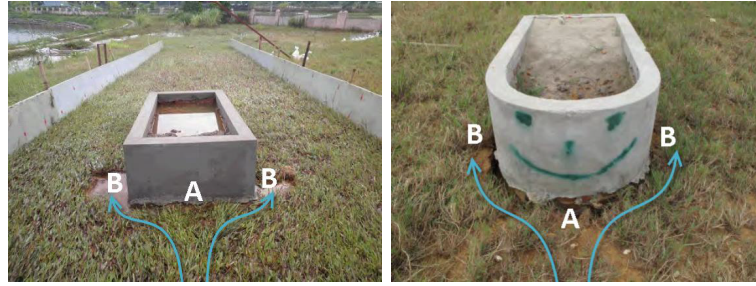
Figure 4-31: Erosion zones A and B around objects Pijpers [2013]
