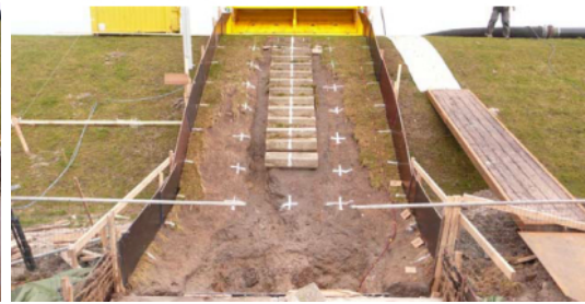
Figure 4-17: Damage NWO staircase landward slope
