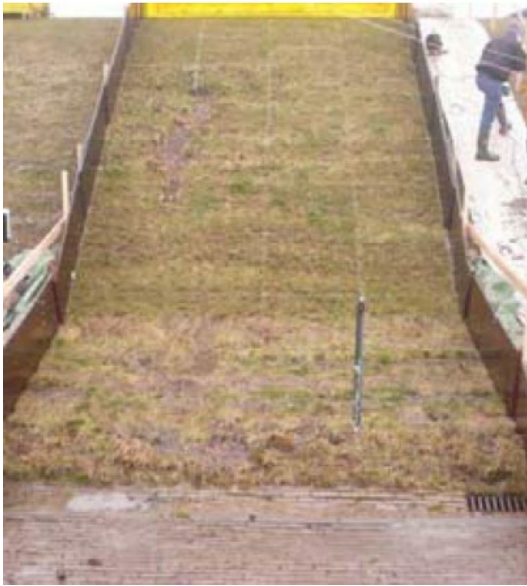
Figure 4-13: Transition between different types of revetment
