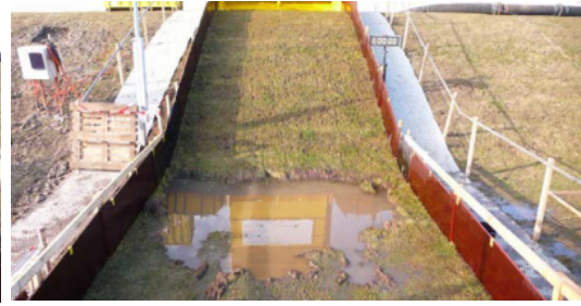
Figure 4-11: Damage transition slope to berm landward slope
