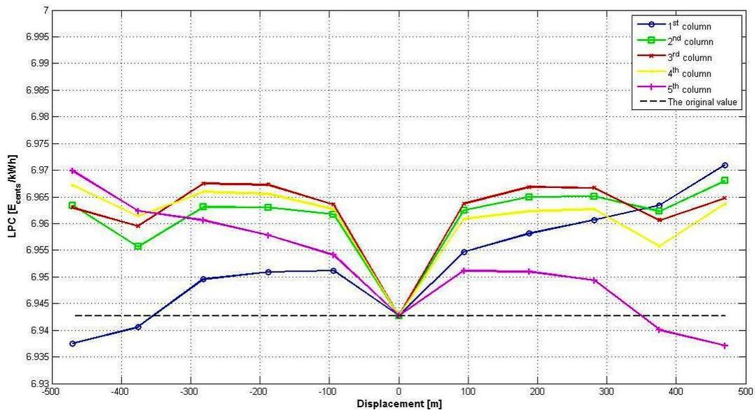
**Figure 4.7:** 25wts-LPC for a column movement along the X-axis. The resulted LPC is illustrated when the original position for all the wind turbines located in the same column is changed. The figure derived after using separately each design variable column of the design vector. To give an example the blue line corresponds to  $\text{Design\_Vector}(1)$
