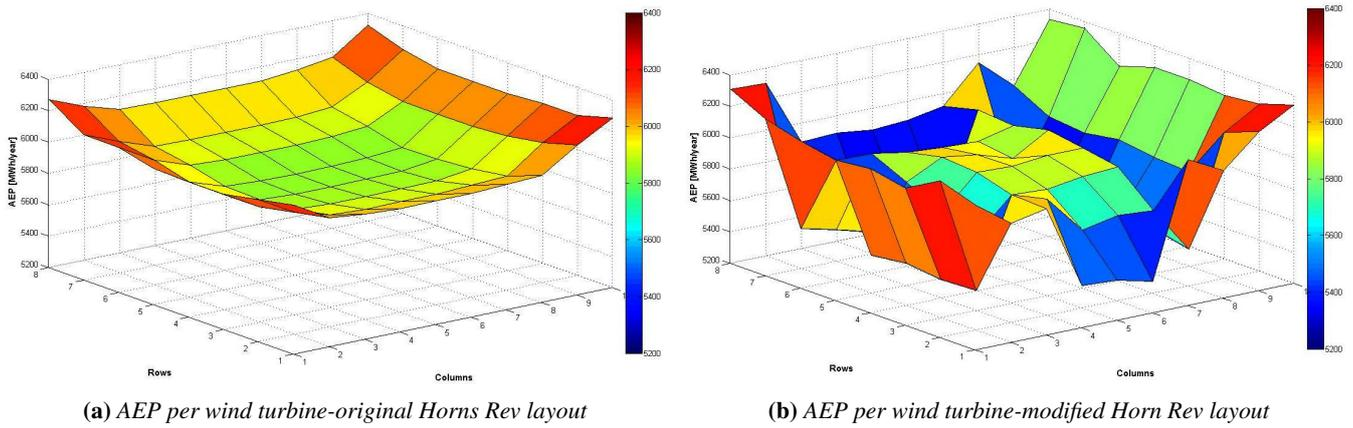
**Figure 5.18:** The Annual Energy Production of each wind turbine for the original and the modified layout-Horns Rev case
