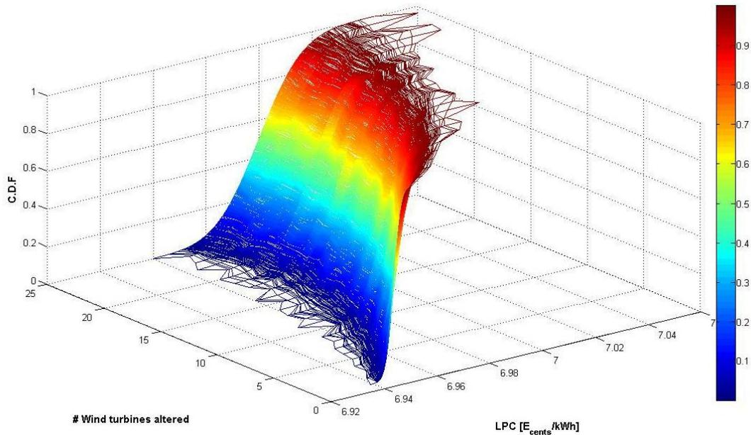
**Figure 5.4:** Cumulative density function of the results obtained for the LPC of an offshore wind farm when the number of wind turbines that are allowed to reposition randomly increases from 1 up to 25
