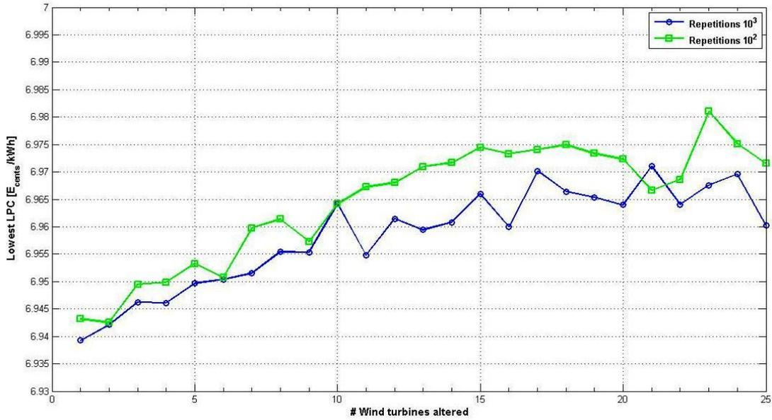
**Figure 5.5:** Lowest LPC values generated by the stochastic process. It is illustrated the cases when a 25 wind turbines wind farm is used and the number of repetitions is set equal to 100 and 1000
