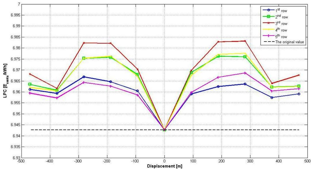
**Figure 4.6:** 25wts-LPC for a row movement along the X-axis. The resulted LPC is illustrated when the original position for all the wind turbines located in the same row is changed. The figure derived after using separately each design variable row of the design vector. To give an example the red line corresponds to Design\_Vector(3)
