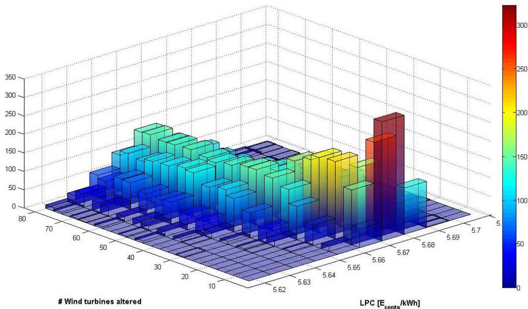
**Figure 5.22:** Histogram per # wind turbines repositioned and LPC for 500 iterations generated by the fully stochastic approach-Horns Rev case
