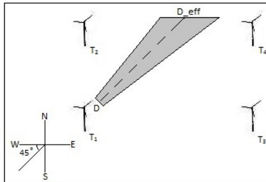
**Figure 4.5:** The expansion of the wake at the downwind row. The wake generated by the upwind turbines affects a larger area when the wind farm rows are not perpendicular to the incoming wind
