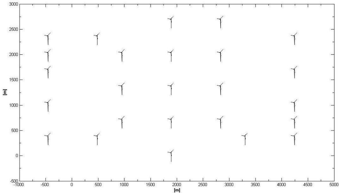
**Figure 5.1:** Individual turbine optimum position-Layout of 25 wind turbines. The layout results when the optimum position for each individual wind turbine is considered as it is explained thoroughly in section 4.7 the original layout can be found in Figure 4.1
