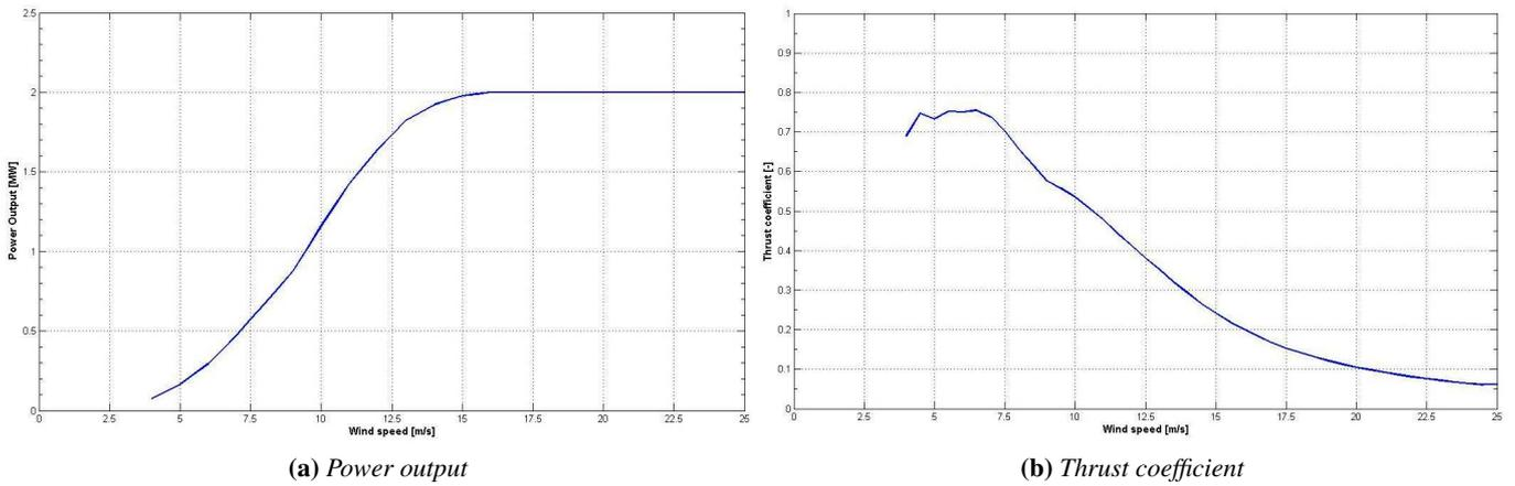
**Figure 4.3:** The characteristic curves of Vestas V80 wind turbine
