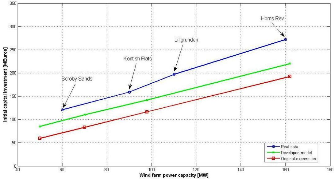
**Figure 3.6:** The initial capital investment versus the wind farm capacity. The real data correspond in the cases of Scroby Sands, Kentish Flats, Lillgrunden and Horns Rev are illustrated [35]
