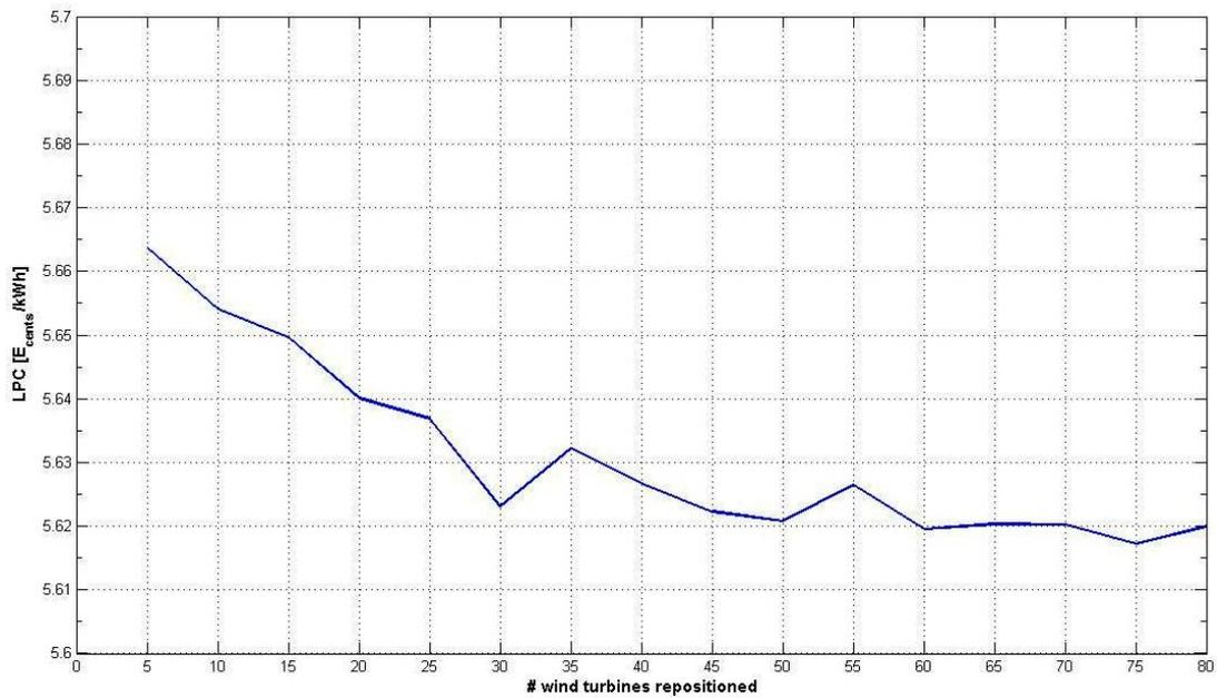
**Figure 5.24:** Lower LPC values obtained by the fully stochastic approach per # of wind turbines relocated-Horns Rev case
