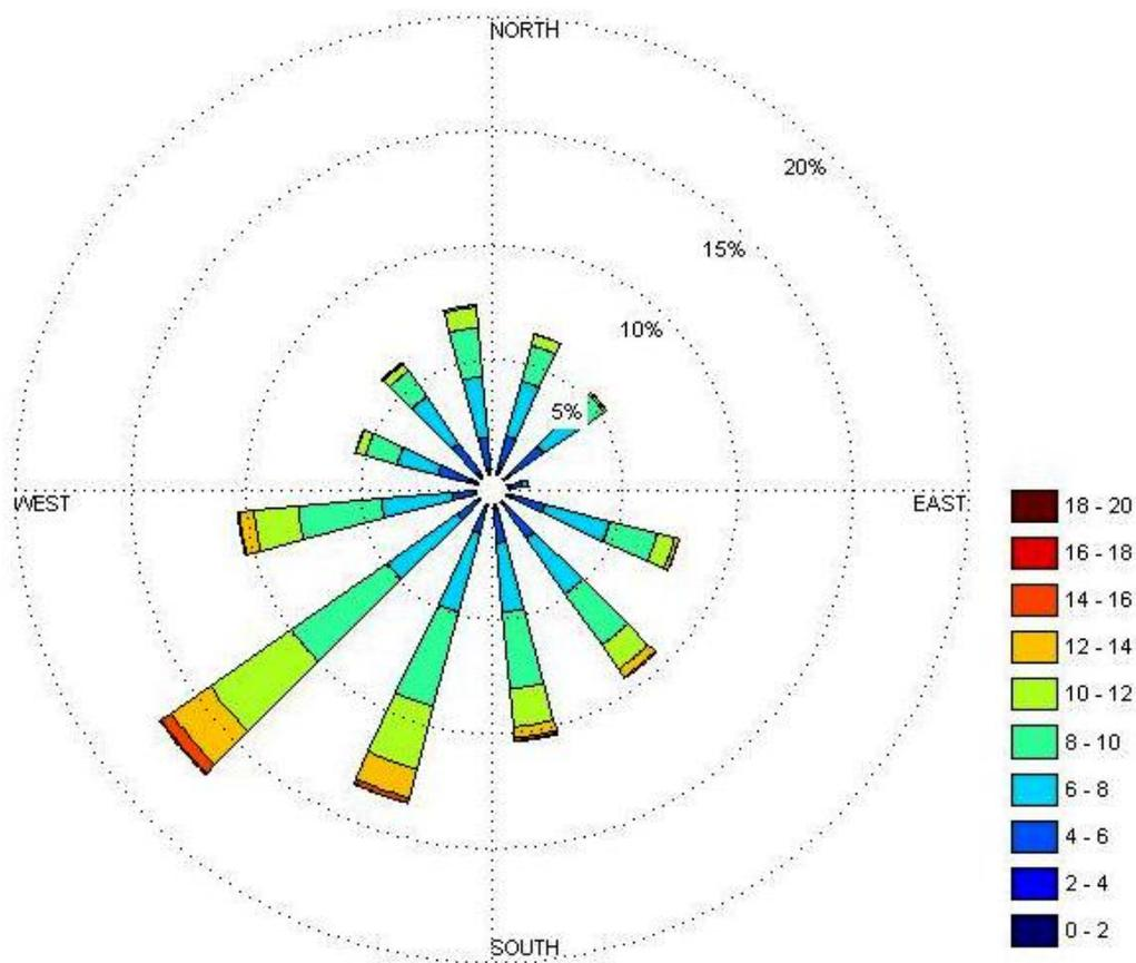
**Figure 5.14:** Wind rose with 12 sectors which is used in the calculations of Horns Rev offshore wind farm
