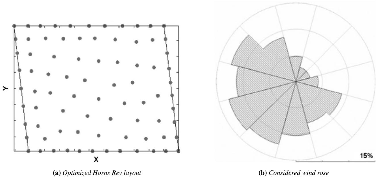
**Figure 5.13:** Optimized layout and considered wind rose for the Simulated Annealing algorithm [20]
