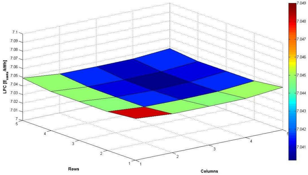
Figure 4.16: LPC estimation for the removal of individual wind turbines
