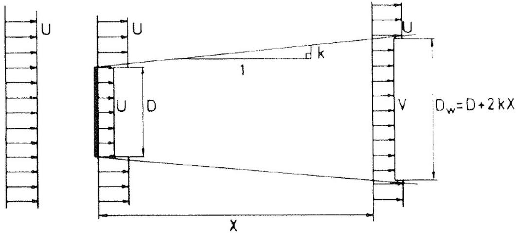
**Figure 3.2:** Jensen model. The figure presents the linear expansion of a wake. Moreover, the equation used for the wake diameter after a given distance, depicted as  $x$ , is shown [28]
