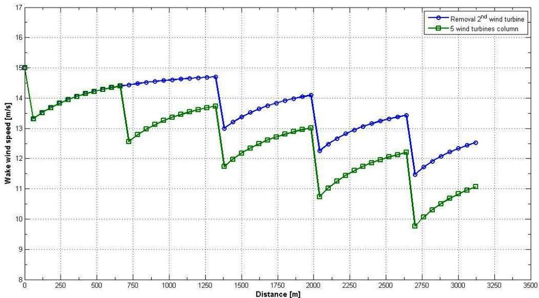
**Figure 4.12:** Wake wind speed vs Distance. Second wind turbine removal
