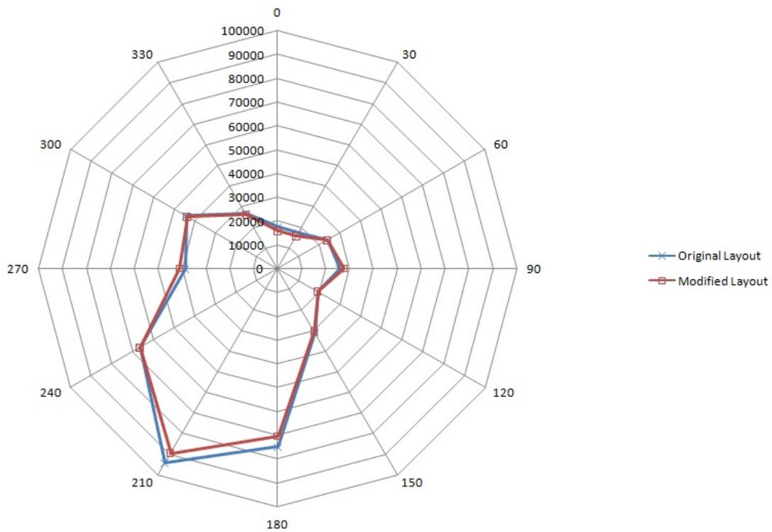
Figure 5.17: Energy production comparison when the original and the modified layout are considered. The original layout is formed having 7D as separation distance for the rows and columns. The modified layout resulted from the best, in terms of LPC estimation, possible combinations of the individual wind turbine movement. The locations of the wind turbines can be seen in Figure 5.15. The energy production is shown in  $MWh/year$
