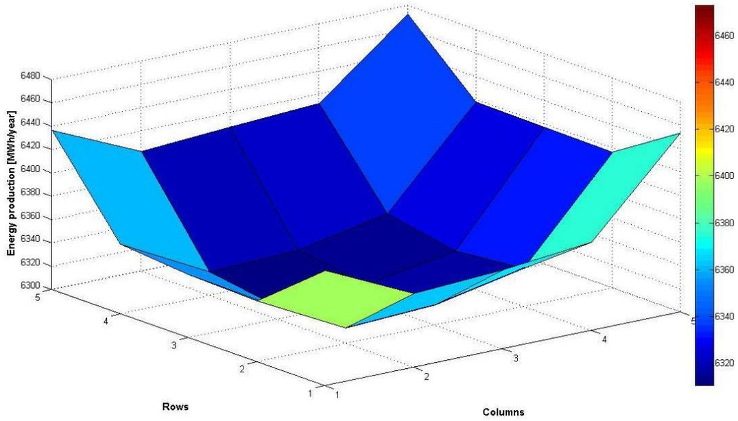
Figure 4.17: Annual energy production per turbine in a 25 wind turbines farm
