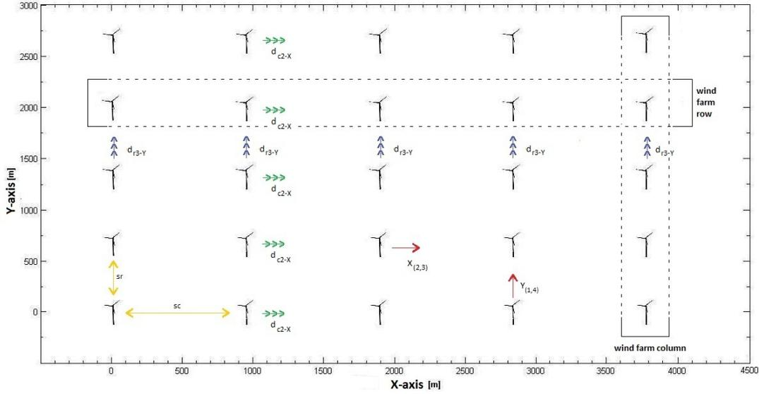
**Figure 4.1:** The original wind farm layout for a wind farm, which is consisted of 25 wind turbines is shown. The separation distances are the same as the ones listed in Table 3.4
