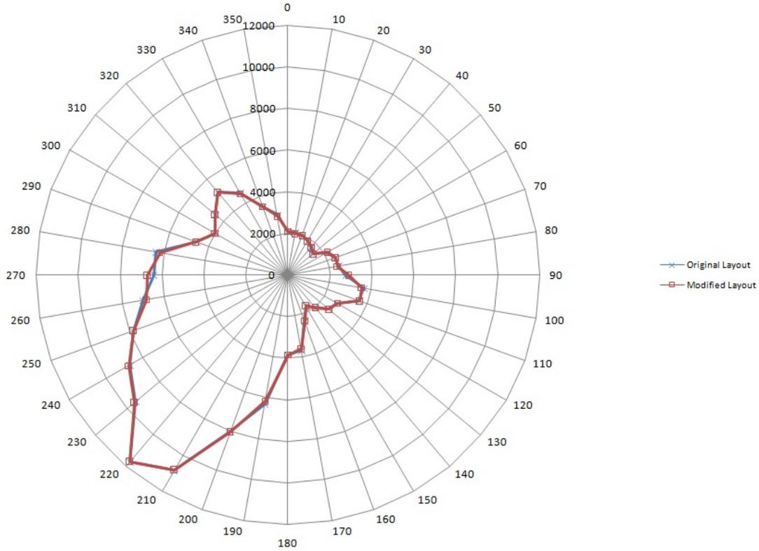
**Figure 5.2:** Energy production comparison when the original and the modified layout are considered. The original layout is formed having  $8.25D$  as separation distance for the rows and  $11.75D$  as separation distance for the columns. The modified layout resulted from the best, in terms of LPC estimation, possible combinations of the individual wind turbine movement. The locations of the wind turbines can be found in the Positioning Matrix. The energy production is shown in  $MWh/year$
