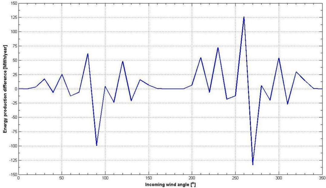
**Figure 4.11:** 25wts-Energy production difference. Y-axis movement. The energy produced per wind direction by the modified layout is subtracted from the energy produced per wind direction by the original layout. The original layout corresponds to a separation distance for the rows and columns of  $8.25D$  and  $11.75D$  respectively. The modified layout has the first column of the wind farm relocated to  $-150m$  from its initial position
