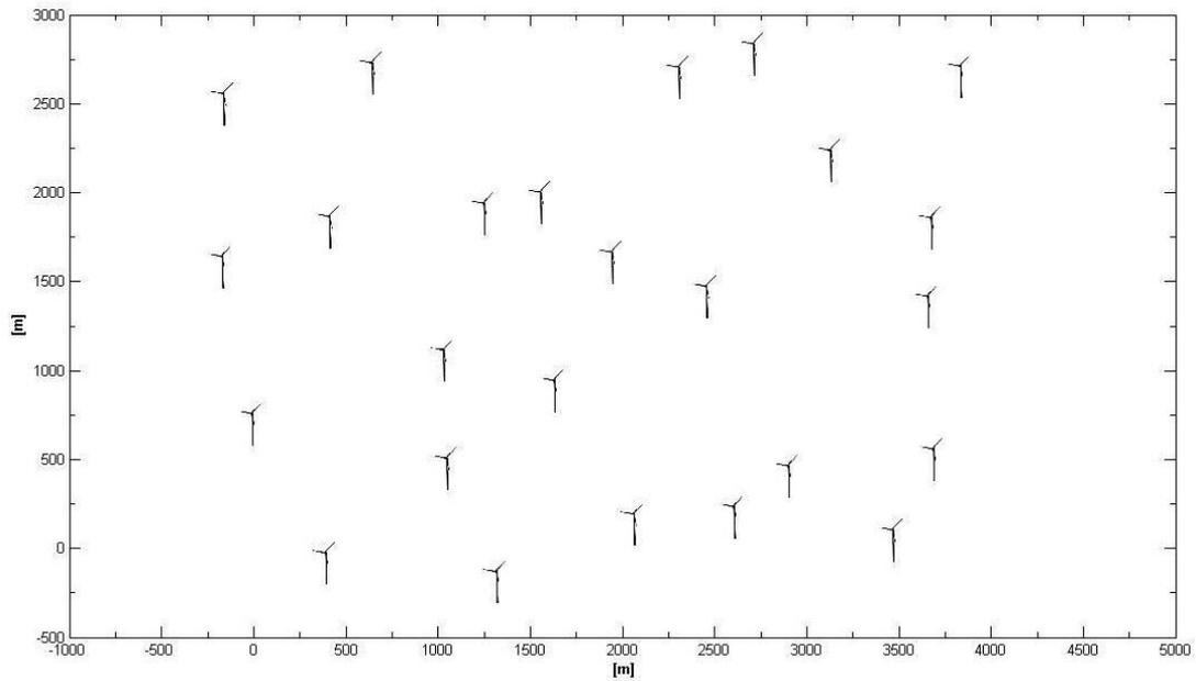
**Figure 5.3:** Example for the layout when 25 wind turbines are randomly placed within the predefined range
