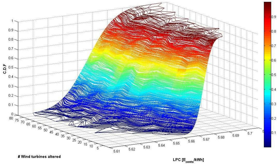
**Figure 5.23:** Cumulative density function for the fully stochastic approach-Horns Rev case
