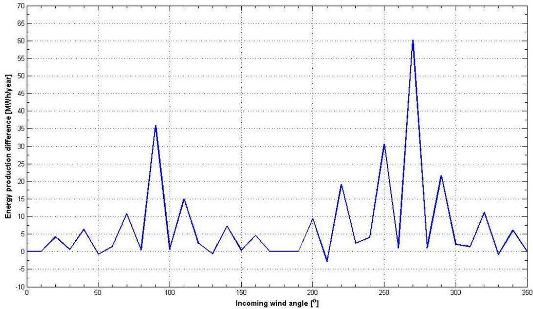
**Figure 4.8:** 25wts-Energy production difference. X-axis movement. The energy produced per wind direction by the modified layout is subtracted from the energy produced per wind direction by the original layout. The original layout corresponds to a separation distance for the rows and columns of  $8.25D$  and  $11.75D$  respectively. The modified layout has the first column of the wind farm relocated to  $-450m$  from its initial position
