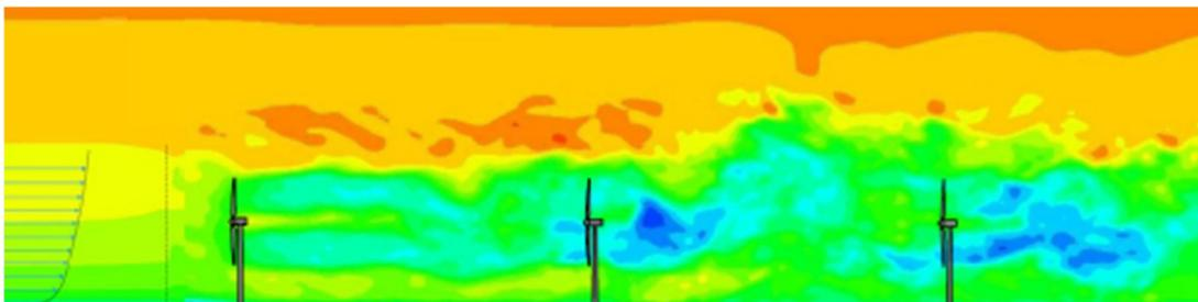
**Figure 3.1:** Wake propagating behind rotating wind turbine rotors. The reduced wind speed, indicated by a color tone close to blue, behind each rotor can be observed. Moreover, the increased turbulence intensity experienced by the downwind turbines is shown [26]
