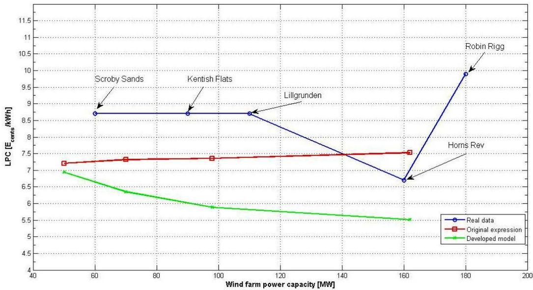
**Figure 3.5:** The cost of energy versus the wind farm capacity. The depicted real data correspond in the cases of Scroby Sands, Kentish Flats, Lillgrund, Horns Rev and Robin Rigg [35]
