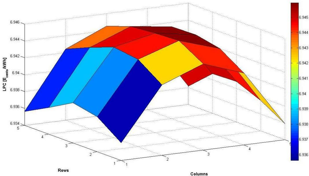
Figure 4.14: LPC results for the individual movement of each wind turbine of the offshore wind farm
