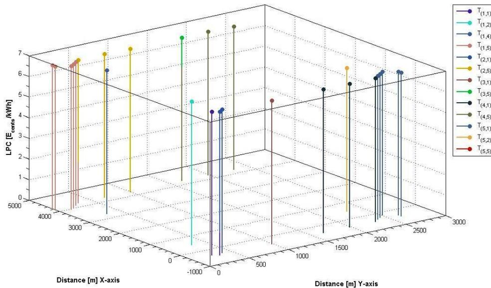
**Figure 4.15:** Position of the wind turbines that improve the LPC. The X- and Y-coordinate of  $T_{(:,1)}$ ,  $T_{(:,5)}$ ,  $T_{(1,2)}$ ,  $T_{(5,2)}$  and  $T_{(1,4)}$  are shown
