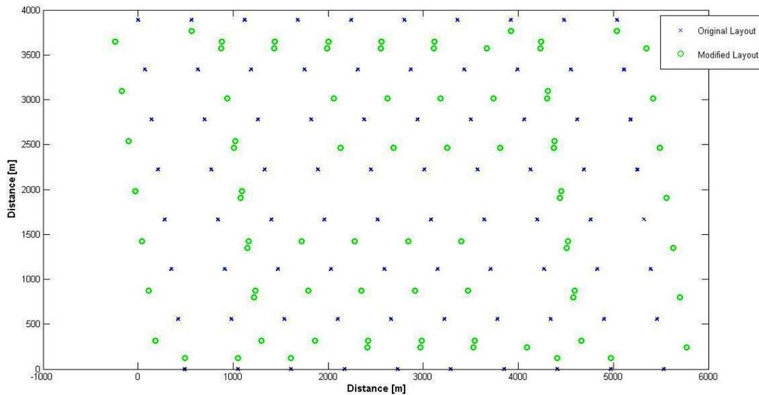
**Figure 5.15:** The Horns Rev offshore wind farm modified layout. The figure depicts the suppositions of the best layout when one turbine at the time is repositioned while it also shows the modified layout. This layout results by the deterministic approach and stems from the combination of the best solutions obtained for each turbine individually
