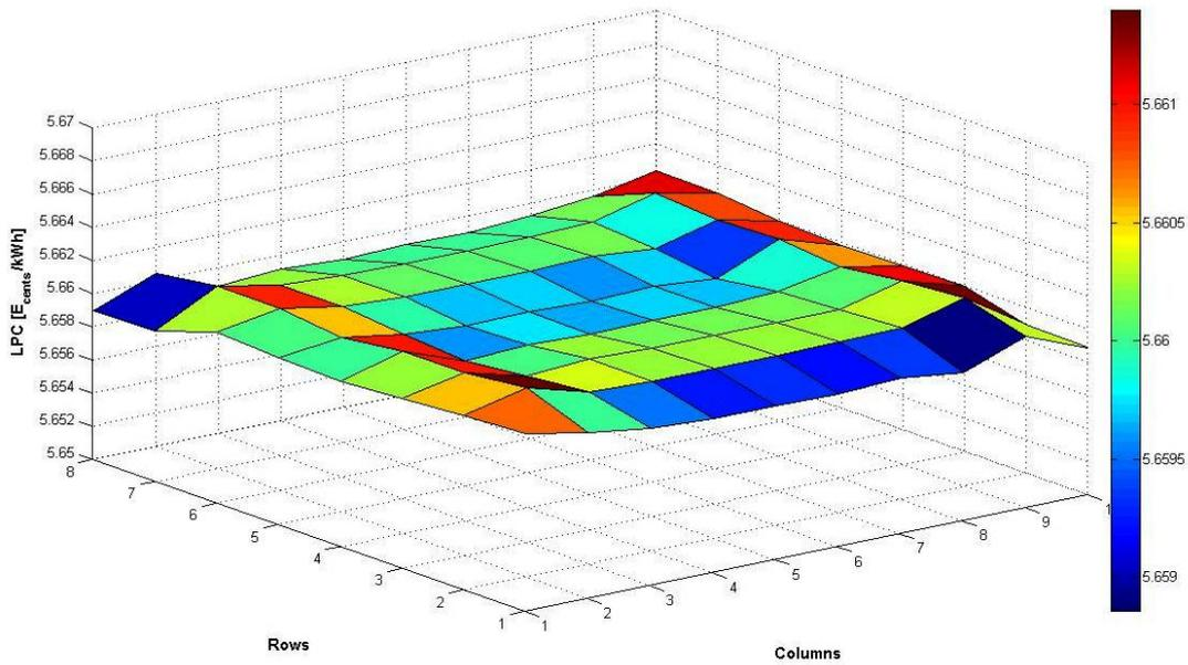
Figure 5.16: LPC for the individual movement of Horns Rev offshore wind farm
