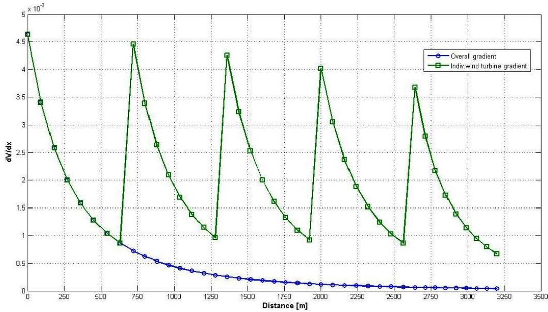
**Figure 4.4:** Wake wind speed gradient for the Jensen model. The curve resulted from the expression (4.1) and it steeply decreases for the first ~ 650m while afterwards the rate drops. The gradient for the consecutive wind turbines is represented with the green curve
