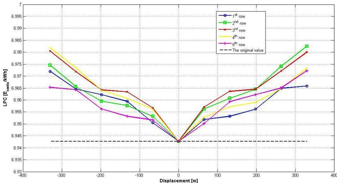
**Figure 4.9:** 25wts-LPC for a row movement along the Y-axis. The resulted LPC is illustrated when the original position for all the wind turbines located in the same row is changed. The figure derived after using separately each design variable row of the design vector
