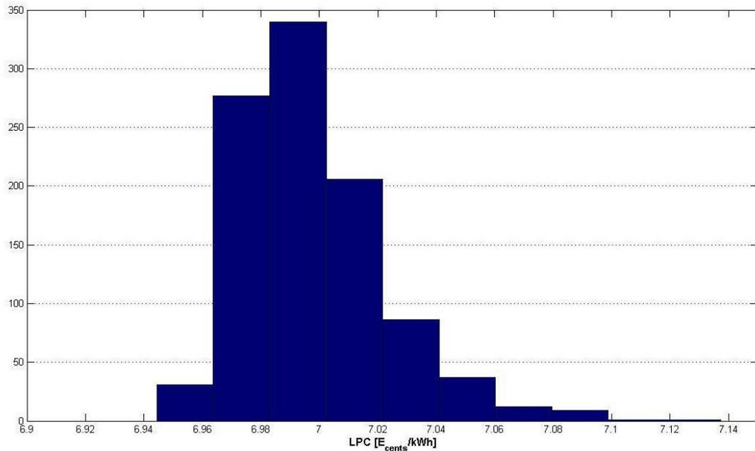
**Figure 5.11:** Histogram for the stochastic process when individual wind turbines movement and column movement is considered
