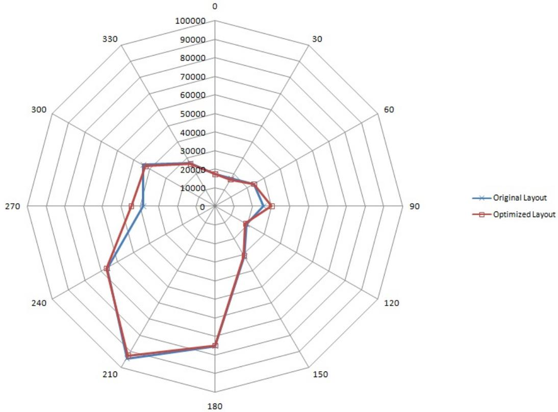
**Figure 5.21:** Energy production comparison when the original and the optimized layout are considered for the case of Horns Rev offshore wind farm. The optimized layout resulted from the best sample, in terms of LPC estimation, of the semi-stochastic approach. The energy production is shown in  $MWh/year$
