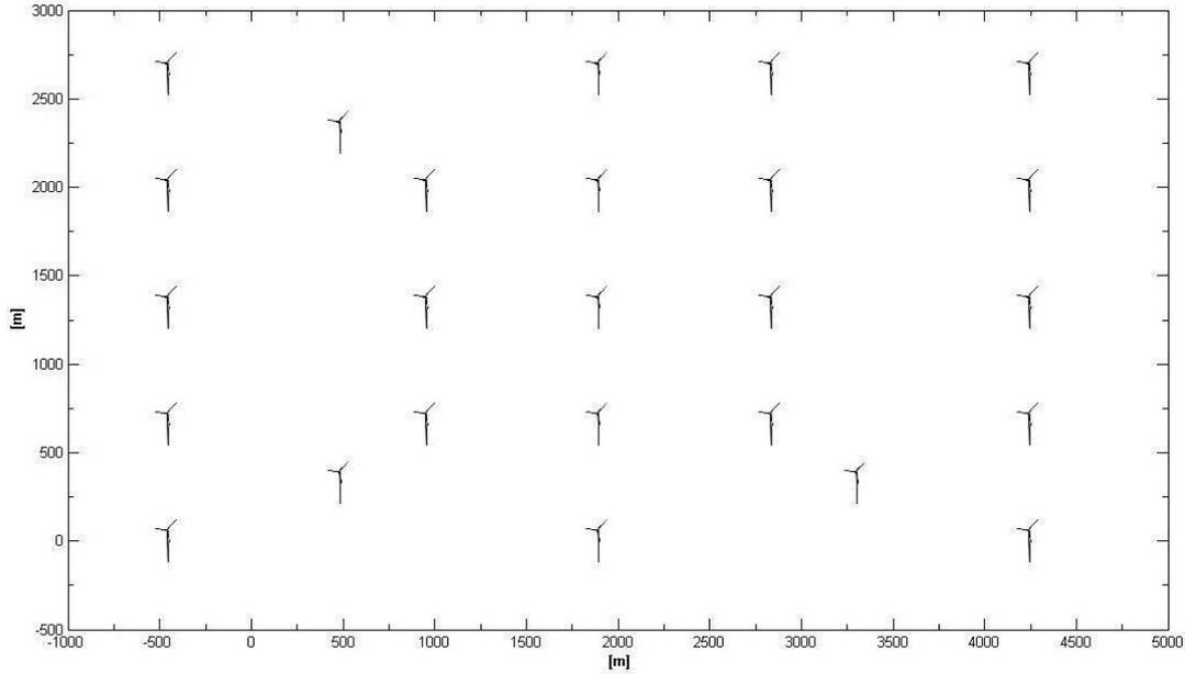
**Figure 5.8:** The layout of the offshore wind farm when the first and fifth columns of the farm are relocated according to the solution found in section 4.4.2 while,  $T_{1,2}$ ,  $T_{1,4}$  and  $T_{5,2}$  change positions as proposed by the positioning matrix in section 4.7. Mind the same, as the original, y-coordinates of the turbines in the first and fifth columns
