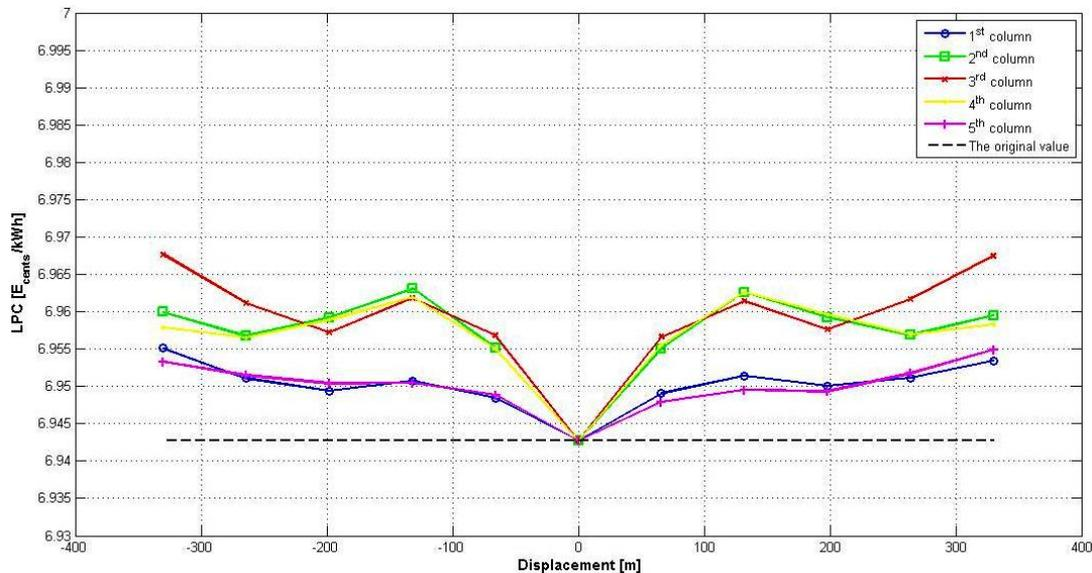
**Figure 4.10:** 25wts-LPC for a column movement along the Y-axis. The resulted LPC is illustrated when the original position for all the wind turbines located in the same column is changed. The figure derived after using separately each design variable row of the design vector
