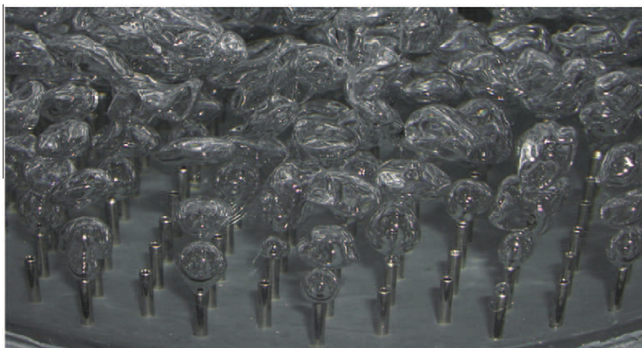
Fig. 1. A photo of a needle sparger used in a slurry bubble column with one-third of the needles in operation. By using long needles instead of holes, a much higher pressure drop is achieved, which leads to a much more uniform bubble size and consequently a lowered E_L [31].
