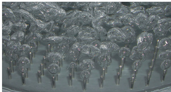
Figure 5. Bubble formation by a needle sparger in a bubble column with one-third of the needles in operation (Mudde et al., 2009).
