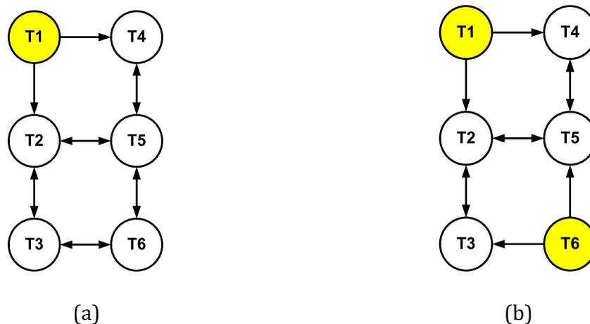
Fig. 8. (a) Directed graph to incorporate all possible sequences of events triggered by a primary event at T1 (SPE domino effect). (b) Directed graph to incorporate all possible sequences of events triggered by two simultaneous primary events at T1 and T6 (MPE domino effect).
