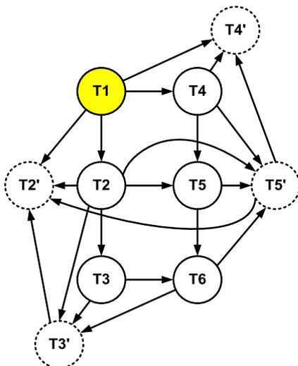
Fig. 5. Application of auxiliary nodes (dashed outlined) to address domino effect model uncertainty in a process plants with six storage tanks.
