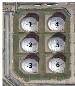
**Fig. 7.** Tank farm consisting of six atmospheric storage tanks containing gasoline. The tanks are identical, with a diameter of D = 33.5 m, height of H = 9.1 m, and capacity of V = 8000 m<sup>3</sup>.
