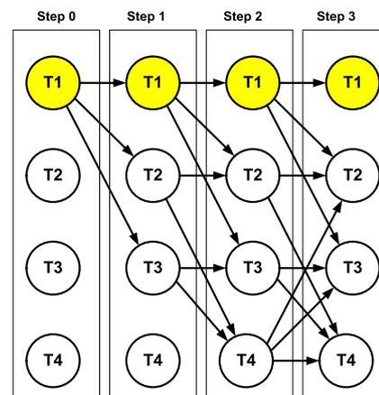
Fig. 6. Dynamic Bayesian network to address domino effect model uncertainty in a process plant comprising four units T1-T4. The domino effect initiates at T1.
