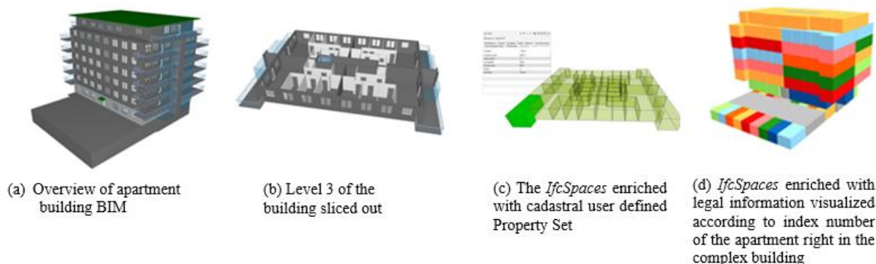
Figure 4. BIM enriched with legal space through a user defined property set visualised with Solibri Model Viewer. Figure (d) visualised with QGIS (Meulmeeste, 2019)
