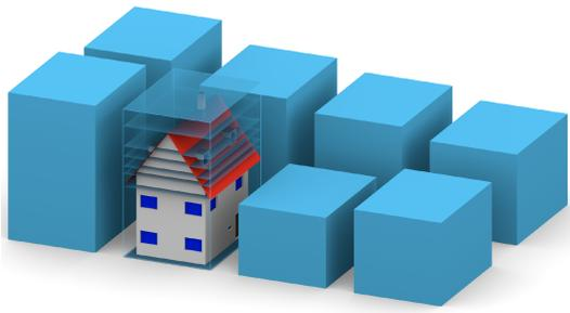
(a) Different height references for the top surface of an LOD1 model. Reprinted from Biljecki et al. (2014).
