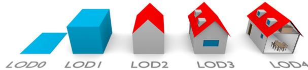
Figure 3: The five LODs defined by the OGC CityGML 2.0 standard. Reprinted from Biljecki et al. (2016a).
