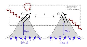
FIG. 1. (Color online) Schematic illustration of the DQD system under study. Two nuclear spin ensembles are hyperfine-coupled to the electronic subsytem; due to various *fast* coherent (double-arrow) and incoherent processes (arrows) the latter settles to a quasisteady state on a time scale shorter than the nuclear dynamics.
