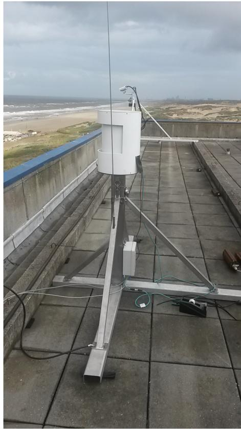
**Figure 3.4:** Photo of the scanner setup mounted on the hotel overlooking the Kijkduin beach. Image courtesy of S. Vos.
