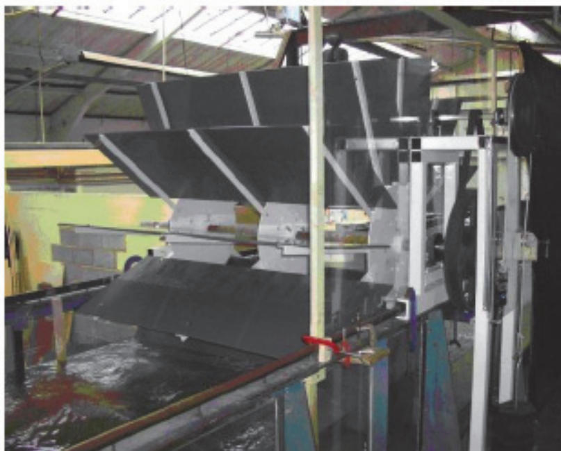
Figure 7-6: Hydrostatic pressure wheel in the laboratory flume
