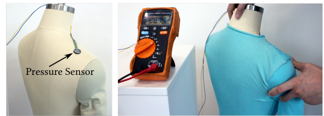
Fig. 20. A pressure sensor is used to measure pressure at the shoulder point on the mannequin. Pressures can be calibrated from the readings of a universal meter (middle) that measures electric resistance.
