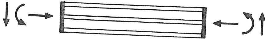
Figure 12a Schematic representation of beam-column element divided in three sub elements (two-dimensional)
