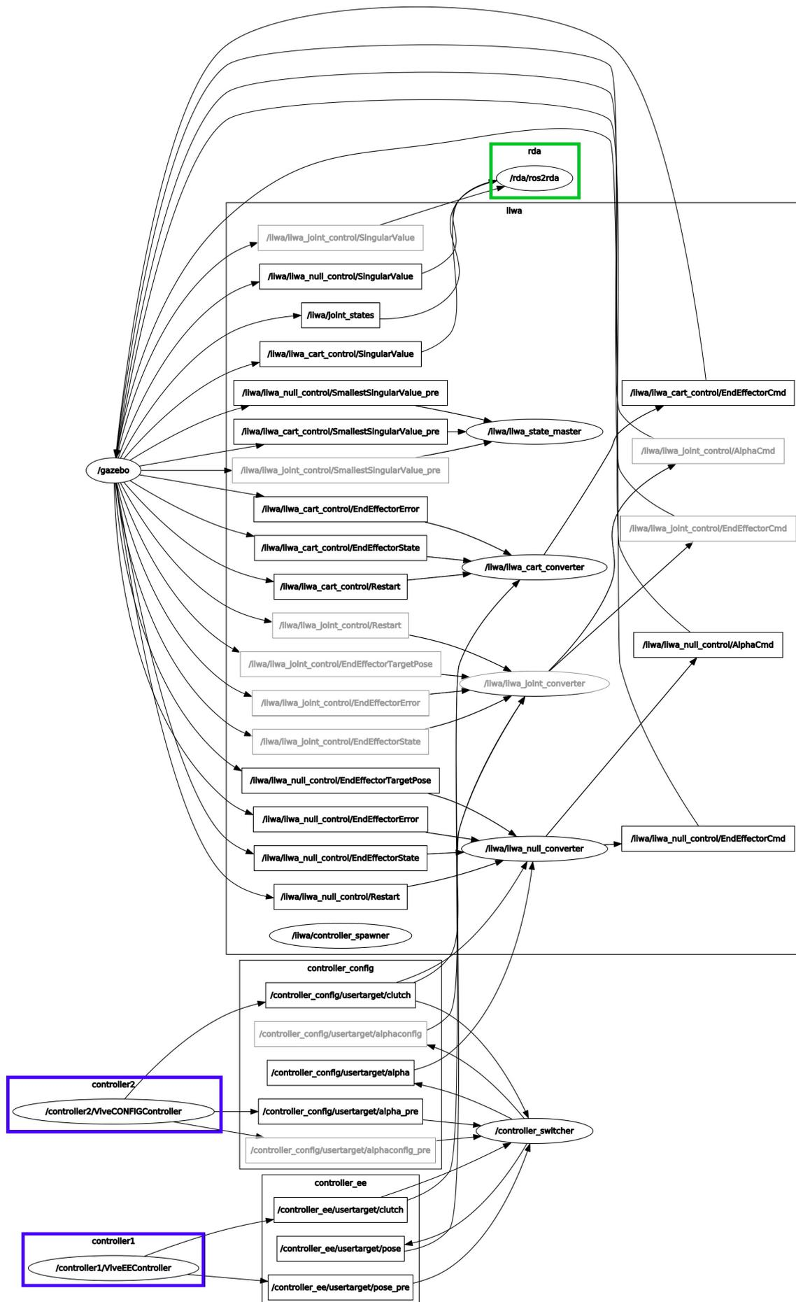
Figure D.1: ROS control scheme containing all nodes (processes) and topic (communication between processes) of the slave device system. Nodes that are faded, are nodes that are in the ROS control scheme but are not used for the experiment. The blue squares indicate the node where data enters the slave system. The green square indicates the node where the data leaves the slave system.
