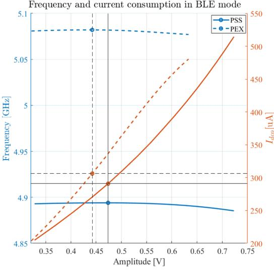
Figure 3.35: BLE frequency and current consumption as function of the amplitude. With active devices biased at  $V_{bp} = 0$  V and  $V_{bn} = 0$  V
