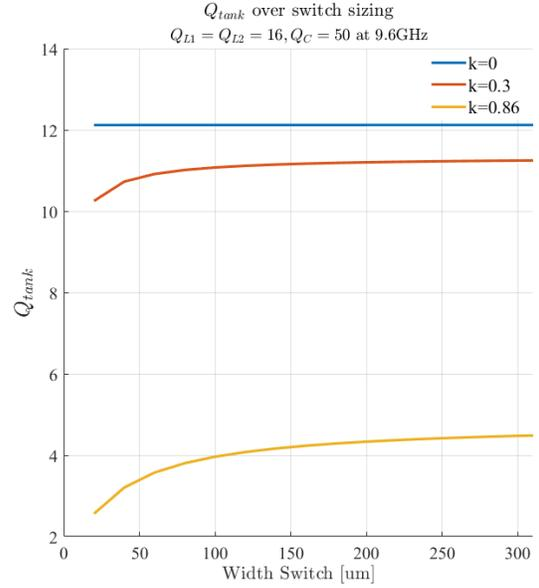
Figure 3.10:  $Q_{tank}$  calculated with the added  $R_{ON}$  from the HVTH switch, biased at 0V. With  $L_1 = 3.92$  nH and  $L_2 = 0.98$  nH.
