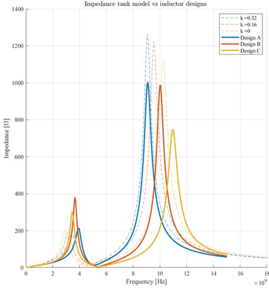
Figure 3.23: Tank impedance compared with EMX inductor designs and a lumped model with similar  $k$ .
