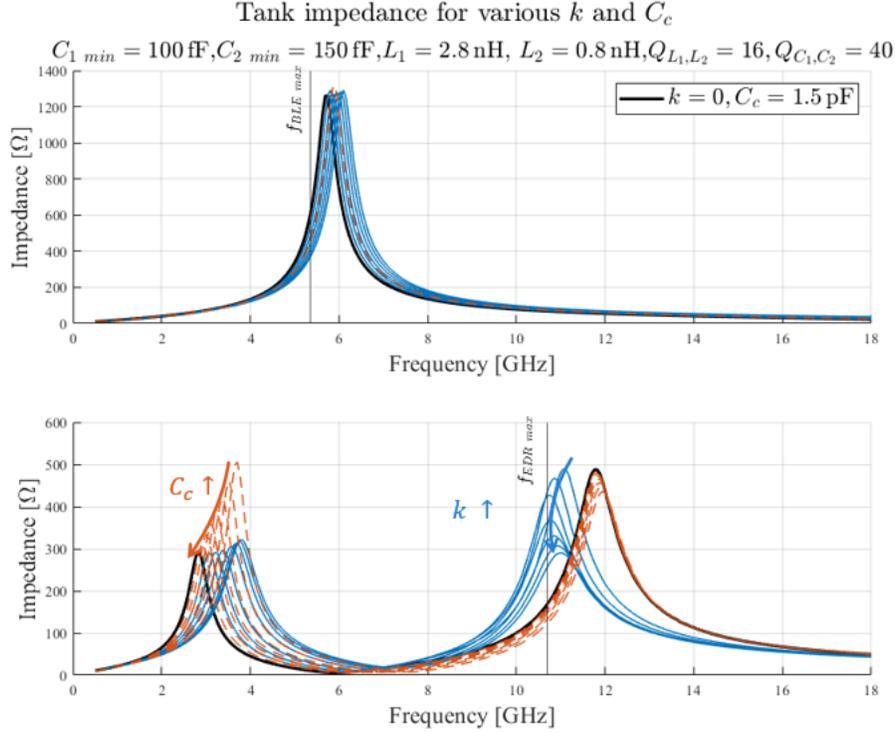
Figure 3.21: Simulated tank impedance for each BLE/EDR mode with lumped components, orange describes the increase of  $C_c$ , while the blue describes the increase in  $k$ .
