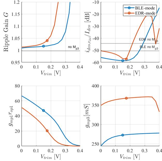
Figure 4.6: The effect on gain ripple  $G$ , current injection ratio  $\frac{i_{dco,vdd}}{I_{dco}}$ , the  $g_{mp1}r_{op1}$  product and the  $g_{mp3}$  over various gate voltages at  $M_{p3}$ .
