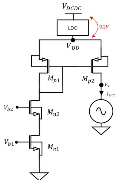
Figure 4.1: Conventional Current mirror topology with cascoded current source ( $M_{n1}, M_{n2}$ ) with LDO.
