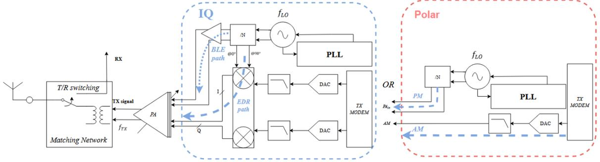
Figure 1.5: Transmitter with IQ mixer and polar on the left and right respectively for 8-DPSK modulation
