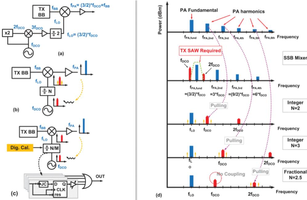
Figure 1.9: Conventional synthesizers ideas: (a) SSB mixer [50], (b) Integer divider, (c) Fractional divider [51].
