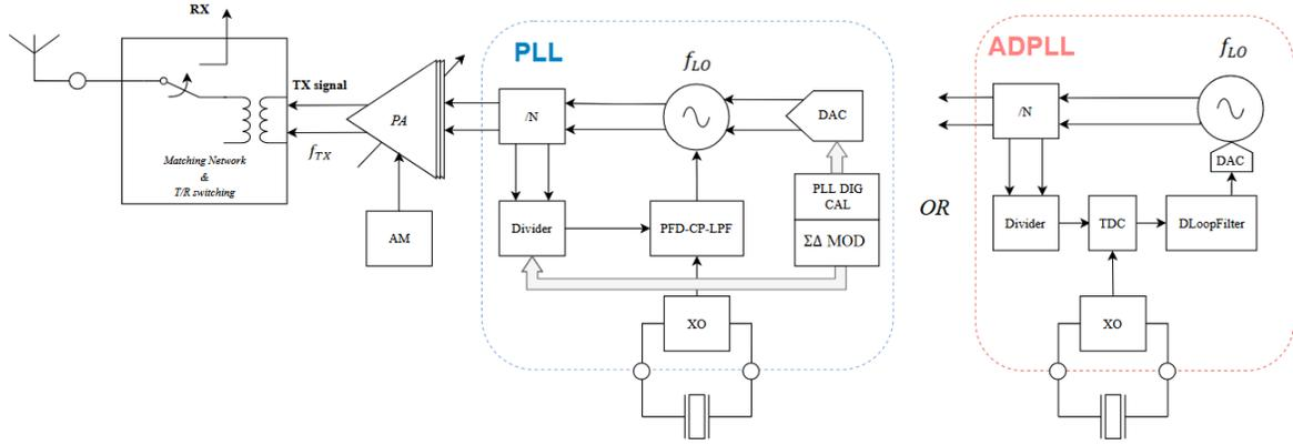
Figure 1.6: transmitter with direct frequency modulation created by the analog PLL or all digital PLL.
