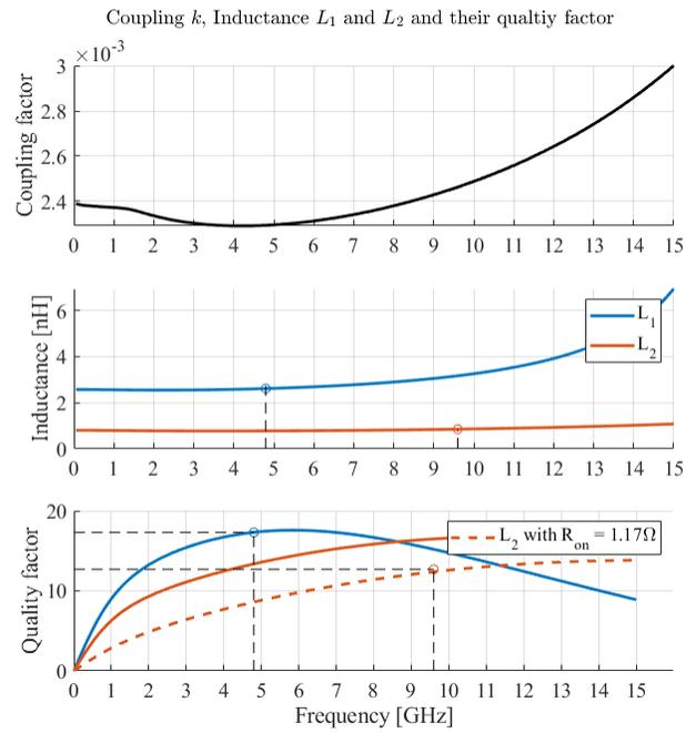
Figure 3.26: Characteristics  $k, Q_L$  and  $L_{1,2}$  for the proposed design.
