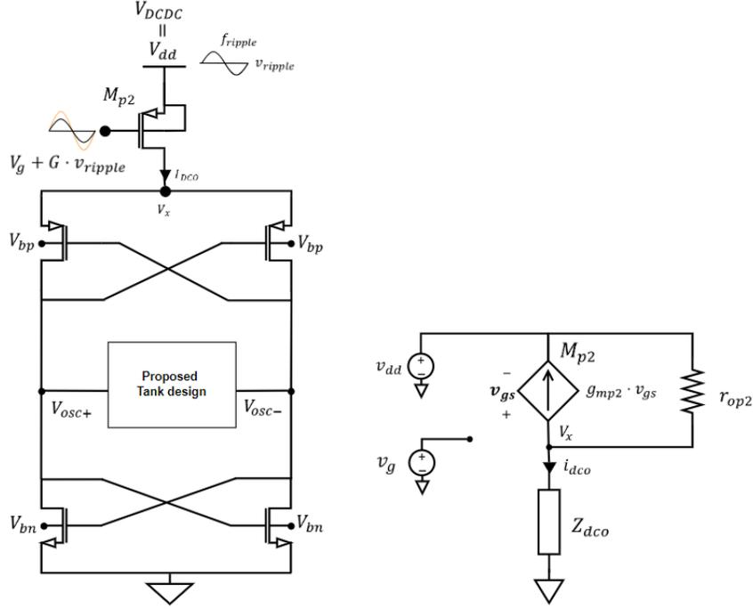
Figure 4.2: The supply ripple replicated on the gate with a gain  $G$  on the current source (left) and equivalent model of the current source (right).
