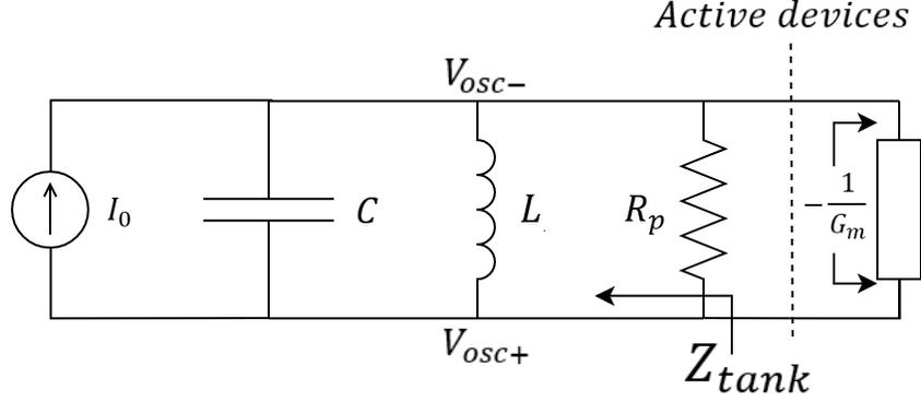
Figure 2.1: LC tank with  $R_p$  losses compensated by positive feedback by the active devices.
