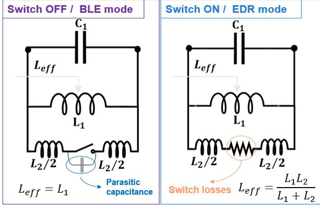
Figure 3.6: Illustration of the  $LC$  tank with an additional  $L_2$  in parallel, that can be turned OFF or ON.
