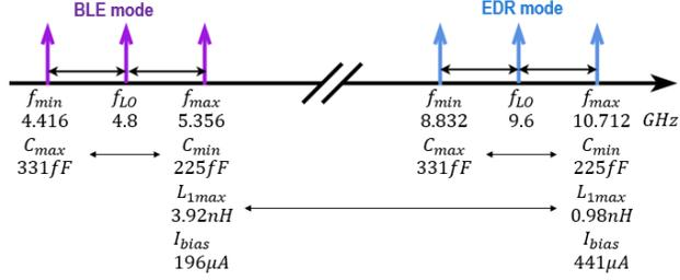
Figure 3.5: Illustration of the frequency band of BLE and EDR, with its required capacitance and expected  $I_{bias}$  with  $Q_{tank} = 12.12$  for tuning the inductance from  $L_1 = 0.98$  nH to  $L_1 = 3.92$  nH.
