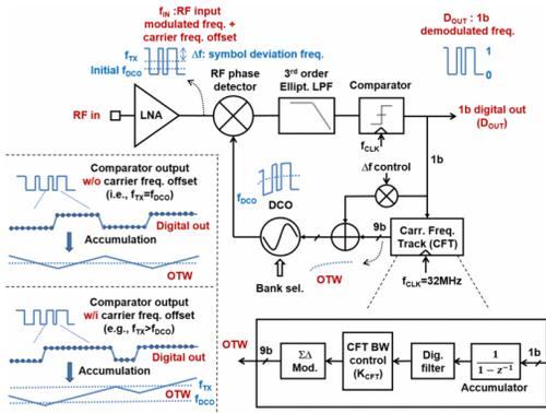
Figure 1.3: Zero-IF with phase tracking. Conducted from [18]
