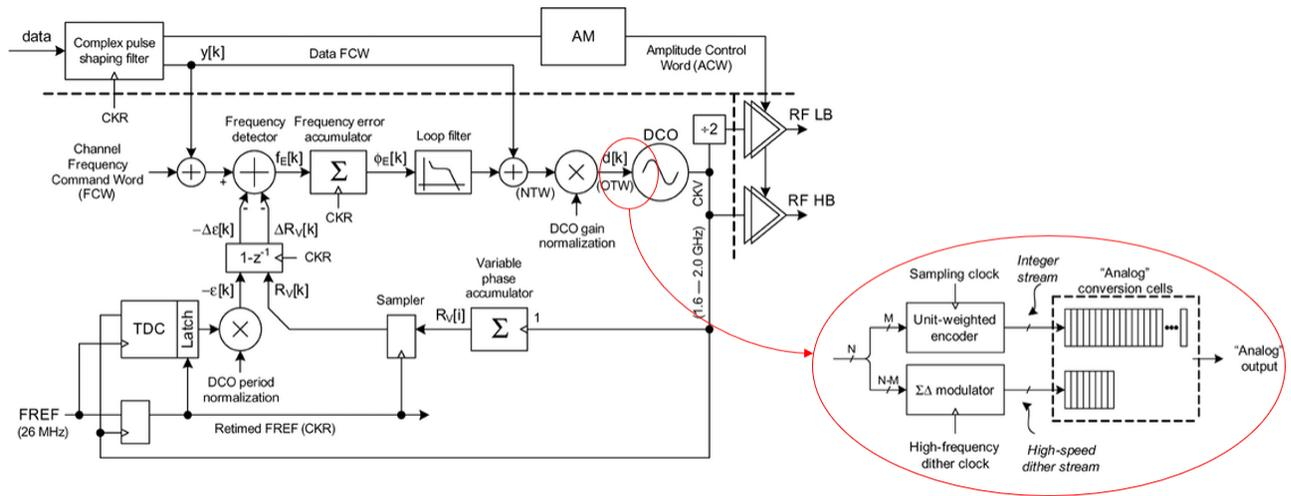
Figure 1.7: Polar transmitter based on ADPLL with described DAC for the DCO [38]
