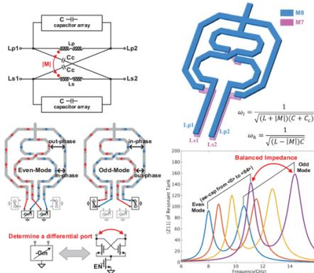
Figure 2.9: (left) Schematic of the resonator with change in current for even and odd mode. (right) Illustration of the inductor with its resulting impedance peaks [96].
