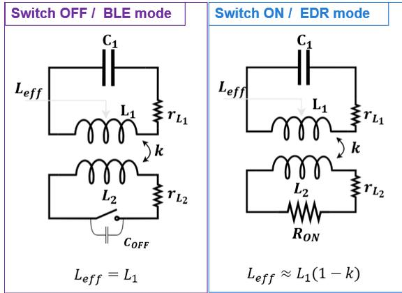
Figure 3.9: Illustration of the LC tank with an additional  $L_2$  magnetically coupled, that can be turned OFF or ON.
