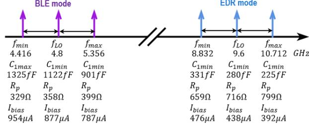
Figure 3.4: Illustration of the frequency band of BLE and EDR, with its required capacitance and expected  $R_p$  and  $I_{bias}$  with  $Q_{tank} = 12.12$  and  $L_1 = 0.98$  nH.
