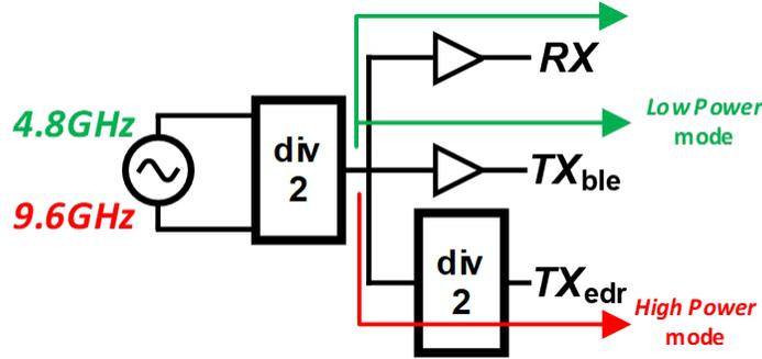
Figure 1.10: The implementations of a dual-mode design with an additional divider
