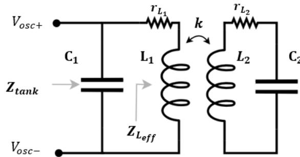
Figure 3.11: Illustration of a resonator with the output of the oscillator at the primary side.
