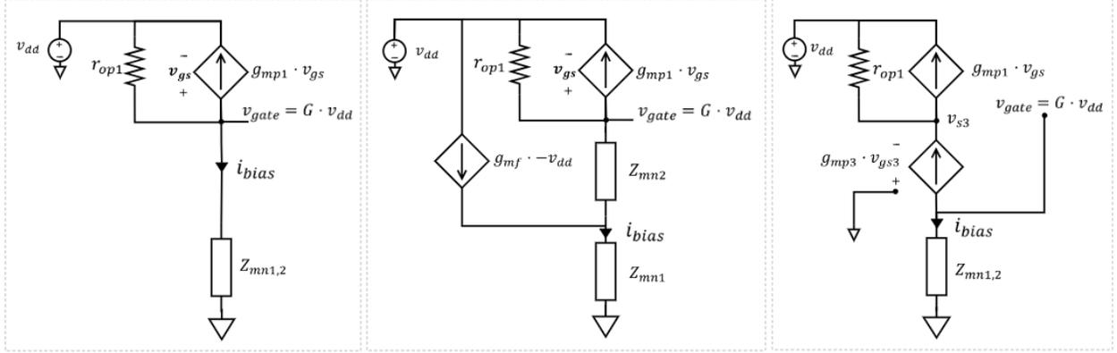
Figure 4.5: Equivalent circuits of the conventional current mirror (left), the circuit from [127] (middle), the proposed circuit with  $M_{p3}$  (right).
