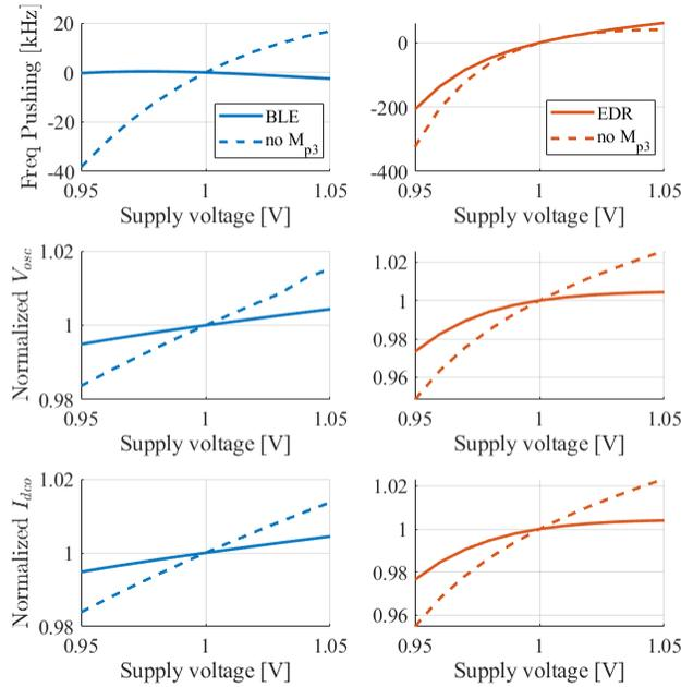
Figure 4.7: The change in frequency, oscillation amplitude and current over supply change.
