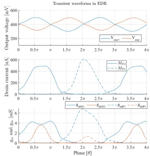
Figure 3.34: Transient PEX simulation EDR at 10.75 GHz with  $I_{dco} = 312 \mu A$
