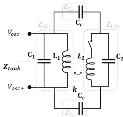
Figure 3.15: Proposed dual-mode resonator with electrically coupled capacitance, creating parallel inductors at high frequency.
