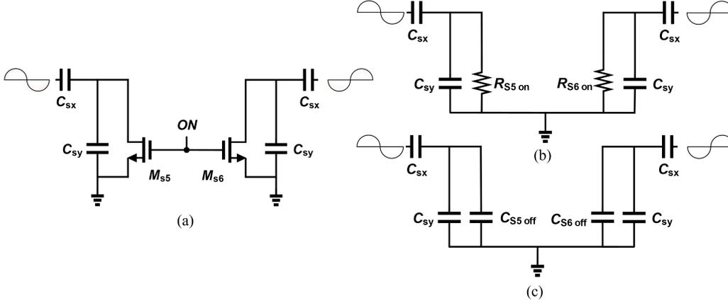
Figure 3.30: Schematic and lumped model of the fine-tuning bank(a), in ON(b) and OFF(c) mode
