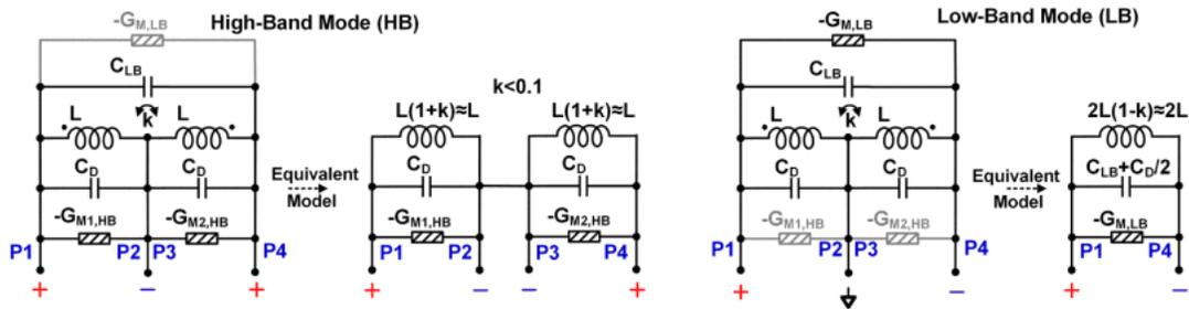
Figure 2.8: (Left) HB mode where two  $-G_m$  are activated. (Right) LB mode where one  $-G_m$  is activated [95].
