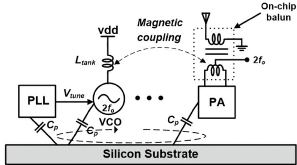
Figure 1.8: Illustration of oscillator pulling in transceivers [43].
