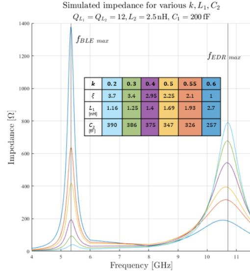
Figure 3.14: Simulated tank impedance for  $\omega_1^2/\omega_2^2 = 4$  and at the tuned at  $f_{max}$  for each mode, as a function of  $k, C_2$  and  $L_1$ .
