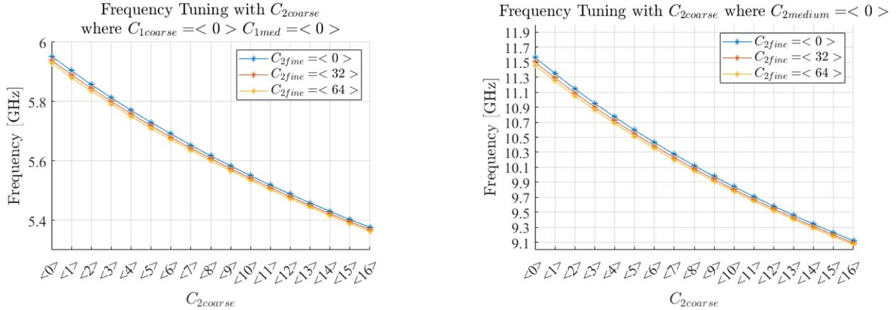
Figure 3.31: Oscillation frequency BLE and EDR over tuning  $C_{fine}$  over various large  $C_{2coarse}$  steps.
