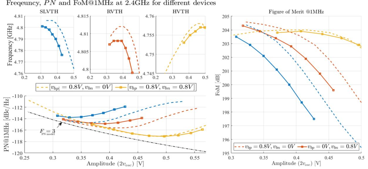
Figure 2.13: Frequency and phase noise results over amplitude on the left and on the right its resulting FoM. For the LTV PN model (equation (2.9)) an  $R_p = 1490\Omega$  and  $F = 3$  are chosen.
