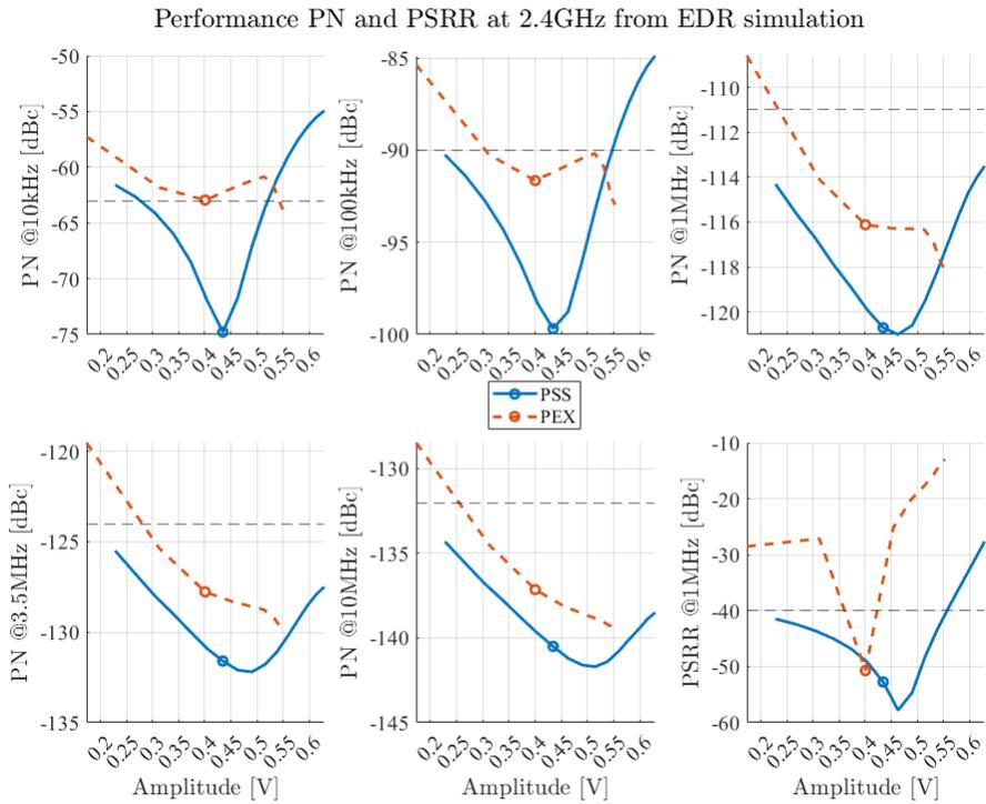
Figure 3.40: EDR PN referred to 2.4GHz band at various offsets. Dotted line describes the minimum PN spec
