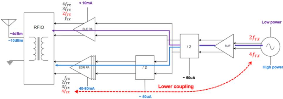
Figure 3.1: Proposed transmitter where the oscillator changes mode with the BLE and EDR mode. A lower coupling between EDR PA and DCO is achieved when operating  $f_{LO} = 4f_{TX}$ .
