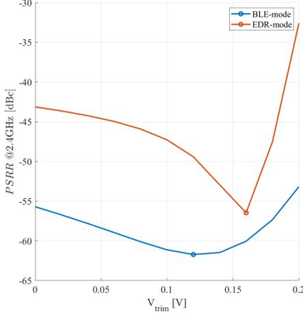
(a) PSRR as a function of gate voltage of  $M_{p3}$ .
