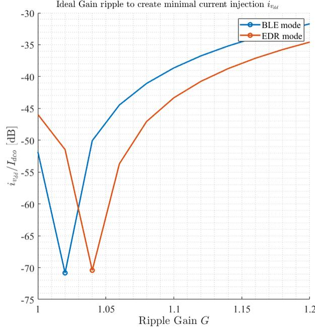
Figure 4.3: Ideal current injection by a 1MHz, 10mV<sub>pp</sub> supply ripple, with ideal ripple gain on  $V_{gate}$ .
