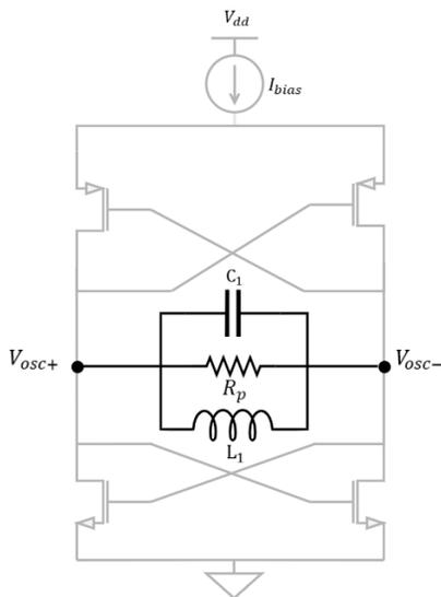
Figure 3.2: The LC tank in CMOS cross-coupled configuration.
