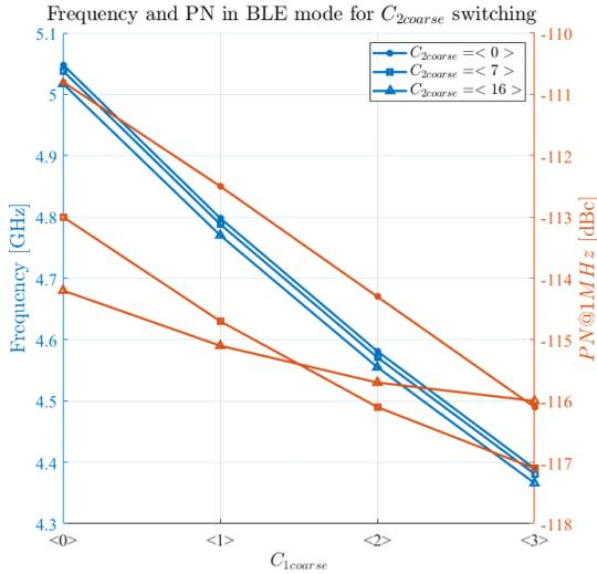
Figure 3.37: BLE frequency and PN as function of the  $C_{1coarse}$  and  $C_{2coarse}$ .
