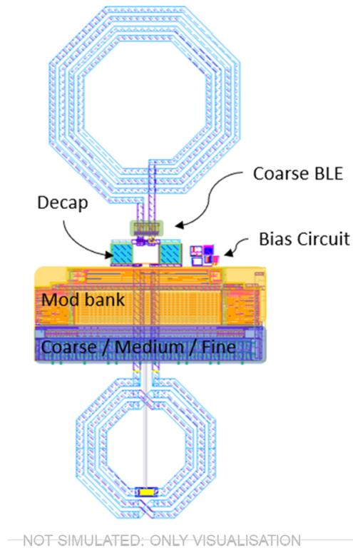
Figure 5.1: Visualization of a possible layout, where all the components fit in between the inductors.
