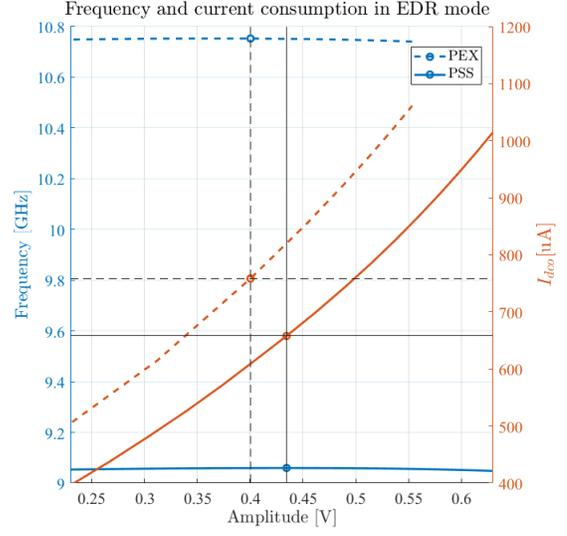
Figure 3.36: EDR frequency and current consumption as function of the amplitude. With active devices biased at  $|V_{bp}| = 0$  V and  $V_{bn} = 0$  V
