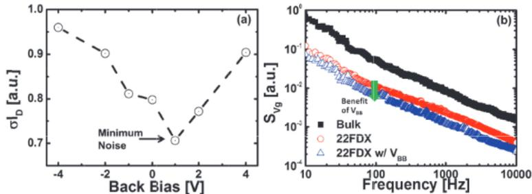
Figure 1.1: (a) Drain current standard deviation  $\sigma I_d$ . (b) Gate bias power spectrum  $S_{V_g}$  of 22FDX and 28nm bulk devices. Conducted from [9]
