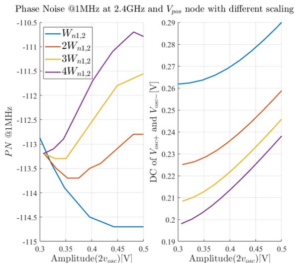
Figure 2.14: PN performance over various for different multiplication factors.  $W_{p1,2}/W_{n1,2} = 2.6$
