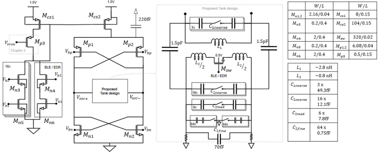
Figure 3.32: Proposed design with current source, CMOS cross coupled devices and the tank.
