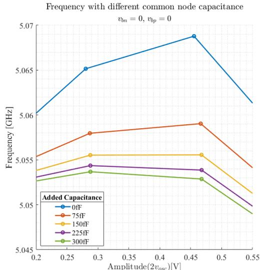
Figure 2.15: Oscillation frequency for various added common node capacitance  $C_{tail}$
