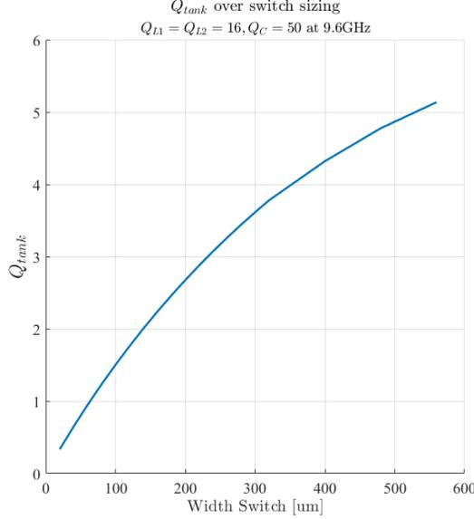
Figure 3.8:  $Q_{tank}$  calculated with the added  $R_{ON}$  from the HVTH switch. With  $L_1 = 3.92$  nH and  $L_2 = 0.98$  nH.
