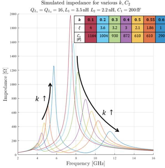
Figure 3.13: Simulated tank impedance for  $\omega_1^2/\omega_2^2 = 4$ , as a function of  $k$  and  $C_2$
