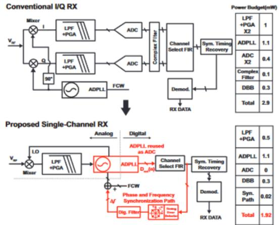
Figure 1.4: Low-IF with hybrid loop. Conducted from [24]
