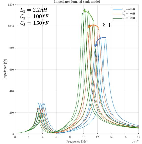
Figure 3.24: Tank impedance with lumped model for various  $L_2$  as a function of  $k$ .  $Q_{C1,2} = \infty$
