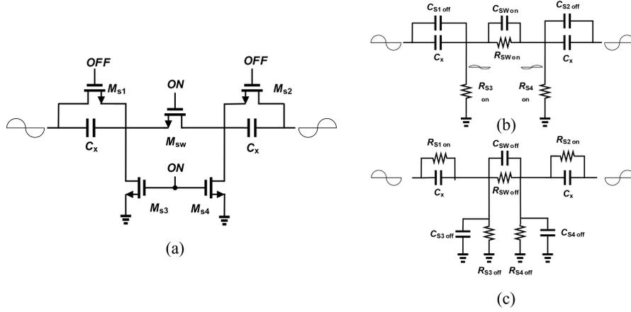
Figure 3.27: Schematic and lumped model of the coarse and medium tuning bank(a), in ON(b) and OFF(c) mode.
