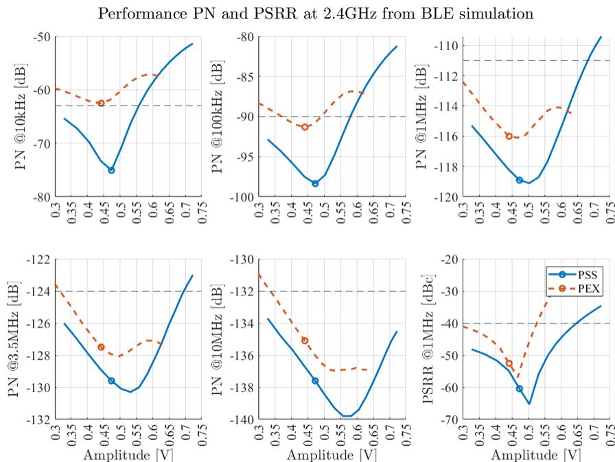
Figure 3.39: BLE PN referred to 2.4GHz band at various offsets. Dotted line describes the minimum PN spec
