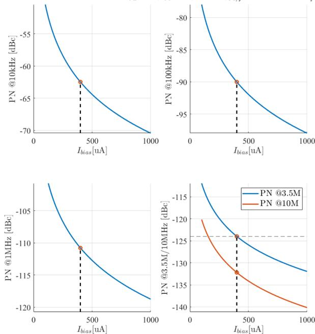
Figure 3.3: Leeson's PN model as a function of  $I_{bias}$  based on equation (2.9)
