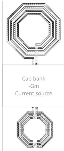
Figure 3.25: Proposed layout with a spiral  $L_1 = 2.80\text{nH}$  and symmetrical inductor  $L_2 = 0.8\text{nH}$ , with  $(143.7\mu\text{m} \times 162.7\mu\text{m})$  and  $(104.8\mu\text{m} \times 111.4\mu\text{m})$  respectively.
