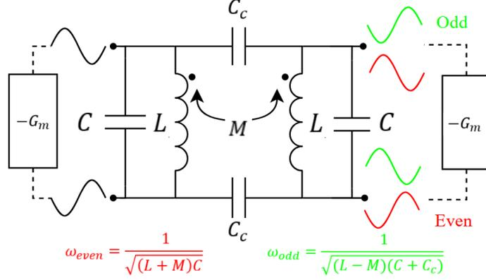
Figure 2.6: Coupling of two identical tanks via  $C_c$  and  $M$
