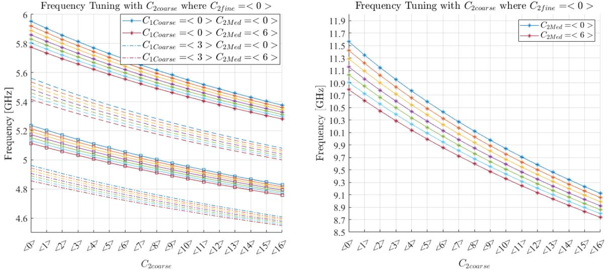
Figure 3.29: Oscillation frequency BLE and EDR over tuning each  $C_{1coarse}$  and  $C_{1med}$  code over various large  $C_{2coarse}$  steps.
