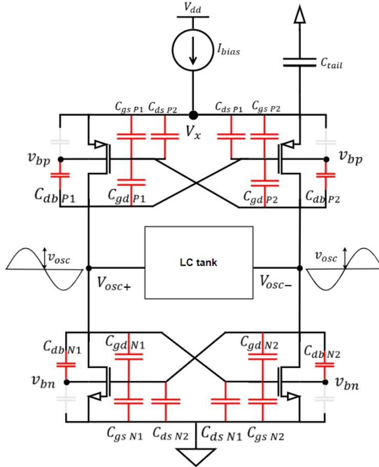
Figure 2.10: CMOS with all the considered parasitic capacitance showed in red.
