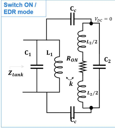
Figure 3.18: Illustration of the proposed tank when the switch is turned ON
