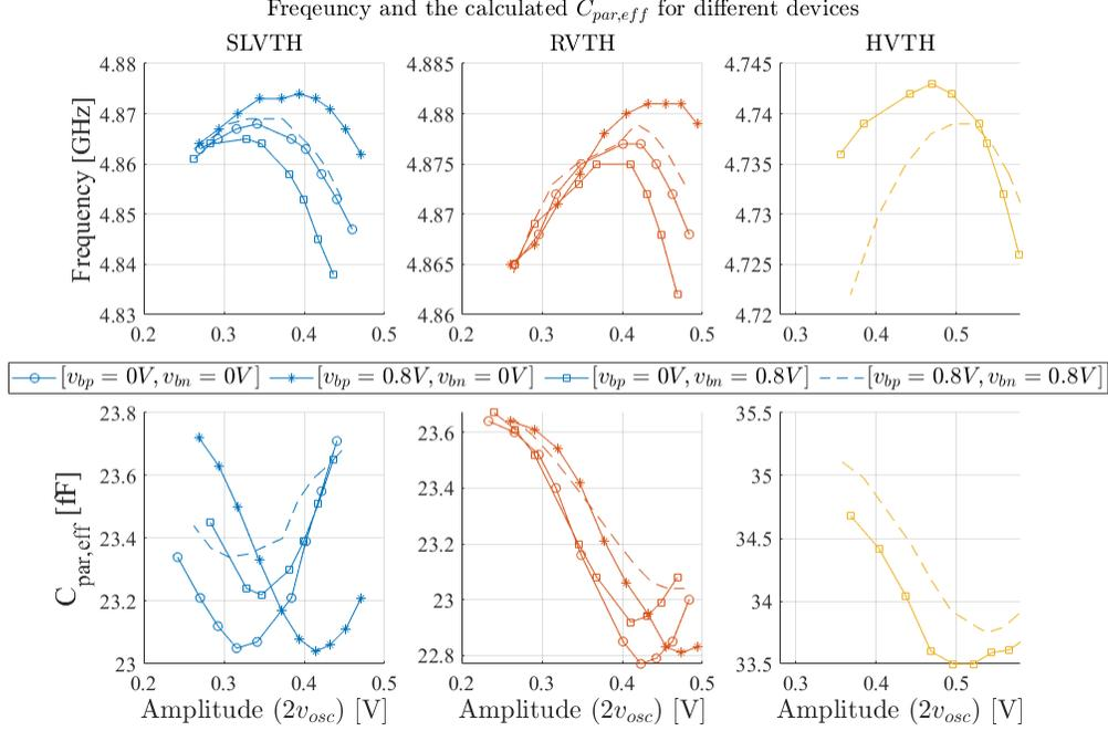
Figure 2.12: Different type of devices with its oscillating frequency at the top and its effective capacitance on the bottom. Different bulk biasing  $v_{bn}, v_{bp}$  are simulated over the various amplitudes.
