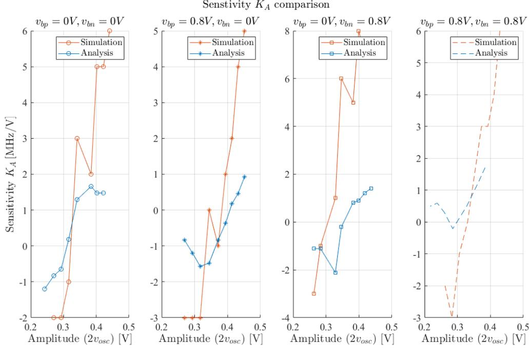
Figure 2.11: Sensitivity  $K_a$  as function amplitude for different  $v_{bp}$  for PMOS and  $v_{bn}$  NMOS.
