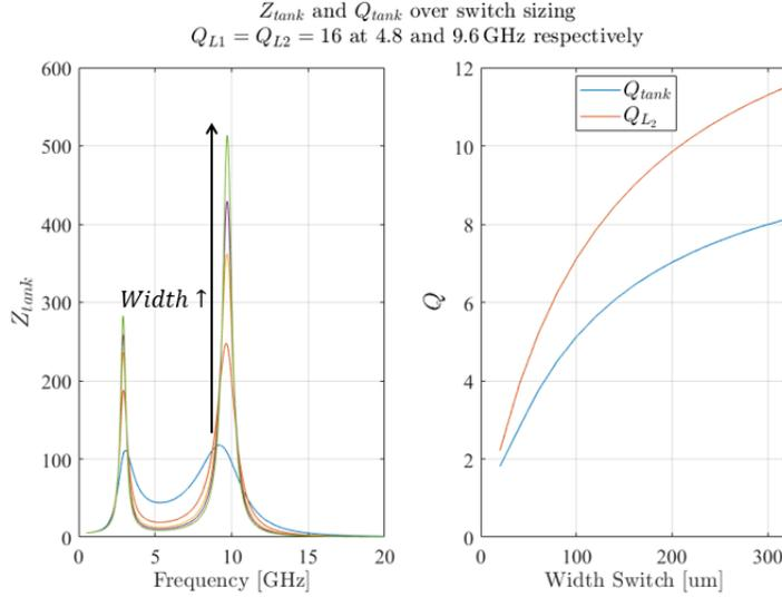
Figure 3.20: The effect of scaling the switch on the  $Z_{tank}$ ,  $Q_{tank}$  and  $Q_{L2}$ .  $C_c = 1.5$  pF,  $C_1 = 100$  fF,  $C_2 = 330$  fF,  $L_1 = 2.8$  nH,  $L_2 = 0.8$  nH.
