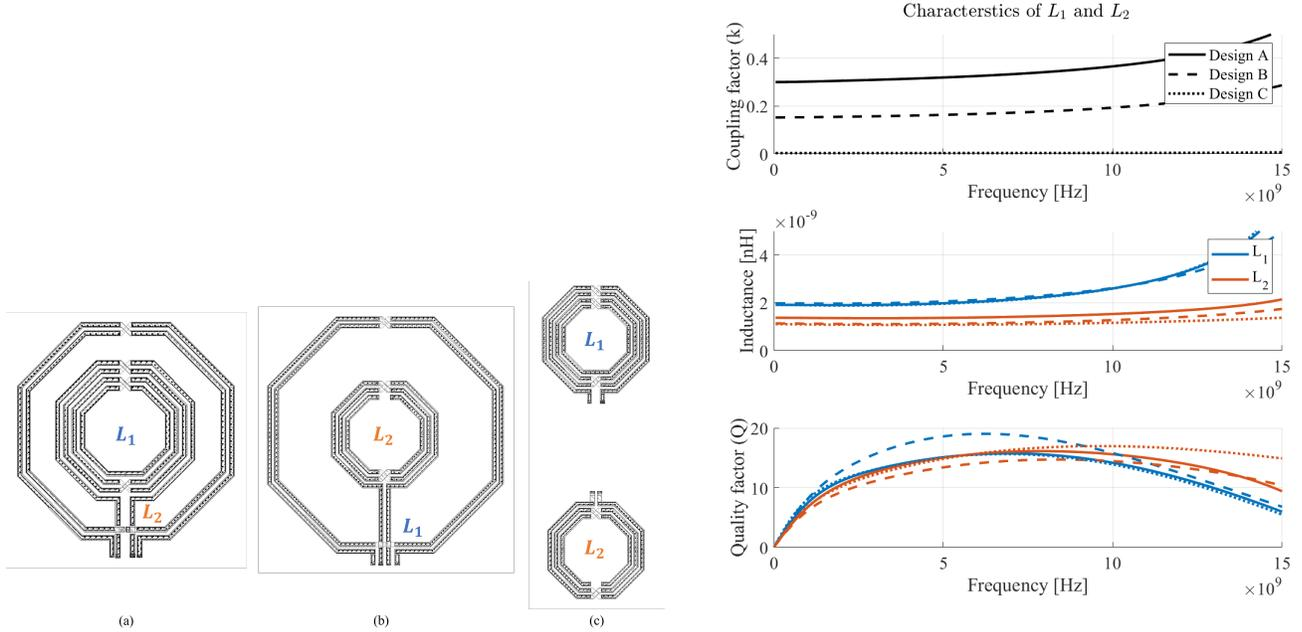
Figure 3.22: Three inductors designs(A,B,C) with each their  $k, L$  and  $Q_L$  over frequency. Layout figures are not equally scaled.
