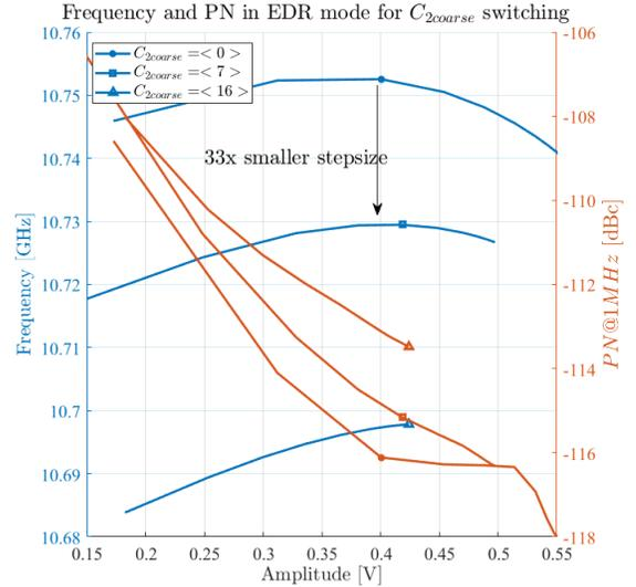
Figure 3.38: EDR frequency and PN as function of the amplitude and  $C_{2coarse}$ .
