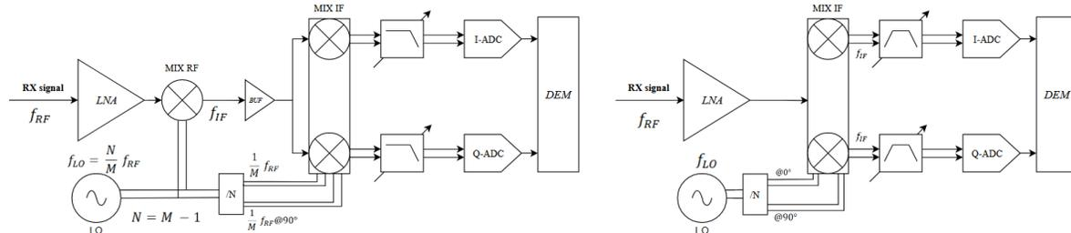
Figure 1.2: Receiver with the sliding- and low- IF architectures shown in left and right respectively.
