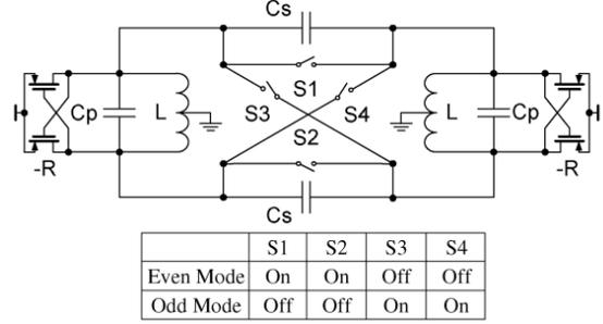
(b) Dual band oscillator with four switches [90]
