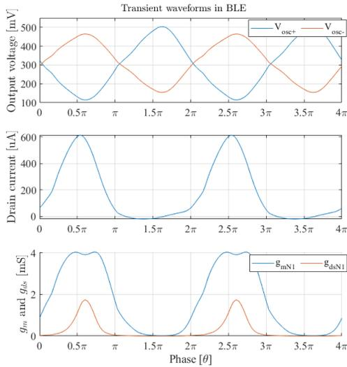
Figure 3.33: Transient PEX simulation BLE at 5.02 GHz with  $I_{dco} = 352 \mu A$
