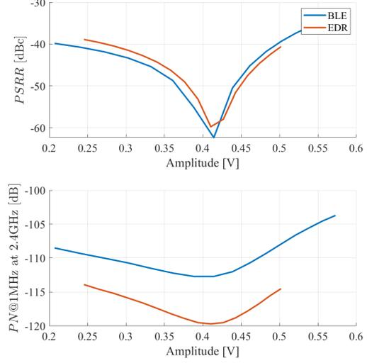
(b) PSRR and PN as a function of different oscillation amplitudes.  $M_{p3}$  is biased at optimal  $V_{trim}$ .  $V_{bp} = 0V$  and  $V_{bn} = 0V$
