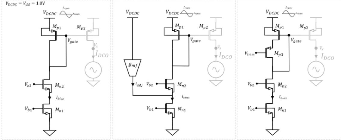
Figure 4.4: Replication circuit containing current mirror ( $M_{p1}, M_{p2}$ ) with cascoded current source ( $M_{n1}, M_{n2}$ ): Conventional (left), Circuit from [127] (middle), proposed circuit with  $M_{p3}$  (right).
