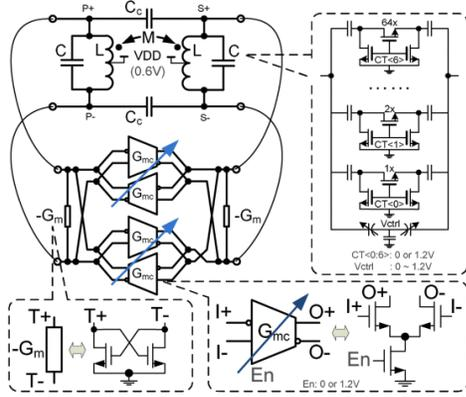
(a) Dual band oscillator with four  $G_m$  cells [89]
