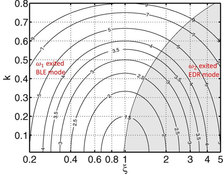
Figure 3.12: Contour plot of  $(\omega_2/\omega_1)^2$  as a function of  $\xi$  and  $k$ . The shaded area represents when  $R_{p2}$  will be exited and otherwise the  $R_{p1}$ . Conducted from [92]
