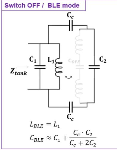
Figure 3.16: Illustration of the proposed tank when the switch is turned OFF.
