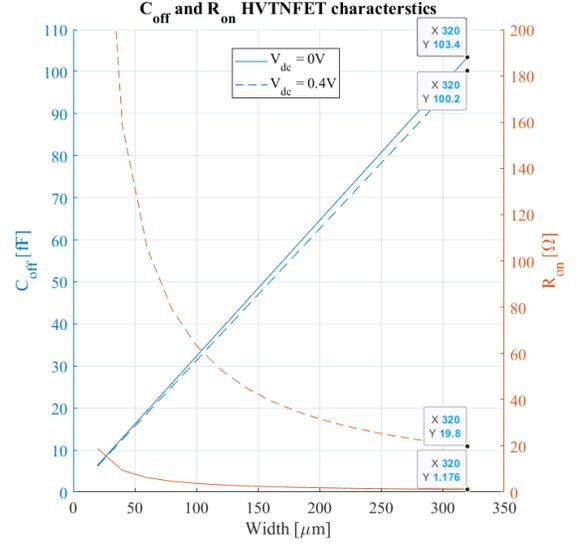
Figure 3.7:  $R_{ON}$  and  $C_{off}$  as function of scaling the HVTH at a DC of 0V and 0.4V
