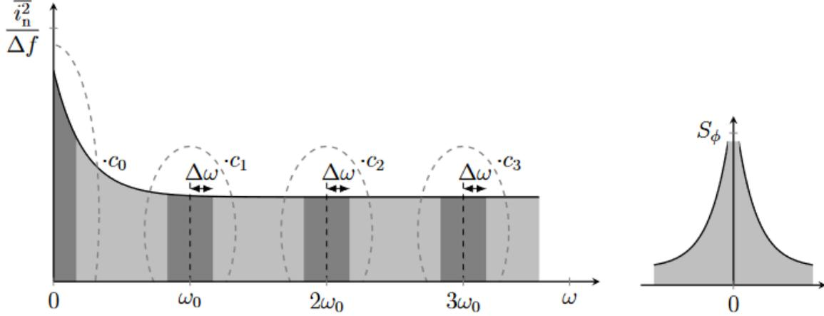
Figure 2.2: Noise folding principle from [57]
