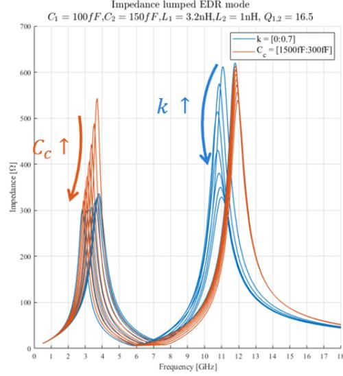
Figure 3.19:  $Z_{tank}$  at various  $k$  and  $C_c$  when the switch is ON and is sized at  $W = 320 \mu\text{m}$
