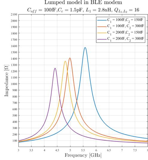
Figure 3.17:  $Z_{tank}$  at different  $C_1$  and  $C_2$  ( $Q_C = \infty$ ) when the switch is OFF and sized at  $320 \mu\text{m}$
