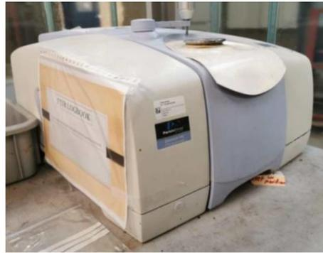
Figure 3.9: The Spectrum 100 FT-IR spectrometer.
