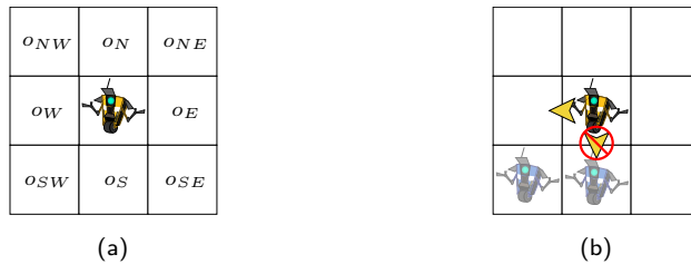
Figure 2.7 Two-robot example in the decentralised setting: (a) the observations each robot can make regarding the position of the other robot and (b) conditioning its action decision based on the previous observation prevents the yellow robot from performing a South move when blue is in either of the shown relative positions.
