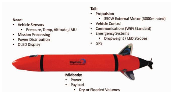
Figure 52: Layout of a typical small AUV (Manley and Smith, 2017)
