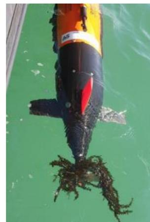
Figure 53: Seaweed tissue stuck in propulsion mechanism of AUV (TNO, 2022)
