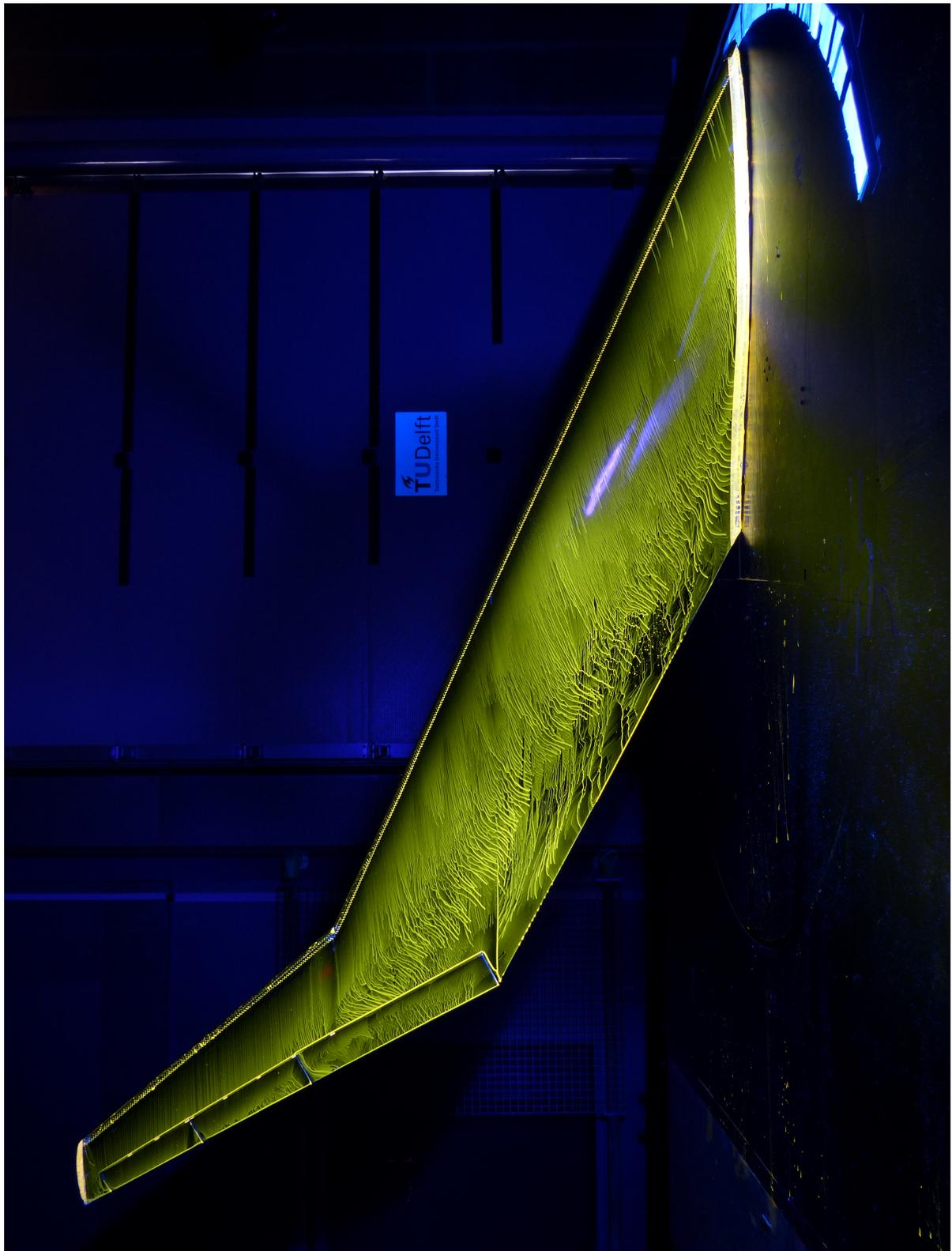
Figure A.3: Oil flow visualisation at 9 degrees angle of attack
