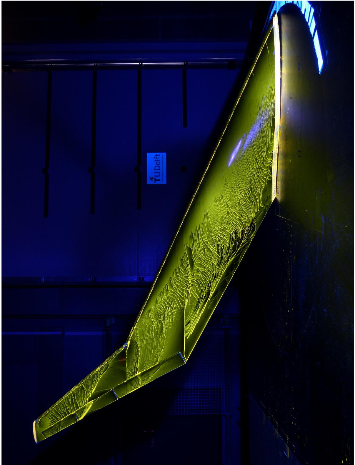
Figure A.5: Oil flow visualisation at 13 degrees angle of attack
