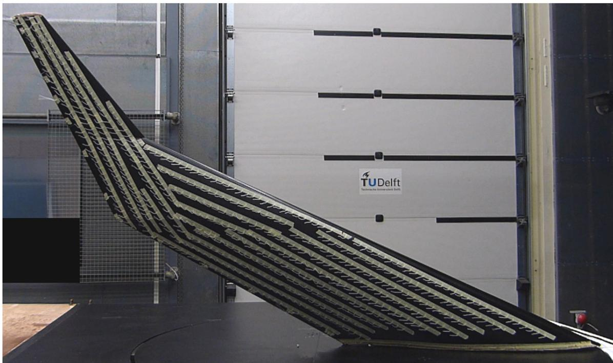
Figure 4.33: Impression of the tuft configuration at 11 degrees angle of attack
