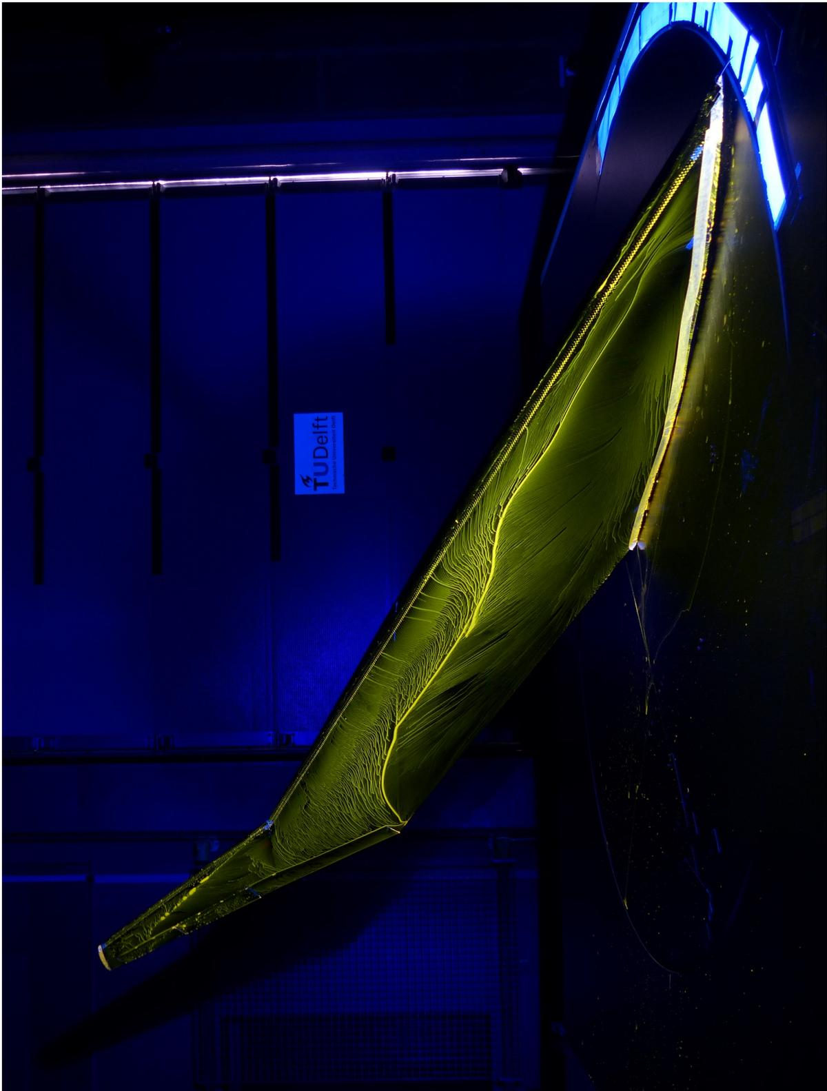
Figure A.20: Oil flow visualisation at 50 degrees angle of attack
