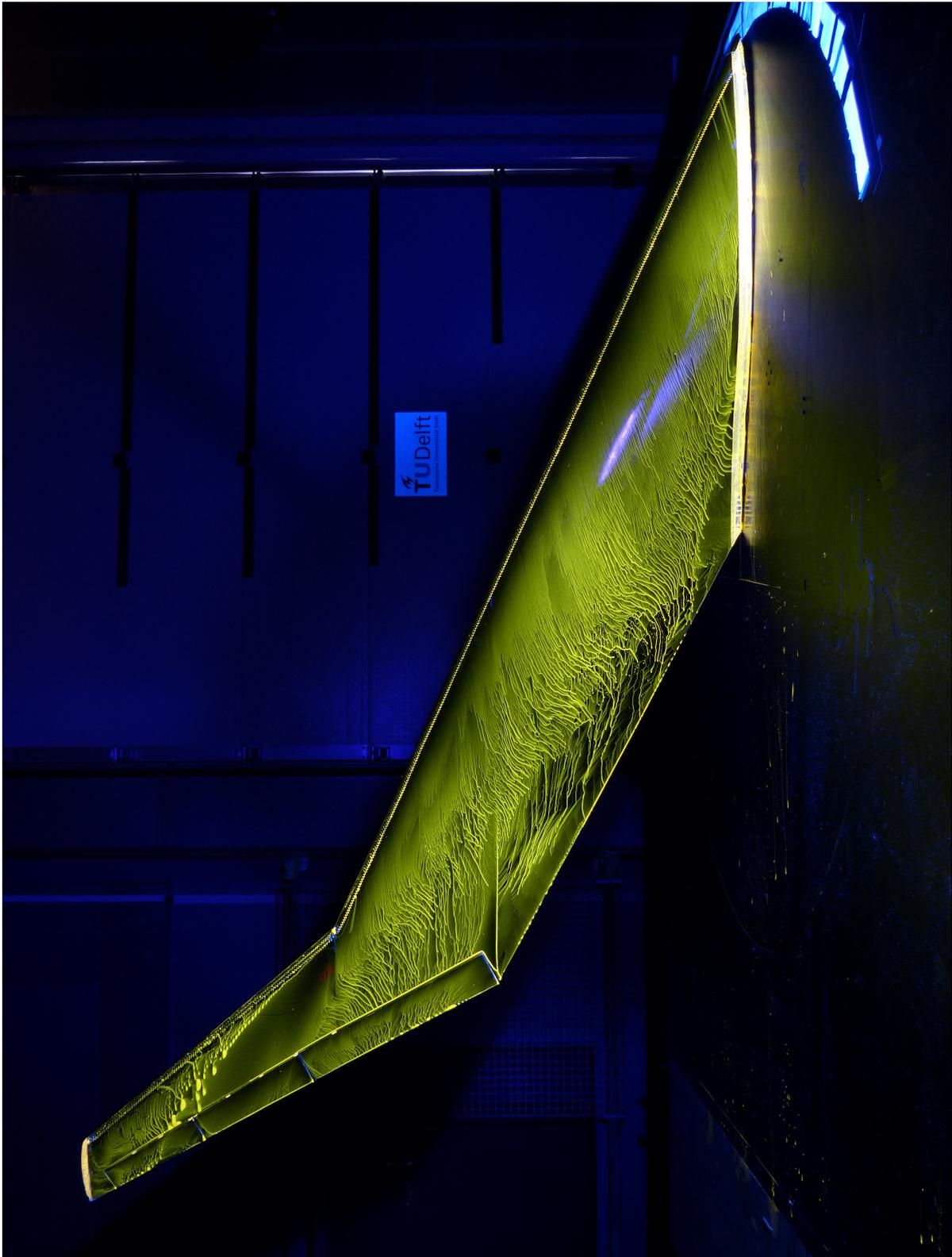
Figure A.4: Oil flow visualisation at 11 degrees angle of attack
