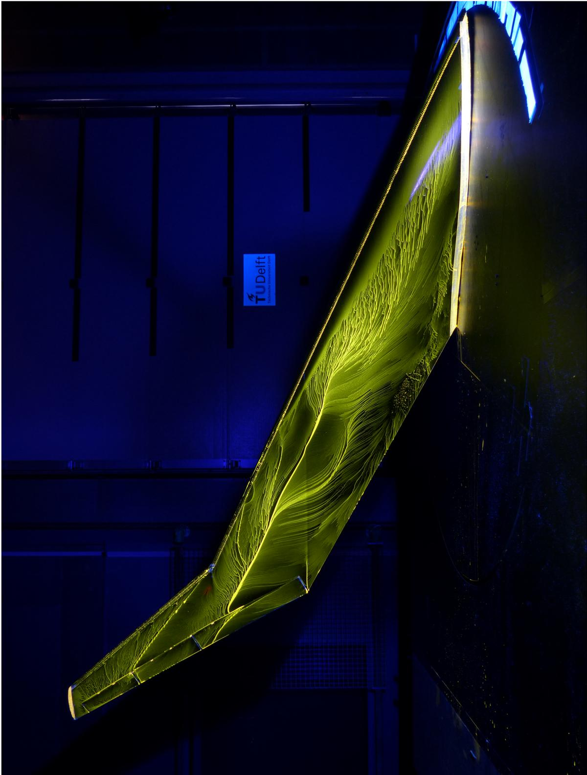
Figure A.10: Oil flow visualisation at 21 degrees angle of attack
