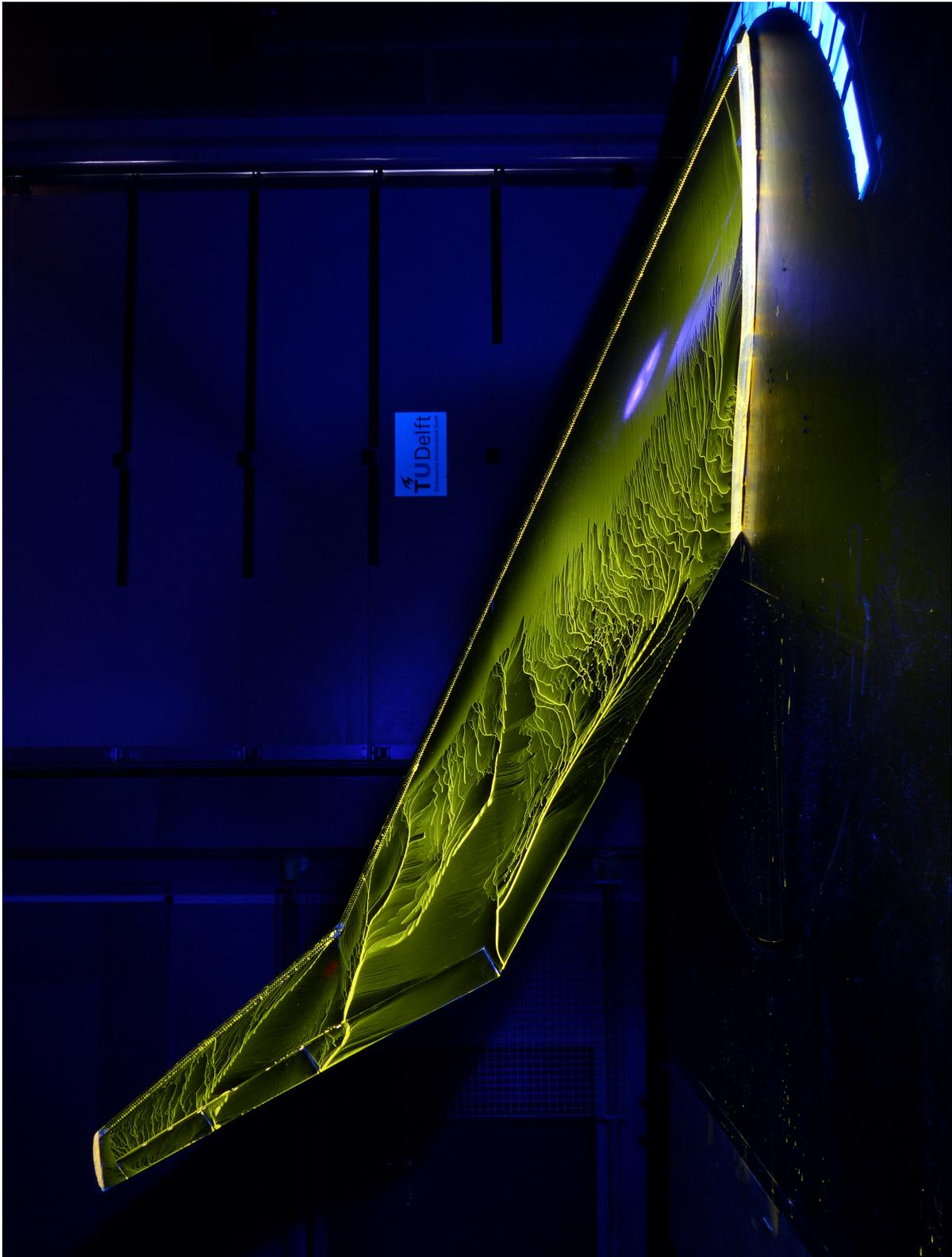
Figure A.6: Oil flow visualisation at 15 degrees angle of attack
