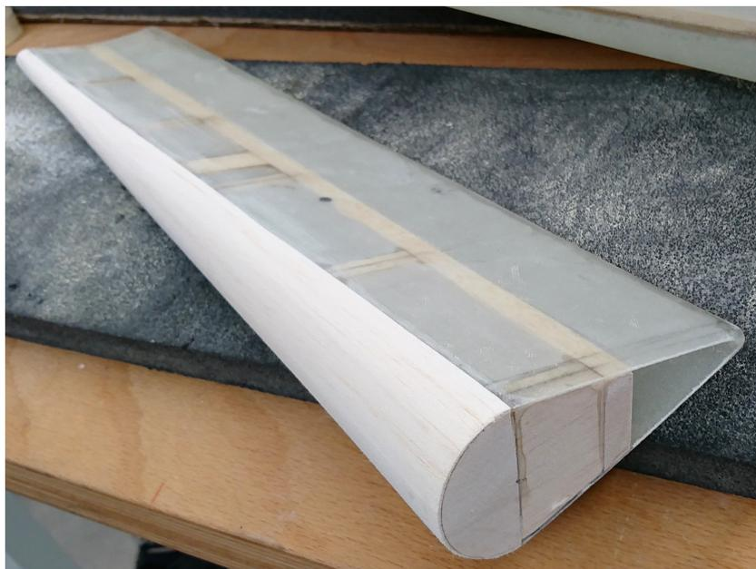
Figure 2.7: Control surface with a balsa wood leading edge
