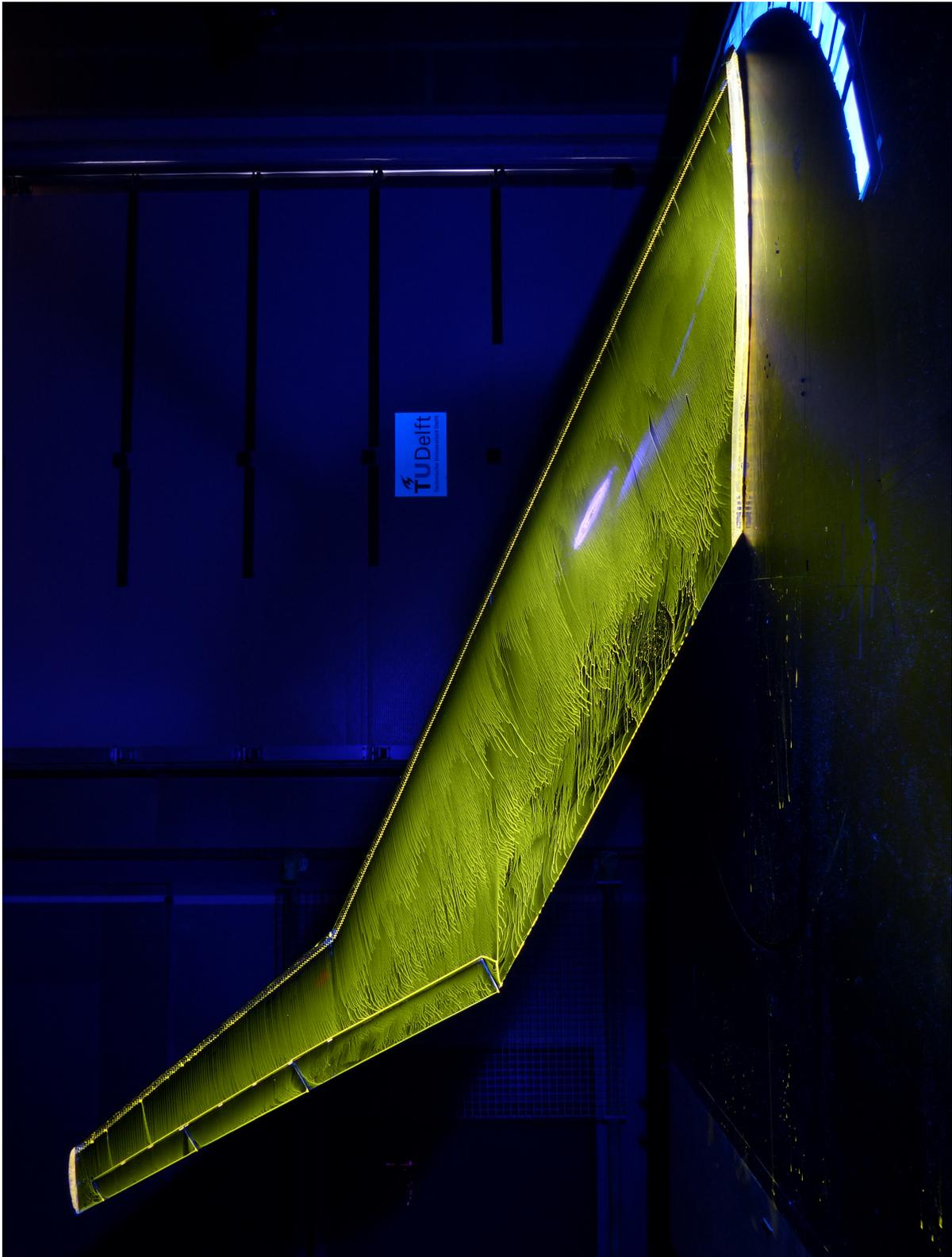
Figure A.2: Oil flow visualisation at 7 degrees angle of attack
