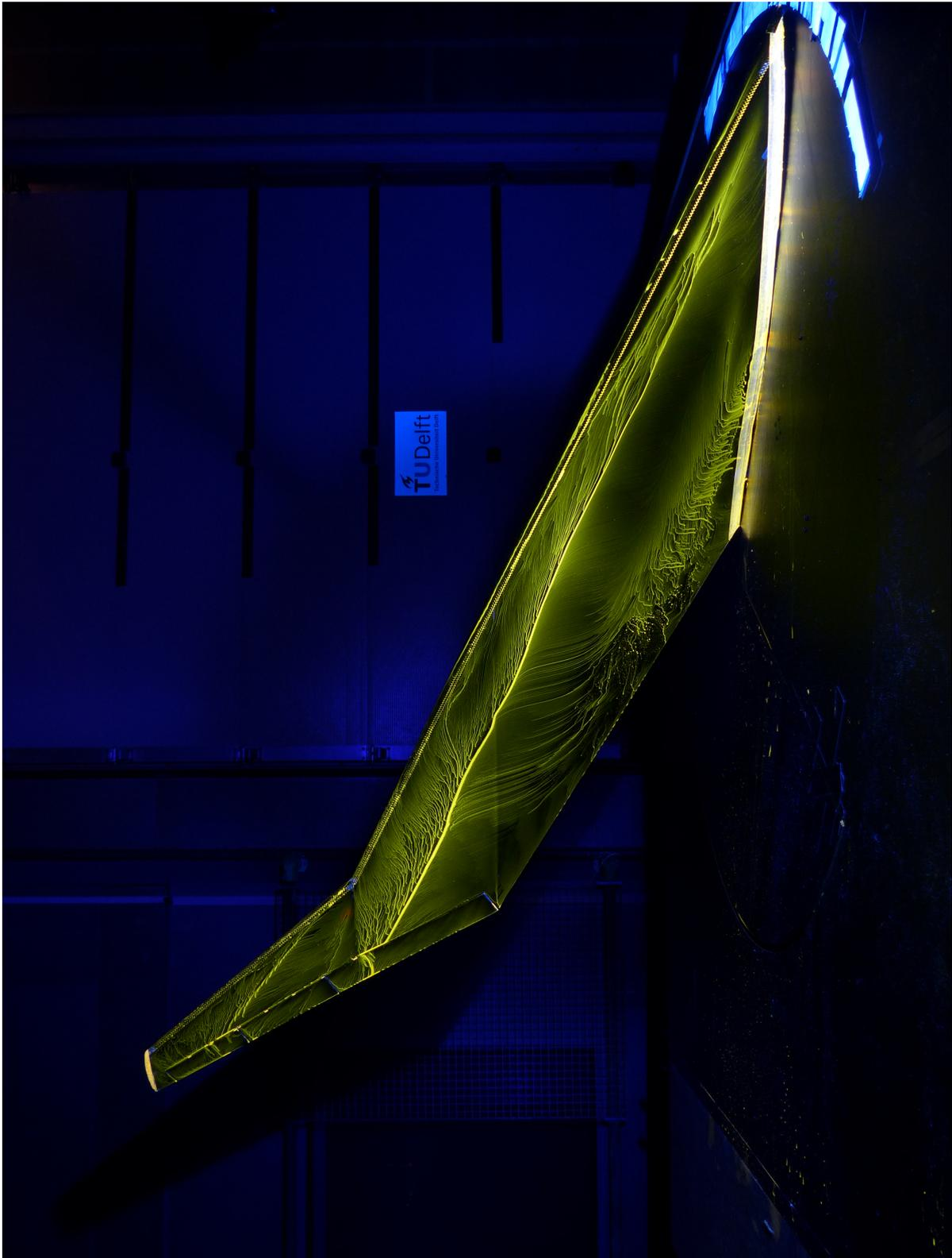
Figure A.18: Oil flow visualisation at 35 degrees angle of attack
