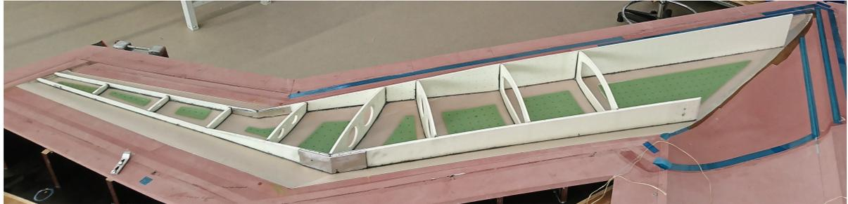
Figure 2.4: Spars and ribs fitted in the lower wing skin
