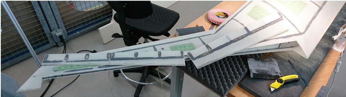
Figure 2.6: Cut out of the control surfaces
