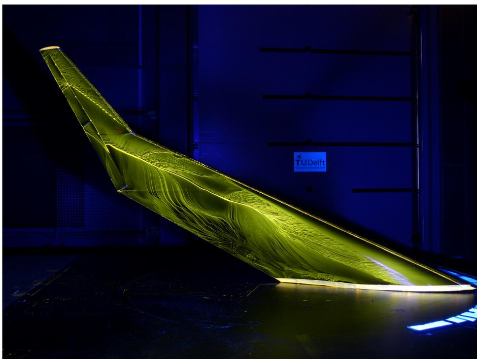
Figure 4.11: Oil visualisation for 22 degrees angle of attack
