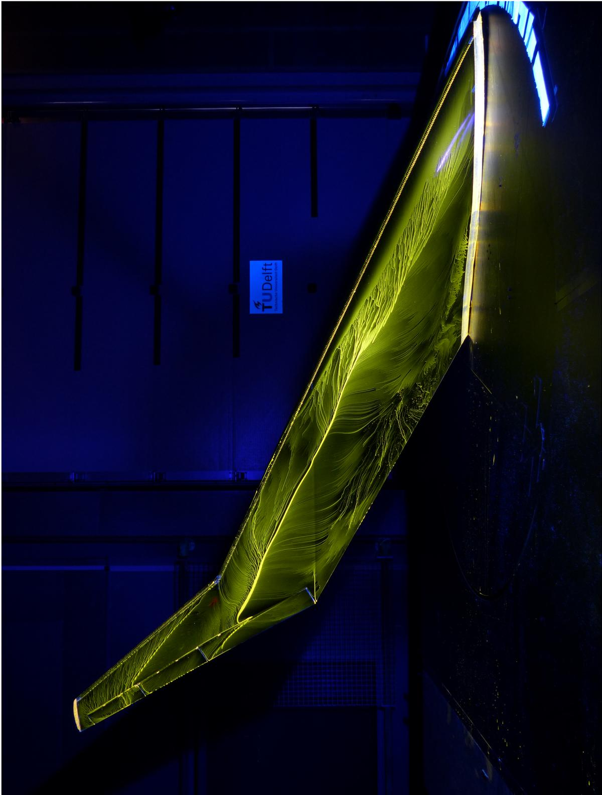
Figure A.12: Oil flow visualisation at 23 degrees angle of attack
