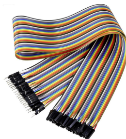
Figure 4.1: 40-pin male-to-female jumper cable used to connect the PIM183 to the Raspberry Pi.
