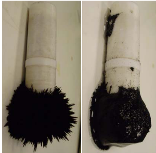
Figure 4.6 Adsorbent in external magnetic field: (left) dry adsorbent; (right) removed from bioreactor
