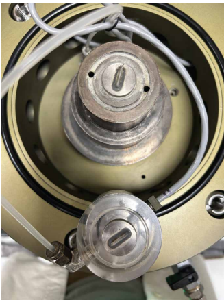
Figure 3.3: Photos and working principle of bender elements (after GDS Bender Elements Hardware Hand-book)
