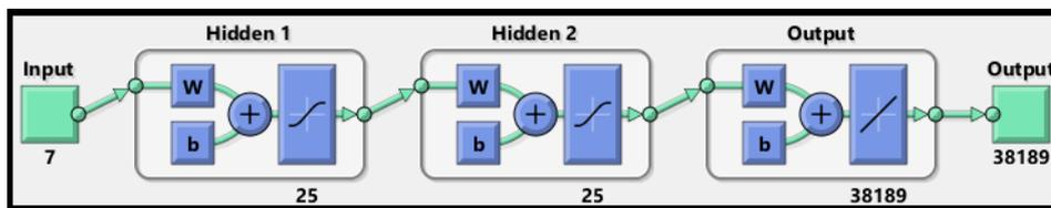
Figure 5.3: 2 layer 25x25 hidden nodes feed forward neural network
