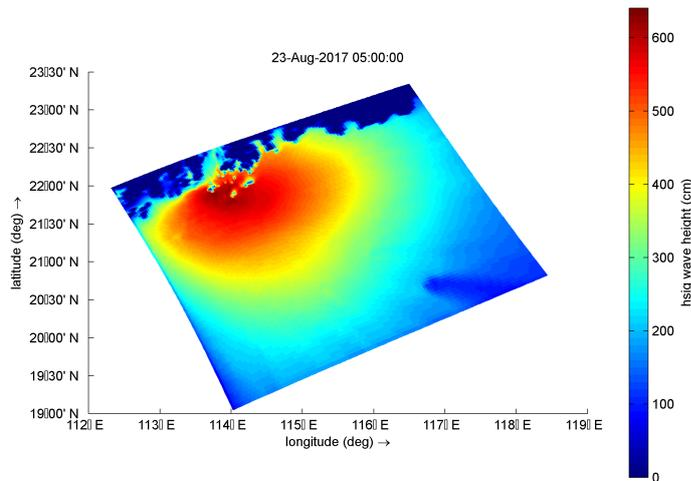
Figure 3.10: Significant wave height at peak storm tide, Course computational grid - Hato (2017)
