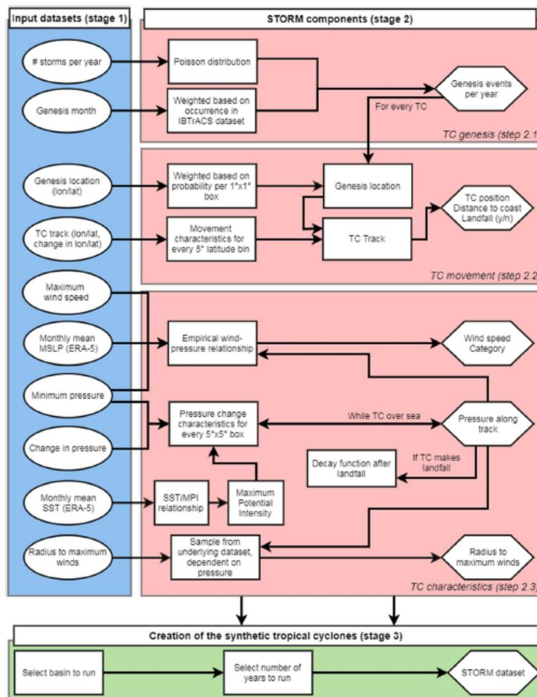
Figure 2.13: Flow chart generation synthetic TC database. Adapted from Bloemendaal et al. (2020)
