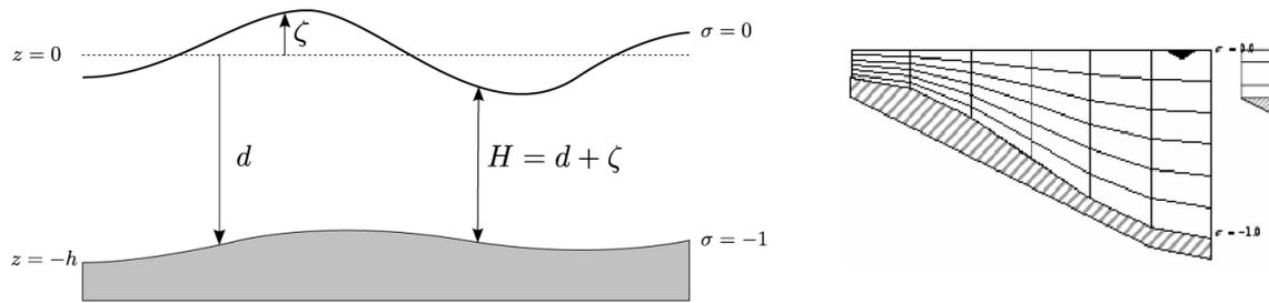
Figure A.3: (a) Definition of water level, depth and total depth (b)  $\sigma$  grid. Adapted from Deltares (2018)
