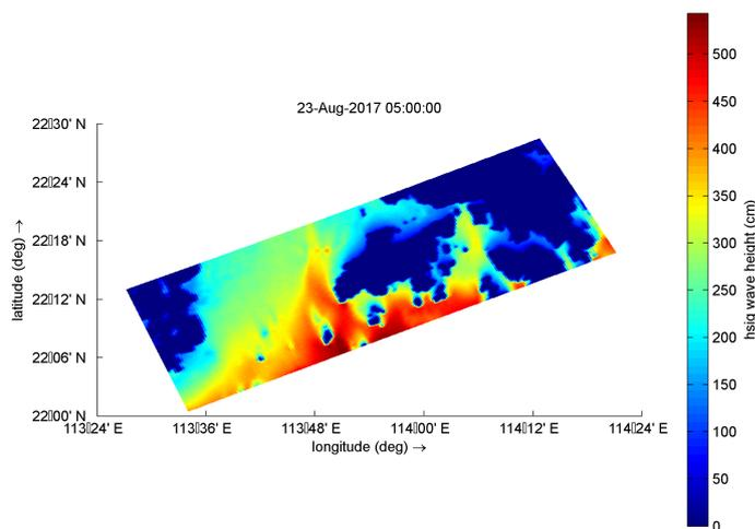
Figure 3.11: Significant wave height at peak storm tide, Fine computational grid - Hato (2017)
