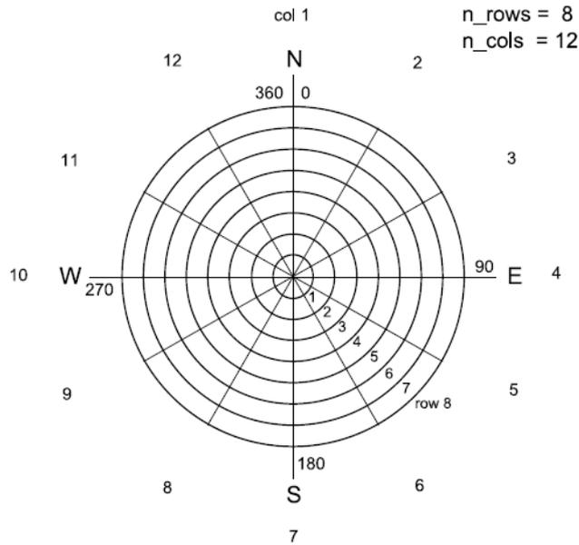
Figure 2.9: Spiderweb grid. adapted from DELFT3D flow manual.
