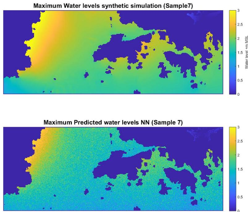
Figure 5.6: Comparison between maximum water levels of Delft3D and NN output. Training sample 7
