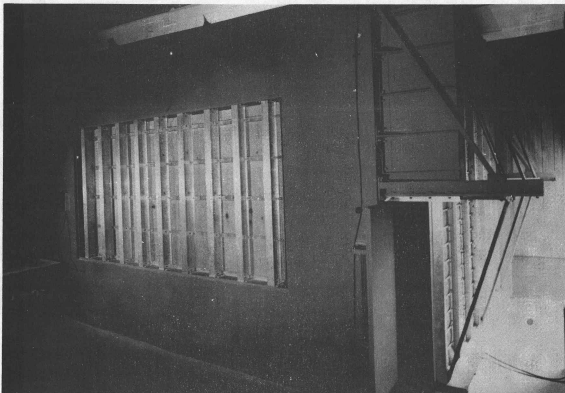
FIG. 11. VIEW OF THE SMALL END OF THE HORN SHOWING ALSO THE LARGE TANK OF THE AIR RESERVOIR SYSTEM, FLAP VALVE AND ELECTRIC-MOTOR DRIVE SYSTEM, CONTROL CONSOLE, AND ANCILLIARY ELECTRONICS.
