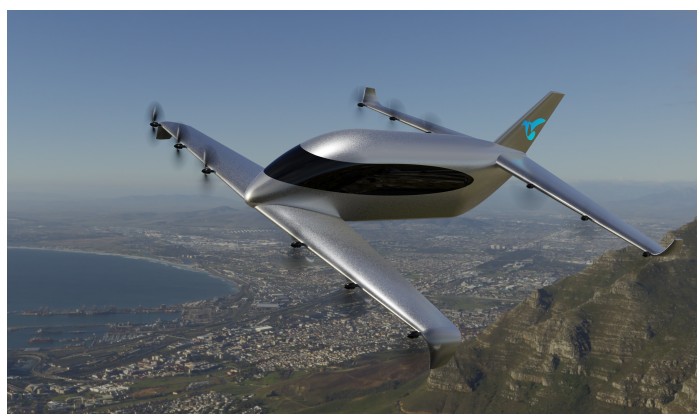
Figure 1. Rendering of the final design of the analysed configuration of the Wigeon.
