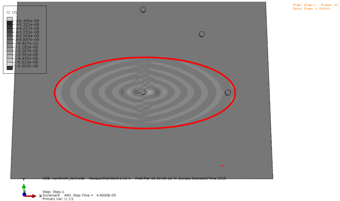
Figure 5-16: Sandwich panel S_0 mode wave front
