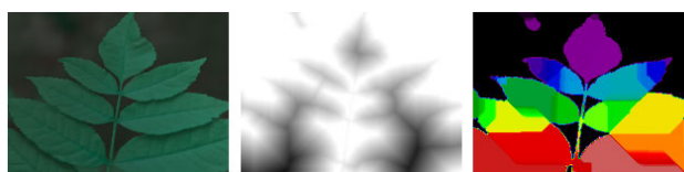
FIGURE 6. Example of the watershed algorithm applied to an image from the dataset (left). The outcome of the distance transform (middle) and the resulting image segmentation (right) can be seen.
